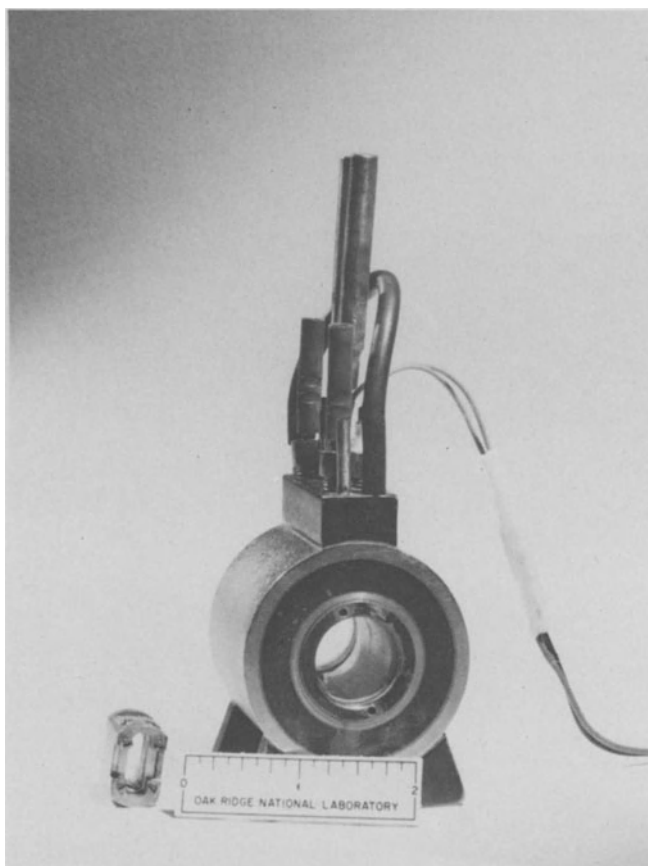
Fig. 13. Infrared furnace and \text{LaF}_3 -windowed cell.
