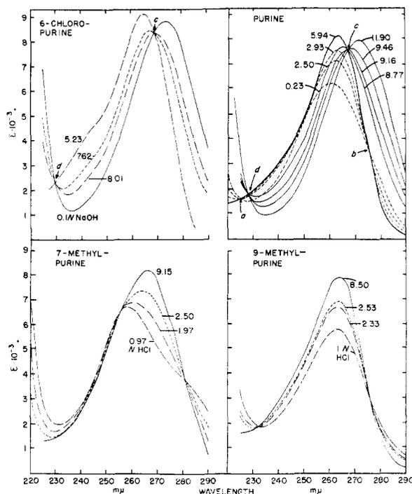
Fig. 1.—Ultraviolet absorption spectra of some purines in aqueous solutions at  $pH$  values indicated on the curves.
