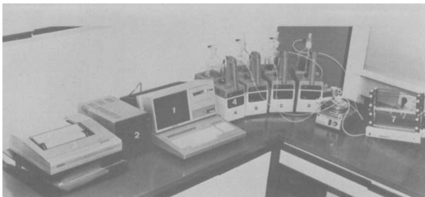
Fig. 17. The complete device for mixing an Immobiline gel gradient. (1)–(3) Computer, floppy disk station and matrix printer; (4) the four burettes, A to D; (5) the mixing chamber on a (6) magnetic stirrer; (7) a polymerization stand with two separation cells to be filled from the bottom. (From Altland and Altland, 1984. Reproduced with permission of the publisher.)
