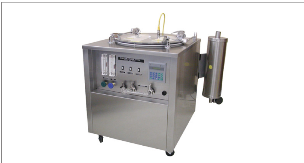
Figure 10A.5.1 Glas-Col aerosol device. This instrument is based upon earlier models originally developed by Middlebrook. The central gasket contains a large steel cage in which up to 80 to 100 mice can be exposed to aerosol at any one time. The device attached on the right is a heat sterilizer to incinerate any bacteria escaping the internal HEPA-filter systems.
