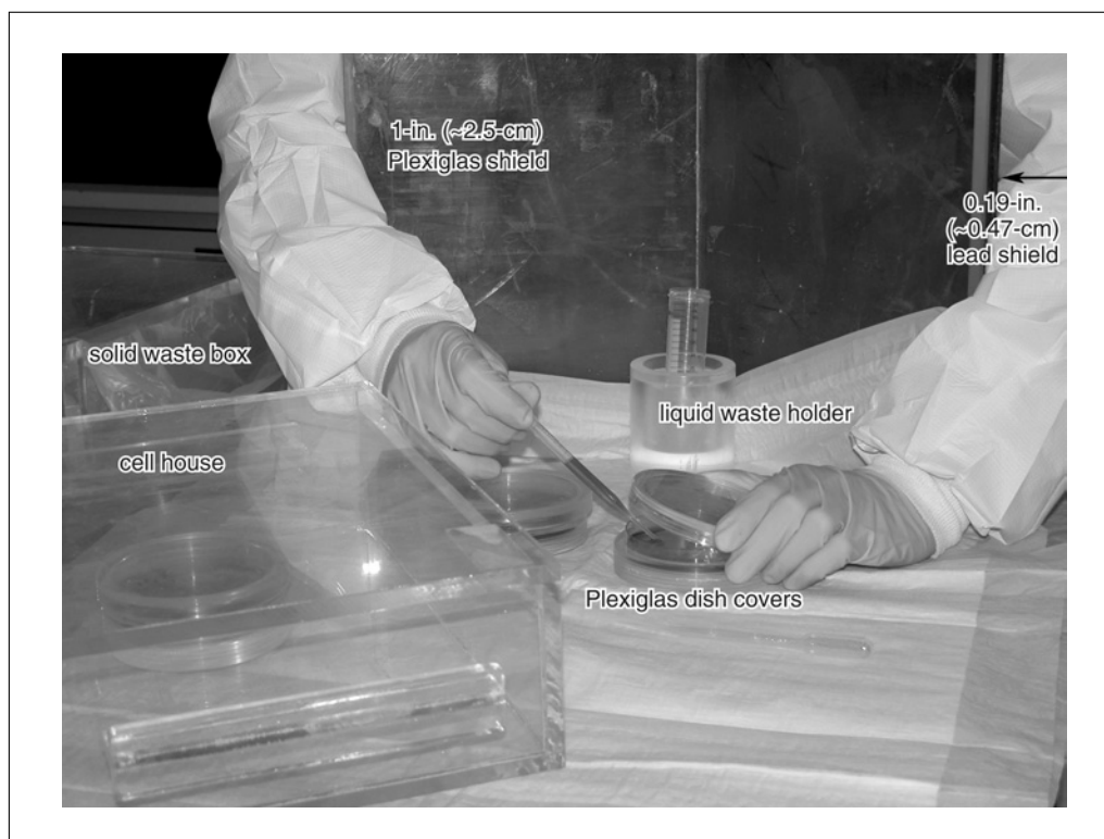
Figure 1A.4.3 Use of Plexiglas dish shields for ^{32}\text{P} labels reduces extremity exposure.
