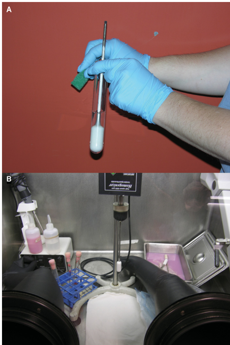
Figure 10A.5.5 (A) Homogenizing tube for mouse organs fitted tightly with a plastic pestle. (B) Homogenizer system with pestle fitted into the chuck.
