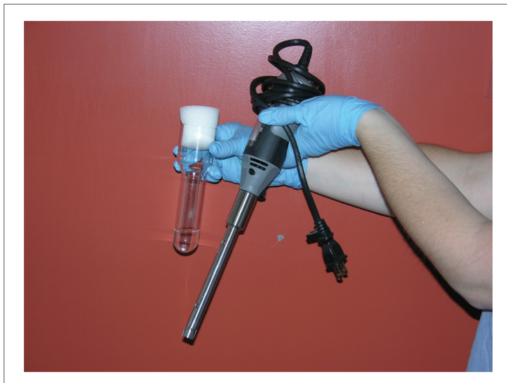
Figure 10A.5.7 Commercial tissue tearer that can be used to rapidly disrupt samples followed by processing for PCR techniques. The worker is holding the tissue sample in a homogenizing tube large enough for guinea pig tissues.
