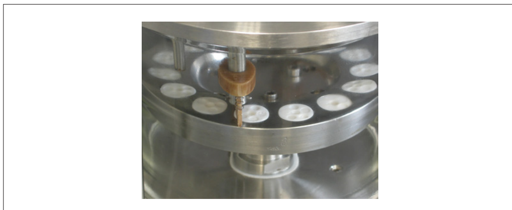
Figure 1B.5.8 Placement of pans in the CDFF.
