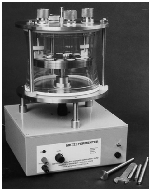
Figure 1B.5.1 The constant depth film fermentor complete with power unit and accessories.
