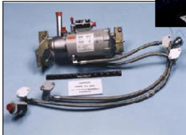
Trident Gas Hydraulic Assembly Turbopump
