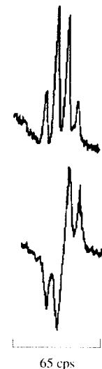
Fig. 7.5. CIDNP in CH 2 protons of CH 3 CH 2 MgI from the reaction of ethyl iodide with Mg in di- n -butyl ether [46]. Top: normal spectrum. Bottom: CIDNP spectrum ( E/A multiplet effect). This is the expected spectrum for CIDNP in RMgI formed in step r from radicals R • that have escaped from pairs [R • R • ] formed when independently diffusing radicals meet [47]. There were no indications of net effects, which would have been expected if diffusing radical pairs [R • •MgI] were significant generators of CIDNP [47]. Reprinted from Bodewitz et al. [46]. Copyright 1972. Page No. 283, with permission from Elsevier Science.
