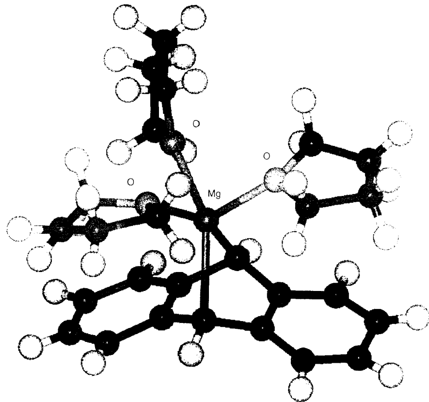
Fig. 1.1. Molecular projection of \text{Mg}(\text{anthracene})(\text{THF})_3 [32].
