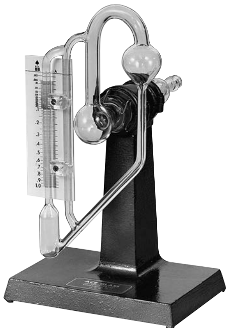
Figure 13.6 A tipping McLeod pressure gauge.
