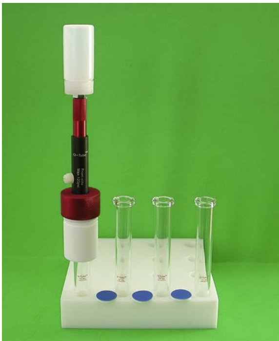
Figure 9.10 The Q-tube is loaded with reagents (up to 1.2 g of starting materials per 12 mL tube) and solvent (to one-third its volume) and sealed to the pressure monitor with a blue Teflon septum.
