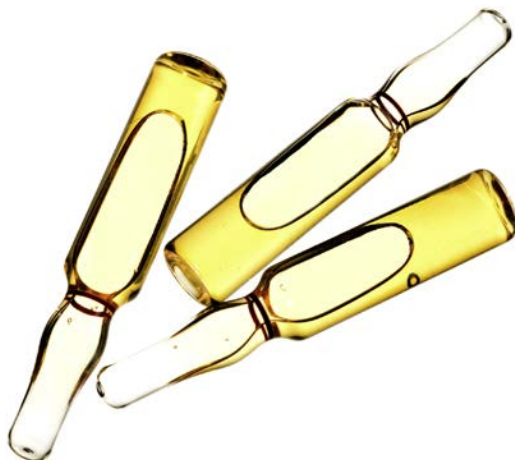
Figure 3.5 Reagents packaged in glass ampoules.
