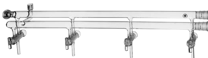
Figure 13.2 A glass double manifold for simultaneous manipulation of the atmosphere in a vessel, including vacuum and delivery of an inert gas.
