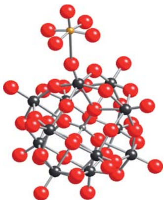
Figure 14.5 Schematic representation of the \text{FeO}(\text{H}_2\text{O})_3^+ counter-cation in interaction with the Keggin anion leading to a charge transfer between iron and molybdenum. Iron, yellow; molybdenum, black; oxygen, red.
