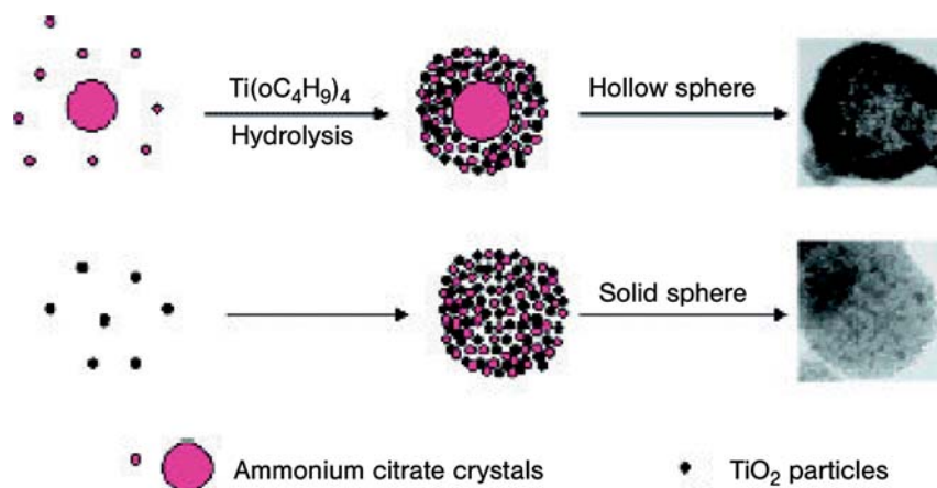
Figure 16.8 Schematic illustration of the formation mechanisms for mesoporous \text{TiO}_2 hollow and solid spheres (from [73]).
