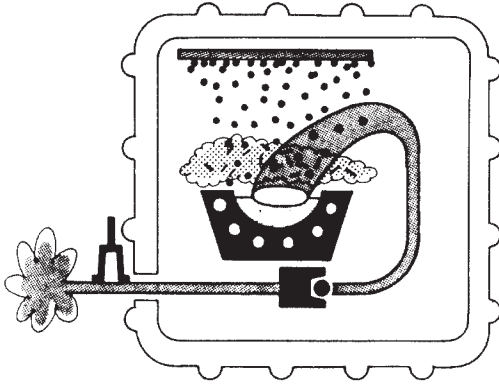
Fig. 22.2 Illustration of an electromagnetic beam deflection through 270^\circ in a vacuum evaporation system using an electron beam heating source. Source: Hill 1986
