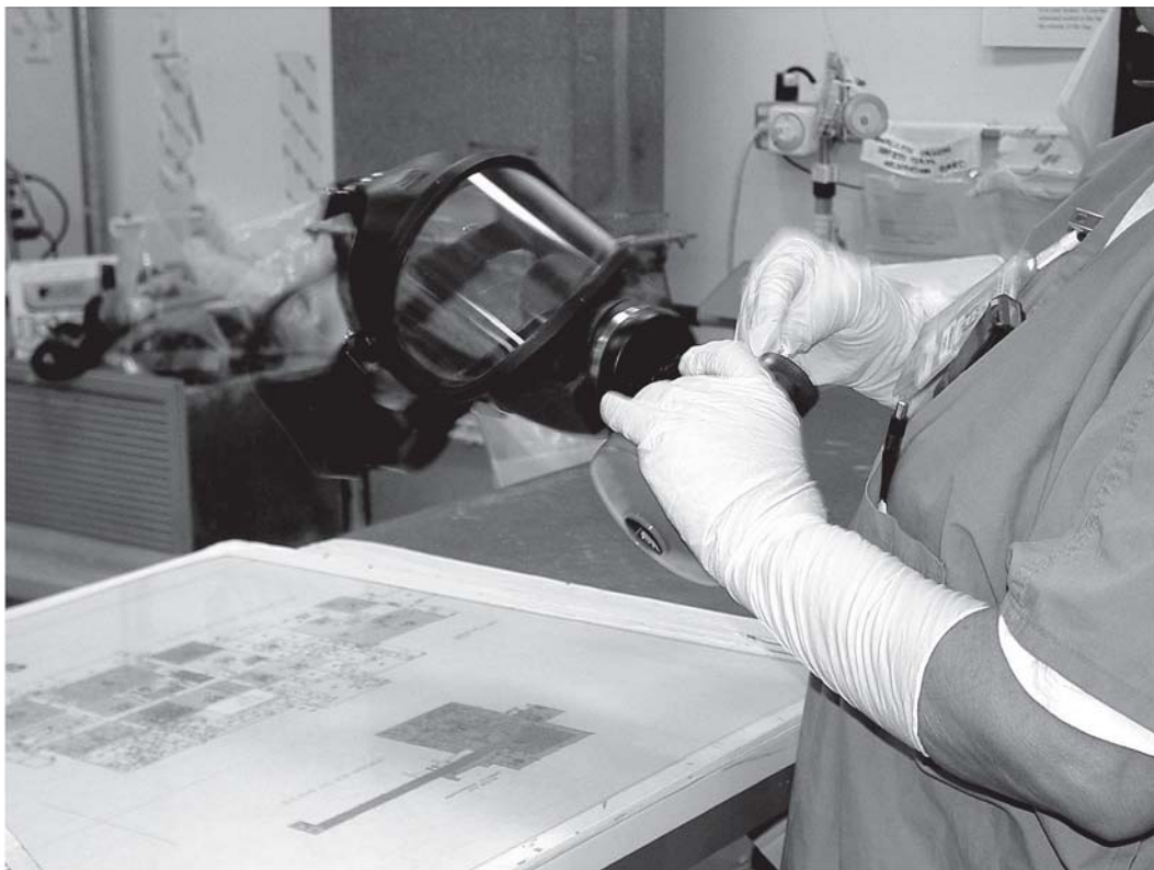
Fig. 29.2 Technician taking a smear sample for beryllium analysis from a recently used respirator. Also shown is a characterization survey map of the facility, listing results from routine surveys.
