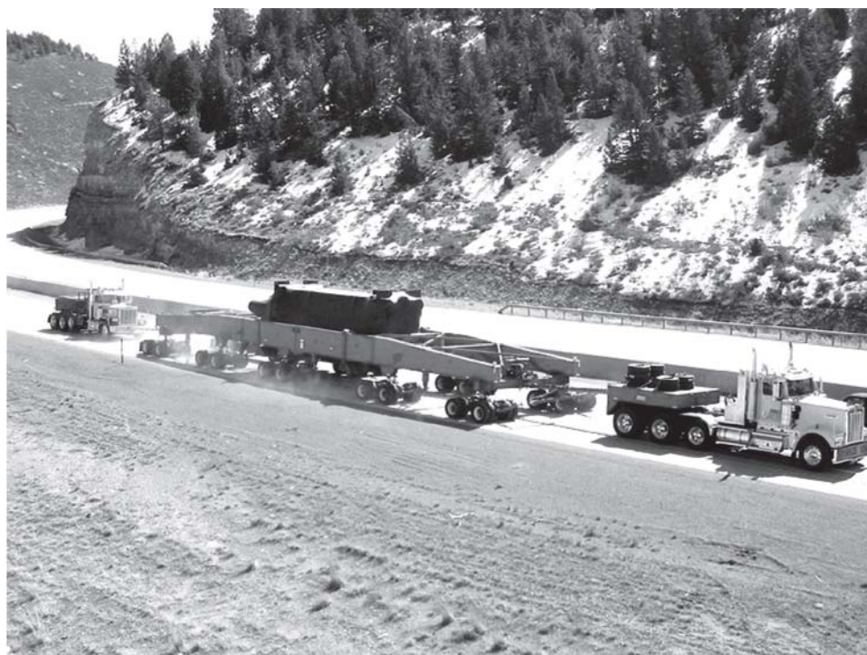
Fig. 29.6 (a) Large press contaminated with uranium and beryllium. It has been coated with a poly-urea-based coating and prepared for transport to a waste repository. (b) Large press, contaminated with uranium and beryllium and coated with a poly-urea-based coating, being transported to a waste repository
