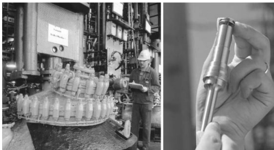
Fig. 8-6. The old (left) and new (right) reactors for the synthesis of dialkoxy-phenylphosphanes at BASF SE (reproduced by courtesy of BASF SE).
