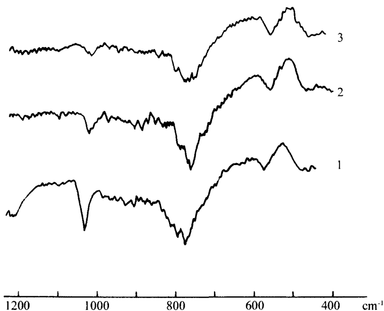
Fig. 94. IR emission spectra of molten system \text{LiNbOF}_4 - \text{LiF} at 660^\circ\text{C} . Curves 1, 2 and 3 correspond to \text{LiNbOF}_4 concentrations of 1.0, 0.8 and 0.6 molar fraction, respectively. Reproduced from [379], A. I. Agulyansky, E. L. Tikhomirova, V. T. Kalinnikov, Zh. Neorg. Khim. , 33 (1988) 1155, Copyright 1988, with permission of “Nauka” (Russian Academy of Sciences) publishing.
