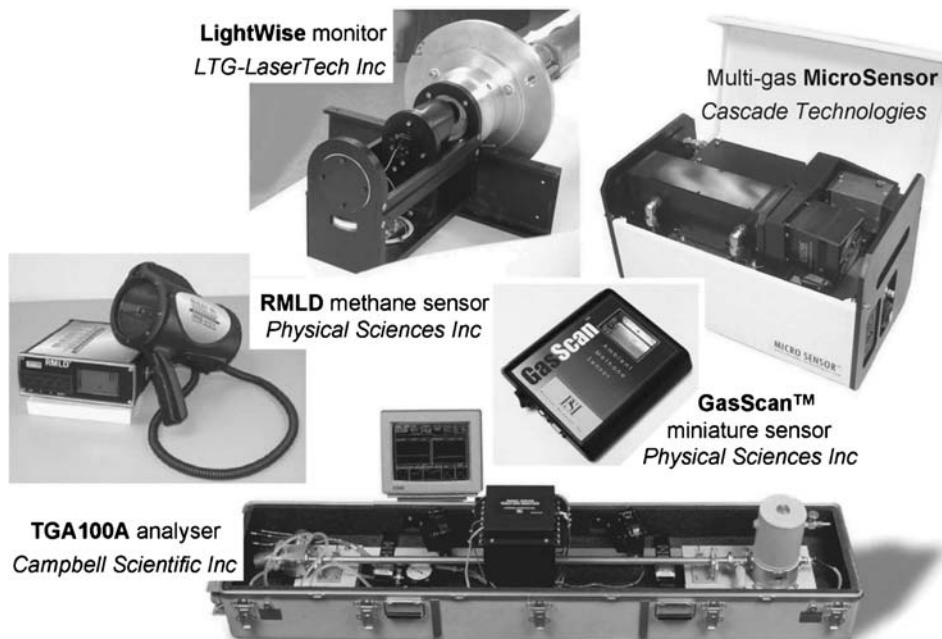
Figure 28.2 Selection of commercially available TDLAS systems. Clockwise, from top to bottom: universal dual-beam system with internal calibration cell, based on visible–near-IR laser diodes ( LTG-LaserTech Inc ); multispecies gas monitor, based on mid-IR QCLs ( Cascade Technologies ); miniature single-gas sensor, based on visible–near-IR laser diodes ( Physical Sciences Inc. ); single-/multi-gas system, based on mid-IR lead-salt lasers ( Campbell Scientific Inc. ); hand-held remote gas sensor, based on near-IR laser diodes ( Physical Sciences Inc. )
