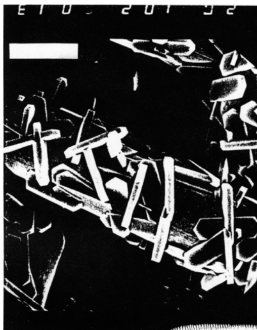
Figure 6. SEM picture of ZSM-5 crystals grown onto a stainless steel wire gauze. The wire diameter is 35 \mu\text{m} .
