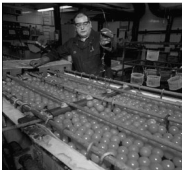
FIGURE 6.13 Example of manual rack plating line. The balls floating on top of the tank reduce solution evaporation.
