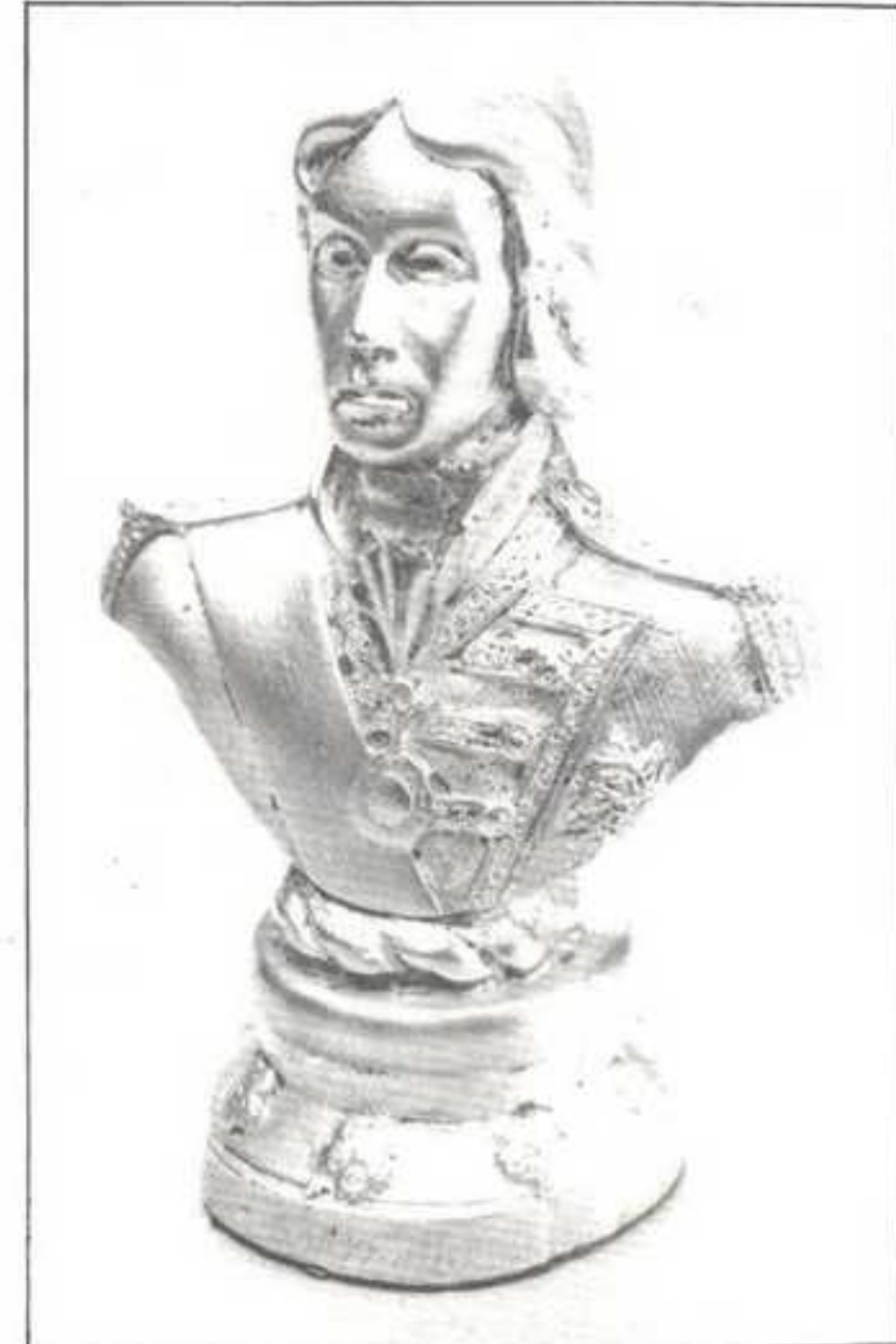
A moulded Araldite resin figure, sensitised with silver loaded paint, and electroplated.
