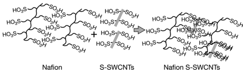
Fig. 9.11 Preparation of S-SWCNT/Nafion composite membrane by mixing solutions of each component. (From [11])
