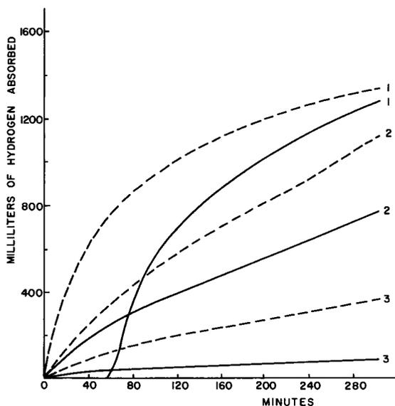
FIG. 1. Effect of stannous chloride on the rate of hydrogenation of heptaldehyde (one mole  $H_2 \equiv 1600$  ml at  $25^\circ C$ ): (1) 5% ruthenium-on-carbon, 1000 mg, (2) 5% platinum-on-carbon, 1000 mg, and (3) platinum oxide, 59.7 mg. Solvent: 44.5% v/v aqueous ethanol. Solid line = no promoter; broken line = one atom  $Sn^{++}$  per atom Ru or Pt.
