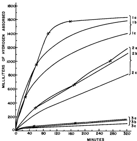
FIG. 2. Effect of oxygen on the rate of hydrogenation of heptaldehyde (one mole  $H_2 \equiv 600$  ml at  $25^\circ C$ ): (1) 5% ruthenium-on-carbon, 1000 mg, (2) 5% platinum-on-carbon, 1000 mg, and (3) platinum oxide, 59.7 mg; (a) intermittent shaking with air, (b) 1% oxygen (as air) in hydrogen, and (c) no oxygen;  $\times$  = hydrogen removed and solution shaken with air for 2 minutes. Solvent: 44.5% v/v aqueous ethanol.
