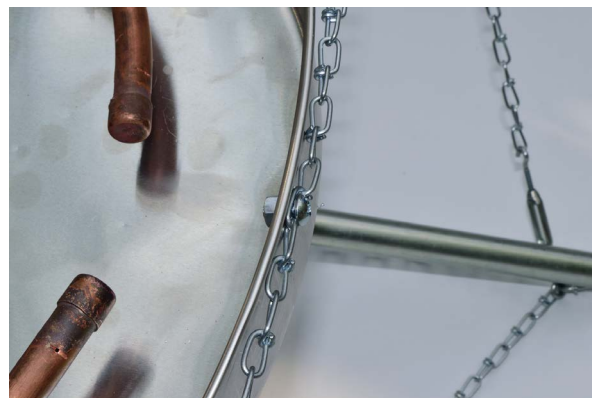
FIGURE 5-45: Step 8f, attaching the pan to the chains
