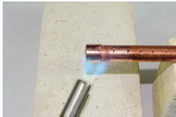
FIGURE 4-18: Heat the parts.
