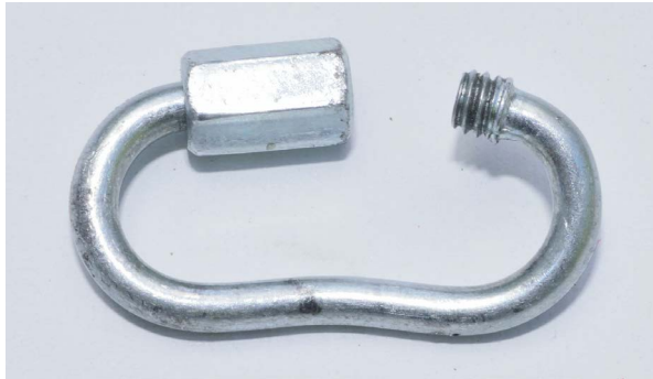
FIGURE 5-36: Bent quick link
