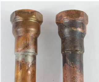
FIGURE 2-23: Soldered vs. brazed fitting
