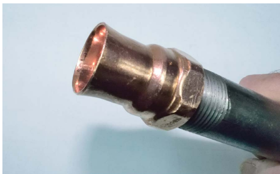
FIGURE 8-28: The completed mini-flare
