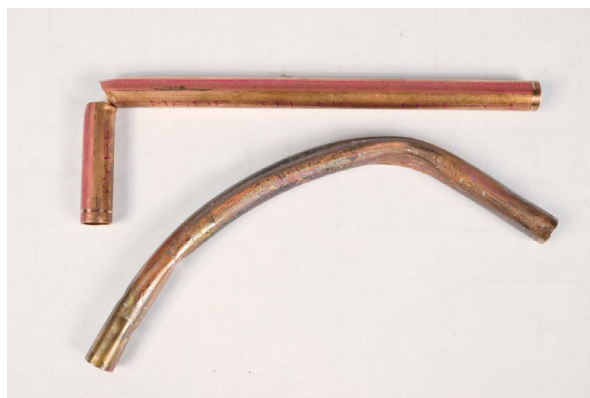
FIGURE 5-8: Failed bends in type M tubing
