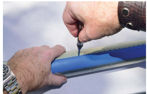
FIGURE 6-7: Make a divot at each mark.
