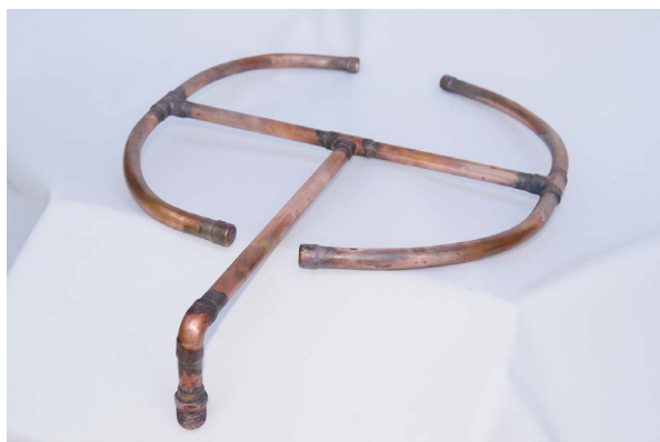
FIGURE 5-25: The brazed burner
