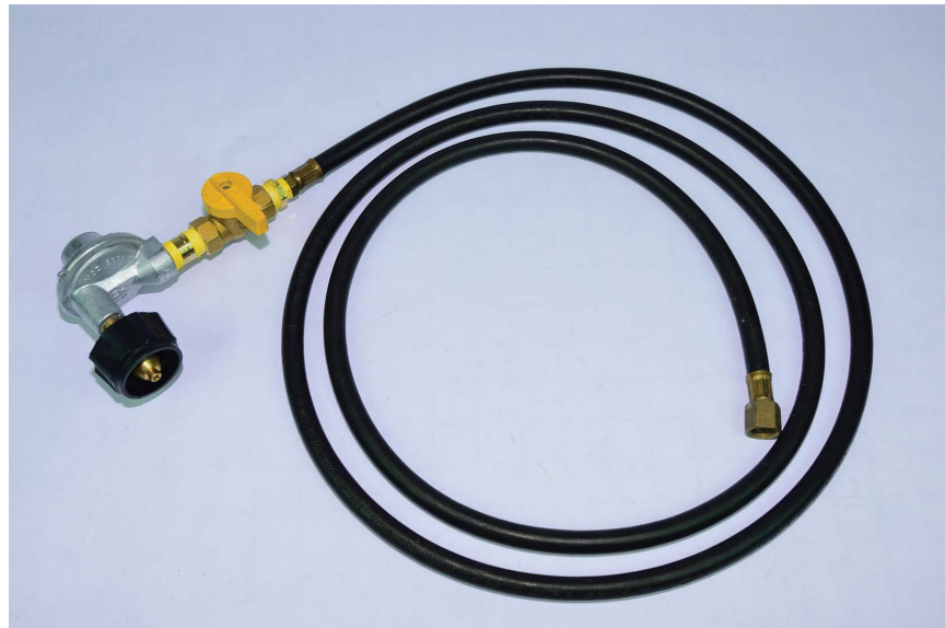
FIGURE 3-7: The completed low-pressure source
