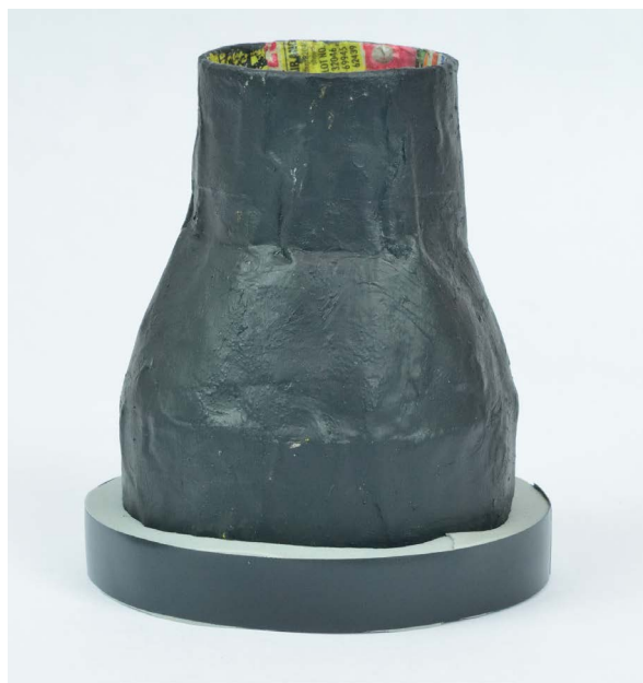
FIGURE 6-22: Attach foam to the connector.
