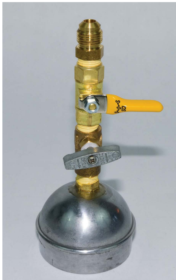
FIGURE 6-16: The fitting stack on the end cap
