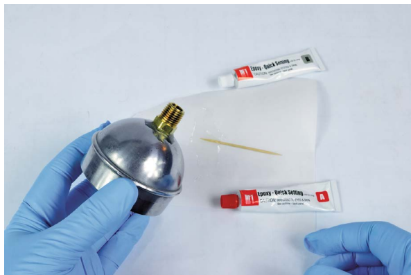
FIGURE 6-15: Epoxy the fitting into the end cap, leaving the clamp-able section of the fitting clean.
