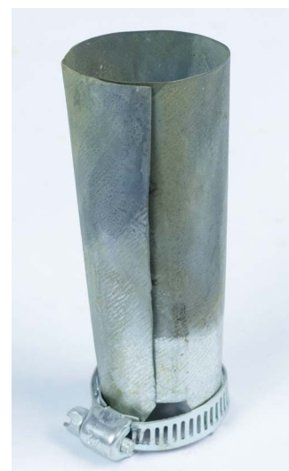
FIGURE 8-31: The completed sheet-metal flare
