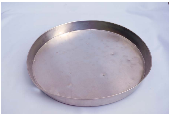
FIGURE 5-27: Punch some drain holes.
