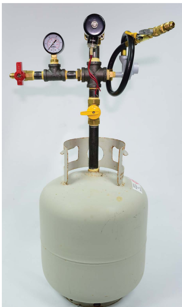
FIGURE 9-12: Main effect branch and plumbing tree
