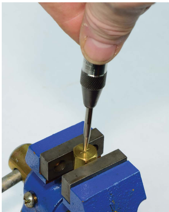
FIGURE 8-3: Mark the cap with a center punch.
