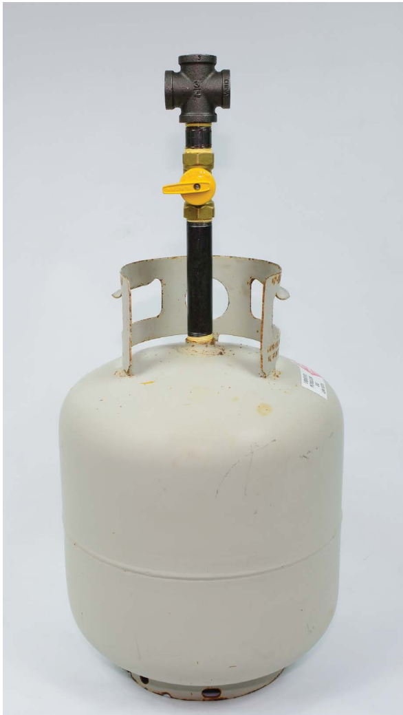
FIGURE 9-9: Accumulator branch
