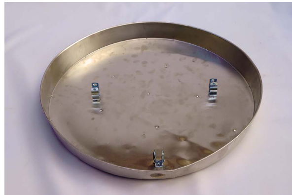
FIGURE 5-28: Hangers mounted in the pan
