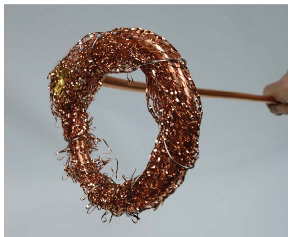
FIGURE 9-17: Scouring pad wind protection
