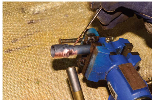
FIGURE 5-23: Braze the threaded adapter to the short arm.
