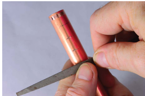
FIGURE 4-14: File a groove where each jet will go.
