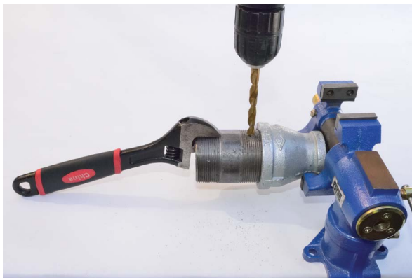
FIGURE 8-9: Drill the main holes for the tube to pass through.
