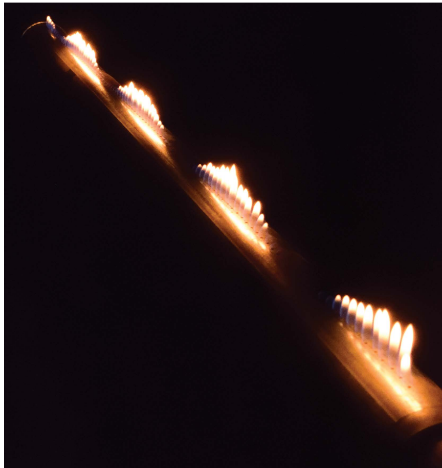
FIGURE 6-28: 460 Hz signal in the Rubens tube
