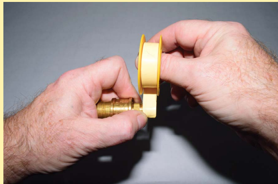
FIGURE 3-4: Taping, step two
