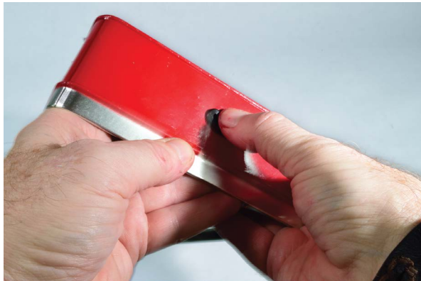
FIGURE 9-23: Mounting grommets
