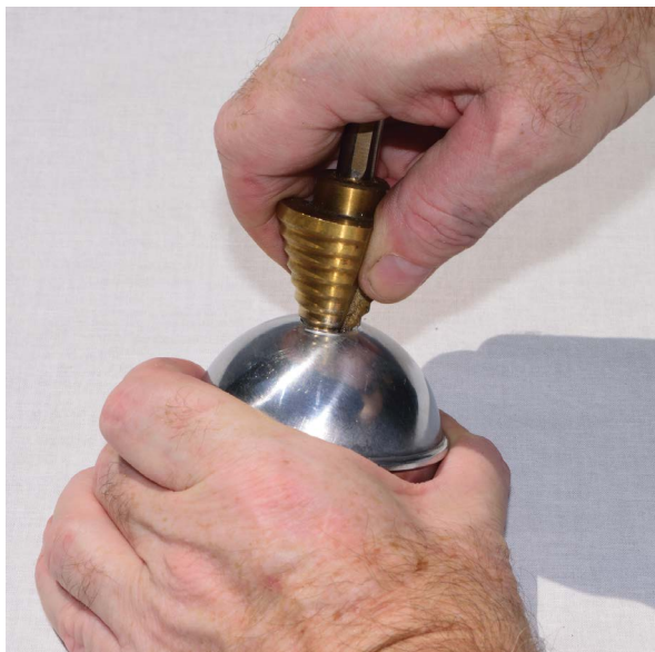
FIGURE 6-14: Ream the hole by hand with a step bit.
