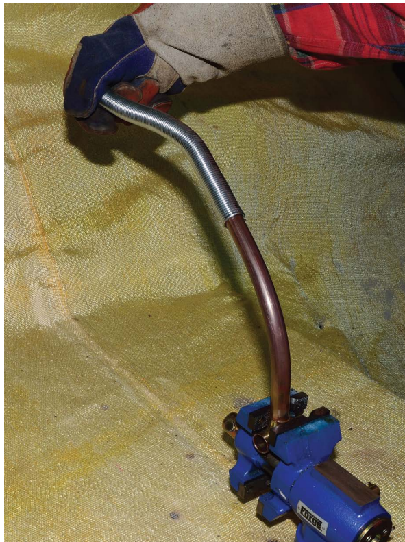
FIGURE 5-14: Twist and pull the spring off.
