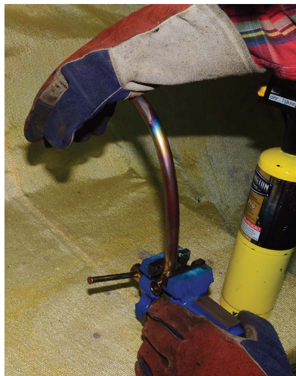
FIGURE 5-15: Complete the final bend without the spring.
