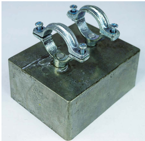
FIGURE 12-23: Mounts attached to the case
