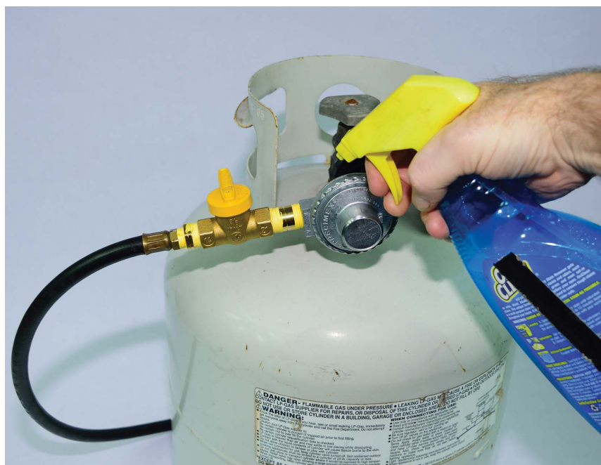
FIGURE 3-9: Leak-test the low-pressure source
