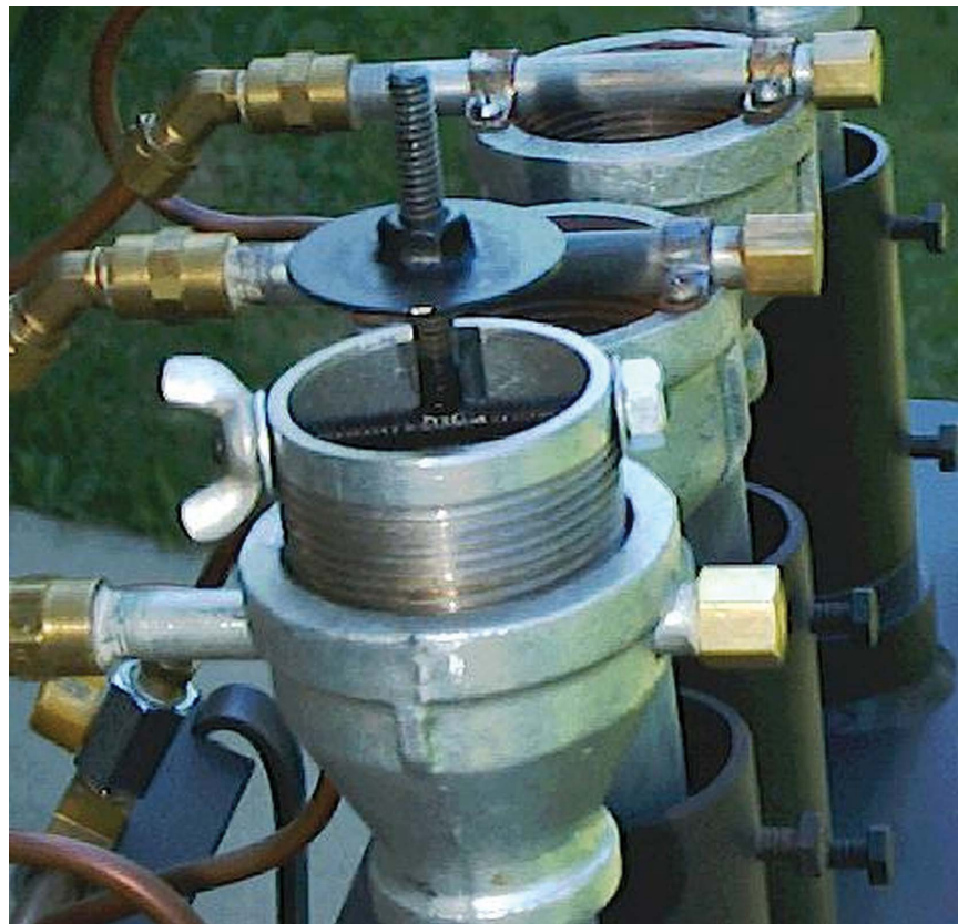
FIGURE 8-32: Upscale axial choke
