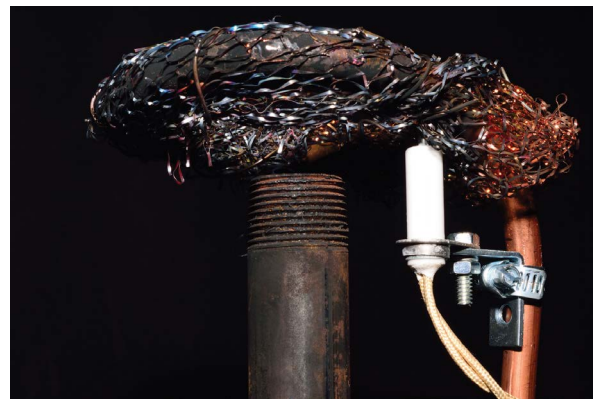
FIGURE 10-5: The mounted igniter
