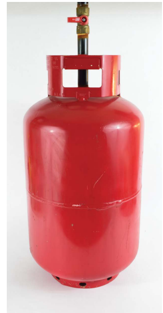
FIGURE 2-20: Repurposed propane cylinder used as an accumulator
