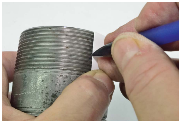
FIGURE 8-8: Mark a line on one side of the pipe.
