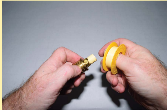
FIGURE 3-6: Taping, step four
