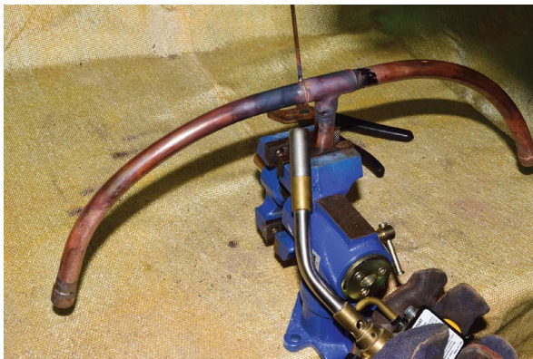
FIGURE 5-21: Braze the bent arms into the tee.
