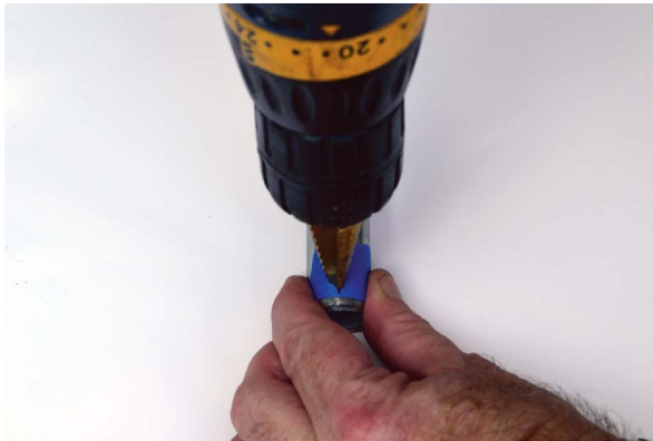
FIGURE 5-34: Drill the final hole with the step drill bit.
