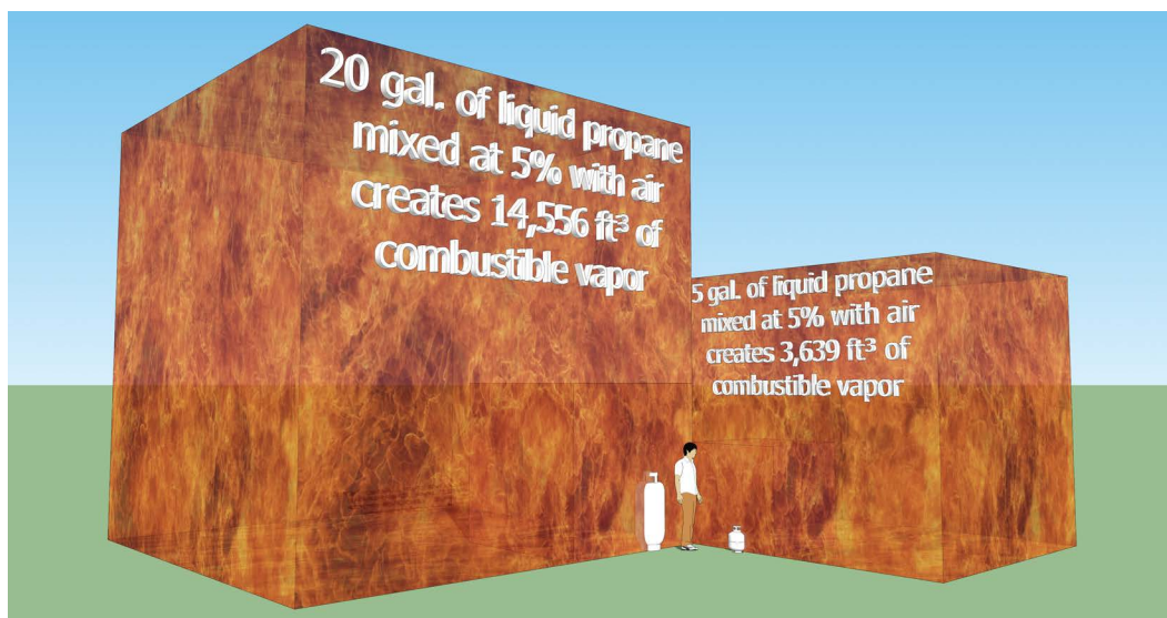
FIGURE 1-5: Mixed with air, the combustible mixture is 20 times larger than propane vapor alone.
