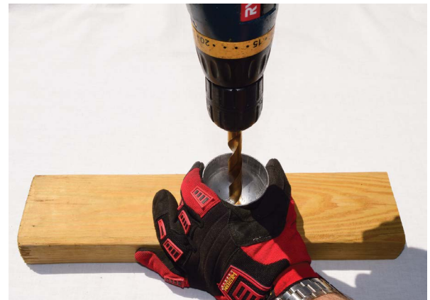
FIGURE 6-13: Drill the hole for the fitting in the end cap.
