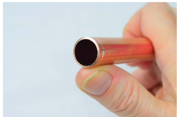
FIGURE 4-9: The cut tube has a flanged lip.
