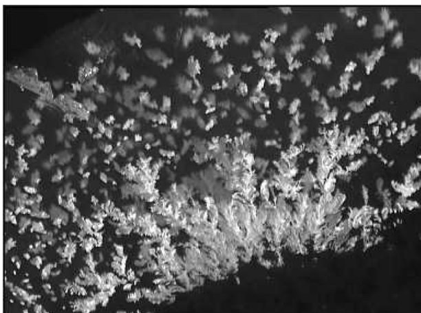
Fig. 12. Picture of the aerogel sample having naphthalene crystals inside.
