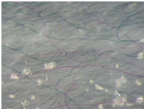
Figure 11. Fibre disorientation in rotor grooves.
