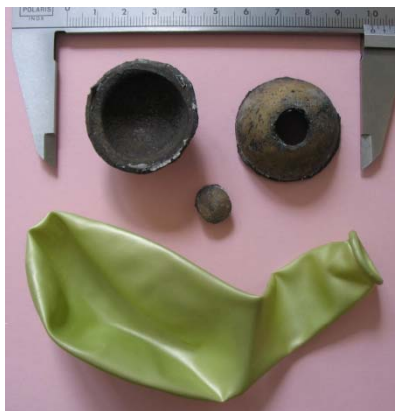
Figure 2. Rubber mould and balloon used for making spherical BN+ZrO 2 coated samples.
