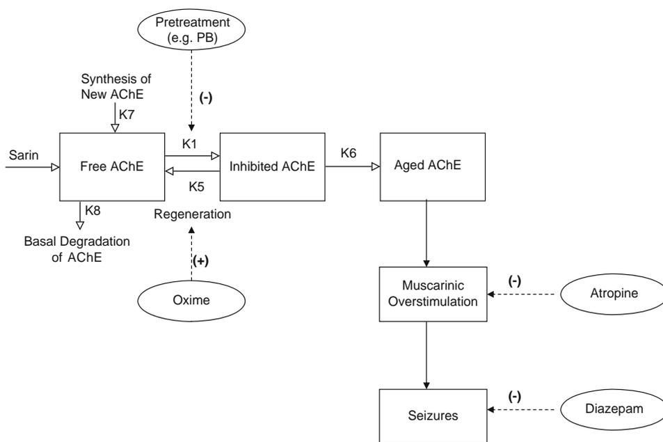
**FIGURE 62.3.** Schematic for AChE inhibition by nerve agents such as sarin, together with the interaction of pretreatment [pyridostigmine bromide (PB)] and countermeasure treatment (oxime, atropine, and diazepam). Pyridostigmine acts as a reversible cholinesterase inhibitor, oxime acts as an AChE regenerator, atropine acts as a muscarinic receptor antagonist, and diazepam acts as a positive allosteric modulator of GABA.
