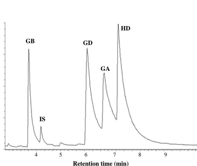
**FIGURE 53.5.** GC-MS data of portable apparatus, Hapsite. Left: total ion chromatogram; right: electron ionization mass spectra. GB, GD: 1 mg/m<sup>3</sup>; GA: 3 mg/m<sup>3</sup>; HD: 0.5 mg/m<sup>3</sup>. IS: internal standard.
