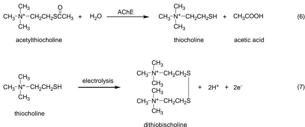
**SCHEME 55.4.** Enzyme and electrochemical reactions in acetylthiocholine-based sensors.
