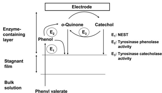
**FIGURE 57.14.** Schematic representation of the pathway that leads to the generation of current in the bi-enzyme biosensor containing tyrosinase and neuropathy target esterase catalytic domain (NEST). Reproduced with permission from Kohli *et al.* (2007a).
