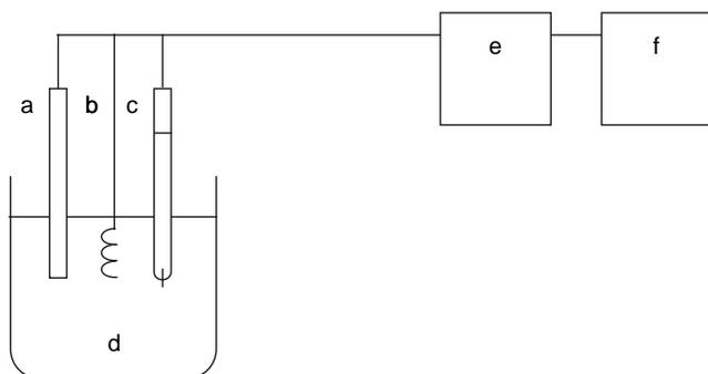
**FIGURE 55.2.** An experimental set-up for operation of electrochemical biosensors. (a) Biosensor, (b) counter electrode, (c) reference electrode, (d) sample solution, (e) potentiostat, and (f) recorder. (Reproduced from Anzai, 2006, with permission).
