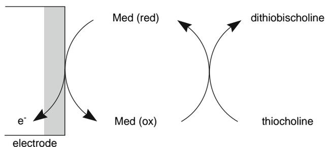
**FIGURE 55.5.** An electrochemical oxidation of thiocholine through electron transfer mediator. Med (red) and Med (ox) represent electrode transfer mediator in reduced and oxidized forms. (Reproduced from Anzai, 2006, with permission).
