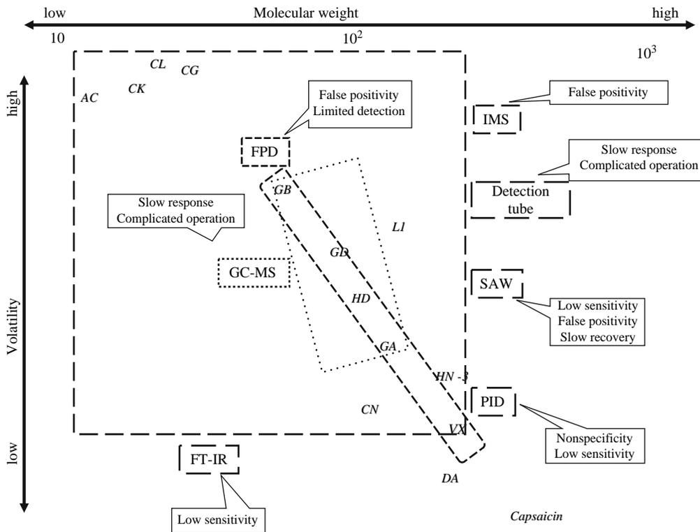
**FIGURE 53.6.** Performance of on-site chemical warfare agent detection equipment.
