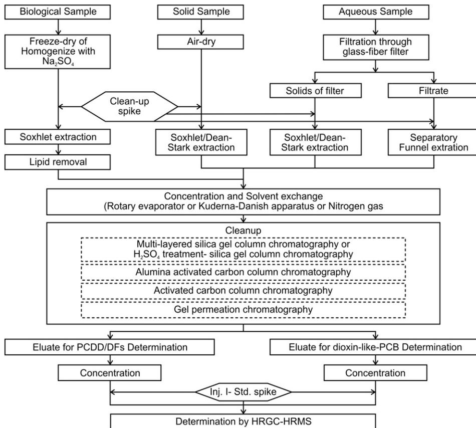
**FIGURE 18.4.** Analytical procedures of dioxins and “dioxin-like PCBs”.
