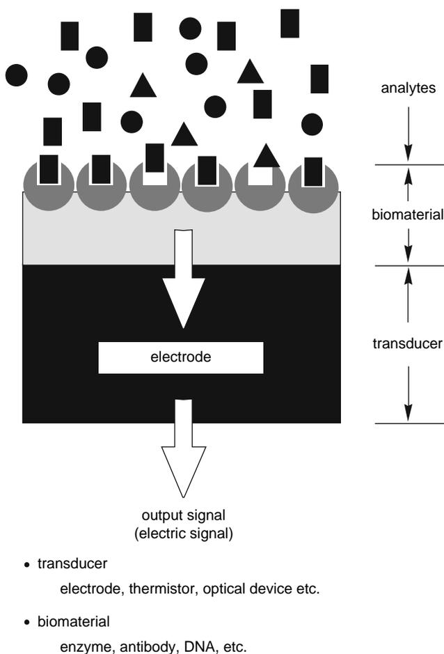
**FIGURE 55.1.** A schematic illustration of the structure of biosensors. (Reproduced from Anzai, 2006, with permission).
