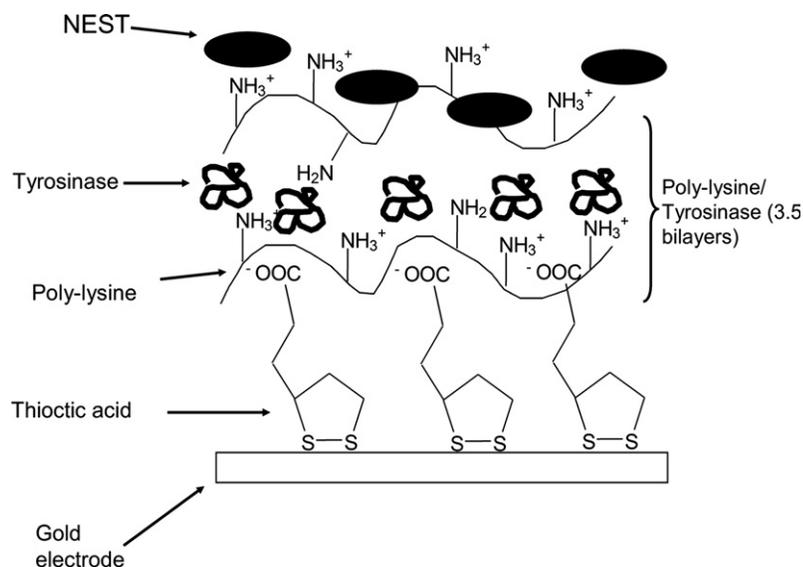
**FIGURE 57.13.** Molecular architecture of bi-enzyme biosensor electrode containing tyrosinase and neuropathy target esterase catalytic domain (NEST). Reproduced with permission from Kohli *et al.* (2007a).
