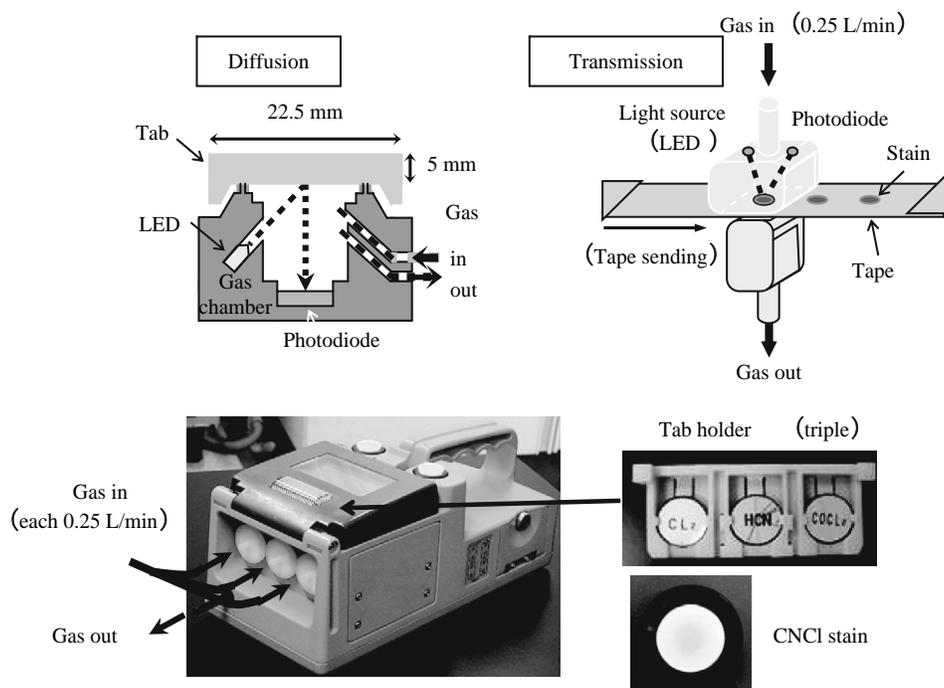
**FIGURE 53.8.** Monitoring tape method. Schematic detection mechanism of diffusion (upper left) and transmission (upper right) types of apparatus and arrayed diffusion-type detector (lower).
