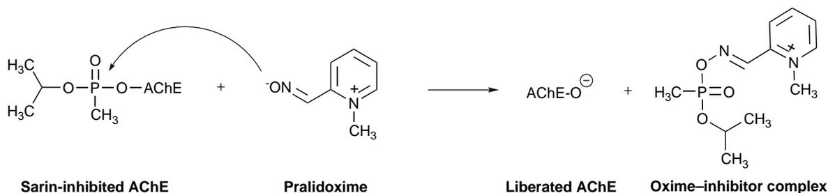
**FIGURE 66.4.** Reactivation of sarin-inhibited acetylcholinesterase.
