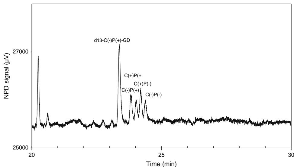
**FIGURE 54.1.** Large volume (200–400  $\mu$ l) thermal desorption from TENAX (300 mg, TA 60–80 mesh) followed by 2D-GC and MS detection in EI mode. (1) Pre-column. (2) Analytical column. Small part of the chromatogram of the first column is reinjected on the second analytical column. From: Trap and Van der Schans (2007), Figures 3 and 4.
