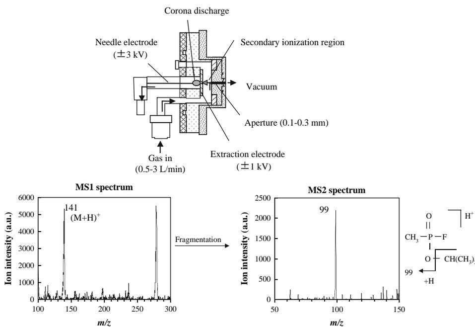
**FIGURE 53.7.** Counterflow introduction/atmospheric pressure chemical ionization mass spectrometer. Upper: structure of ionization chamber; lower: exemplified mass spectra of GB.
