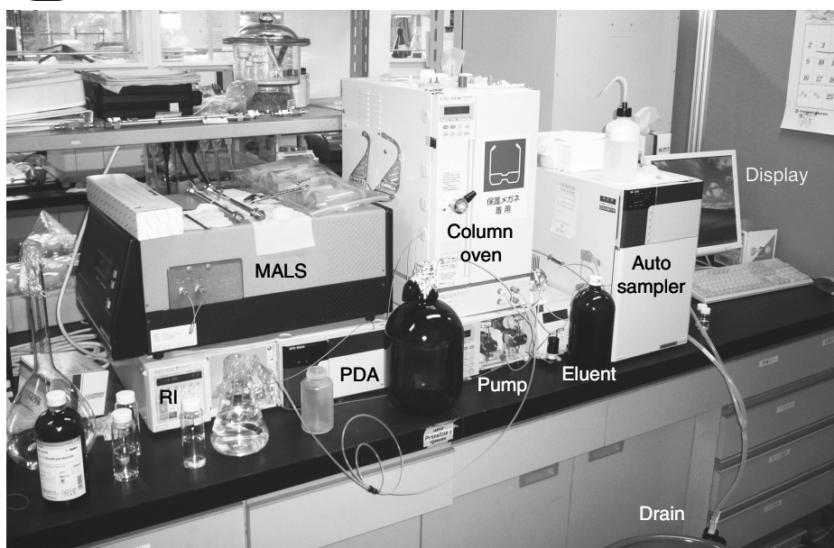
Figure 12.4 Schematic representation and photograph of our SEC-PDA-MALS-QELS system.
