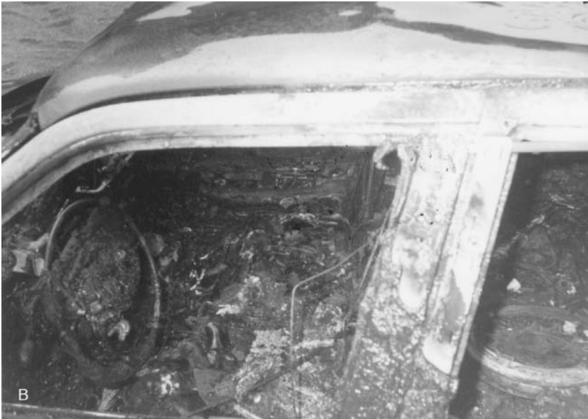
FIGURE 9.2 Photographs of a car damaged by an oxygen-enriched fire.
