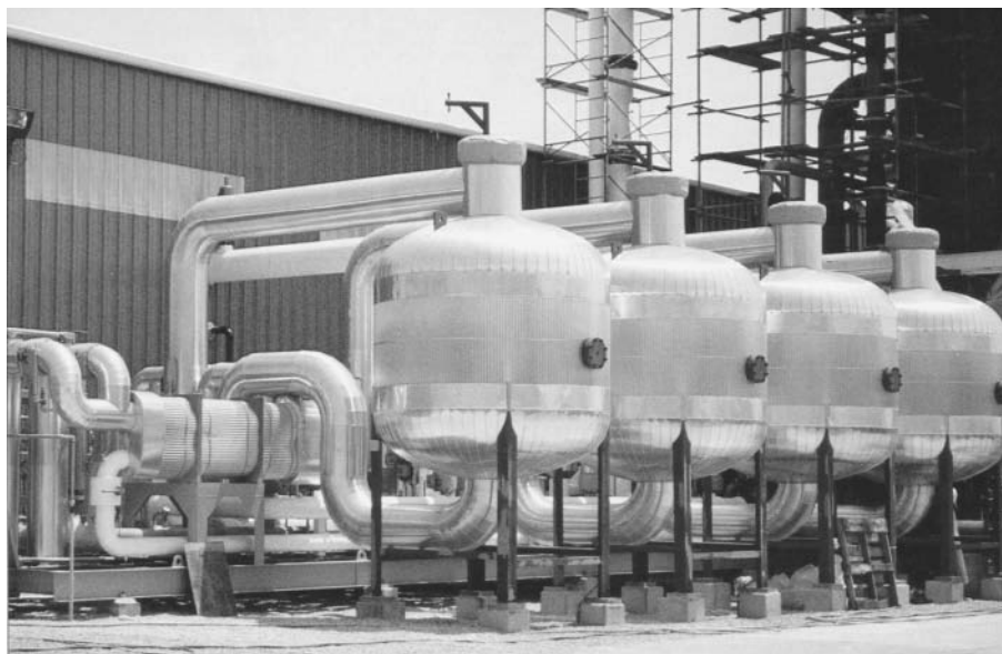
FIGURE 3.34 Four-bed temperature swing adsorber installation. (Courtesy of Chemical Design Inc.)
