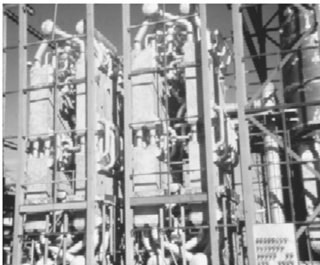
FIGURE 3.39 Manifolded core assembly. (Courtesy of Air Products.)
