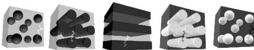
Figure 7 The classical morphologies in block copolymer systems.
