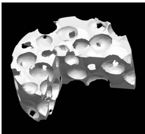
Figure 3 3D computerized tomography (CT) image of a foamed polysiloxane incorporating a small admixture of carborane cages.
