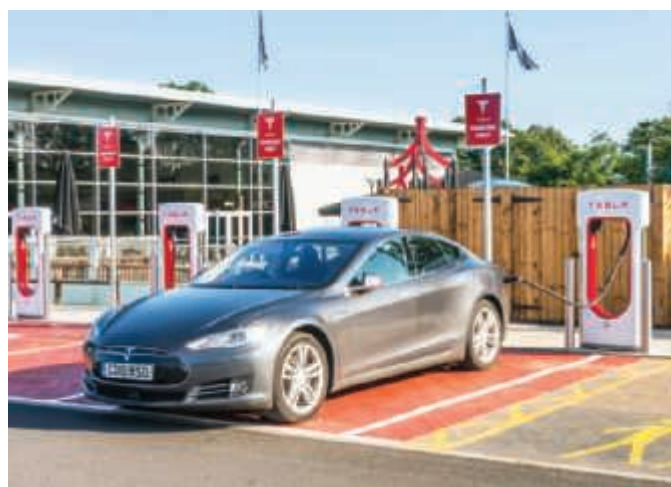
▲ Figure 20.22 Electric car. This Tesla electric automobile can go about 200 miles after 30 minutes of charging at this station.
