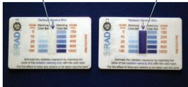
▲ Figure 21.8 Badge dosimeters monitor the extent to which the individual has been exposed to high-energy radiation. The radiation dose is determined from the extent of darkening of the film in the dosimeter.
