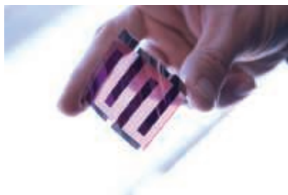
▲ Figure 12.43 Plastic electronics. Flexible organic solar cells are made from conducting polymers.
