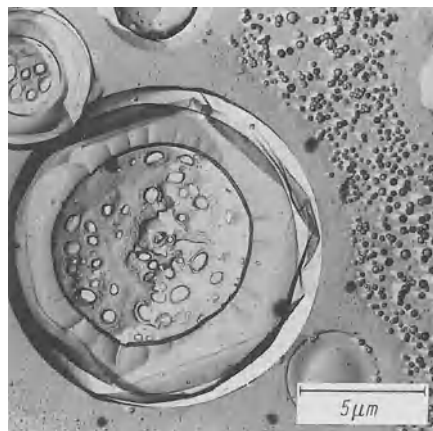
Fig. 6.21. Electron-optical micrograph of a barium borosilicate glass after \text{HNO}_3 etching and replica preparation. The glass consists of four glass phases. In the matrix phase, diffusion halos around the large-droplet phase can be recognized. The large droplets are surrounded by an \text{SiO}_2 shell
