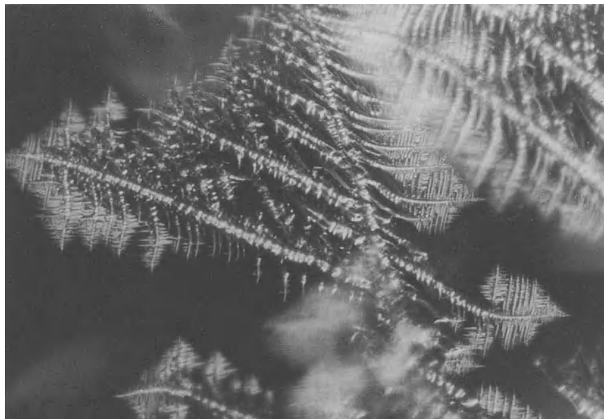
Fig. 10.11. Dendrite precipitation of crystal skeletons resembling water plants in a \text{BeF}_2 glass (250:1)
