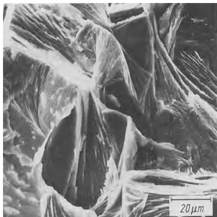
Fig. 10.37. Large sodium phlogopite crystals ( \text{Na}_{0.5-1}\text{Mg}(\text{AlSi}_3\text{O}_{10}\text{F}_2) ) in a base glass of the system \text{Na}_2\text{O}-\text{MgO}-\text{Al}_2\text{O}_3-\text{SiO}_2-\text{F} (scanning electron micrograph)
