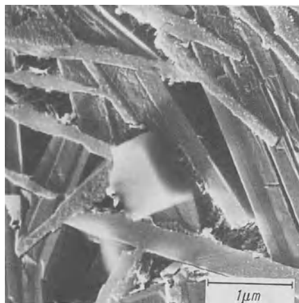
Fig. 10.53. Machinable glass ceramic which also contains cubic spinel mixed crystals II of the type \text{Mg, Fe}^{\text{II}} (\text{Fe}^{\text{III}}\text{Al}_{1-x})_2\text{O}_4 aside from biotite mica crystals
