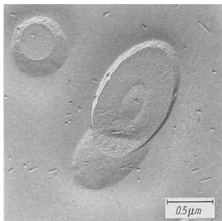
Fig. 10.75. Single crystallite from Fig. 10.74. An iron phosphate primary nucleus obviously grows by an epitaxial interaction with apatite
