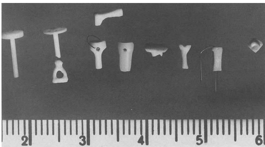
Fig. 10.83. Middle ear implants of machinable biocompatible and bioactive glass-ceramics which were made by the physician himself; scale: cm (Dr. E. Beleites, HNO Clinic of the Friedrich Schiller University in Jena)
