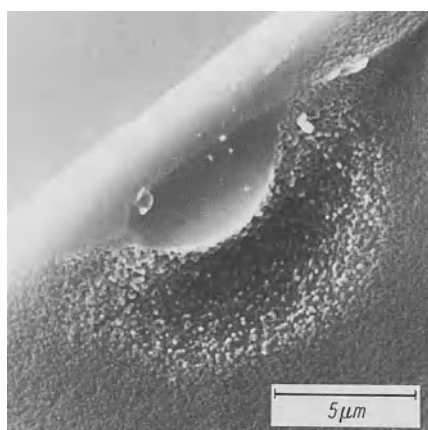
Fig. 5.50. Enlarged section of Fig. 5.49. Fracture surface perpendicular to the trace. The micrograph clearly shows structure modifications of the glass caused by thermal effects (electron absorption) in the immediate vicinity of the trace
