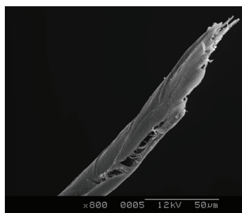
Fig. 9. External cracks after fatigue test (Cotton I)
