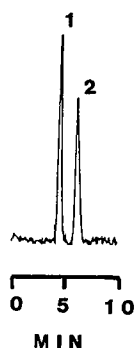
Fig. 9.15. HPLC-DCP chromatogram for the separation-detection of selenite and selenate species under paired-ion, RP conditions: C-18 column (10 \mu\text{m} , 15 cm \times 3.9 mm i.d.); mobile phase of 2.5 mM TBAHS, 0.01 M each dipotassium hydrogen phosphate and potassium dihydrogen phosphate, pH = 6.55; flow rate 0.5 ml min -1 ; DCP detection at 196.026 nm; injections of 50 \mu\text{l} of 20 ppm each Se species as standards. Peak identities: 1 = selenite; 2 = selenate. (Reprinted with permission of the copyright owner, The American Chemical Society and the ACS Symposium Series [50].)
