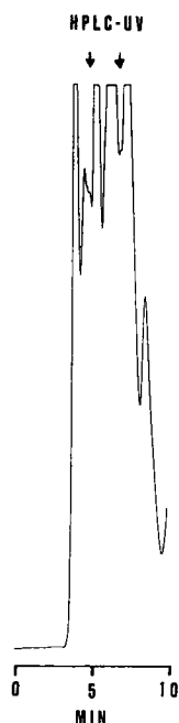
Fig. 9.16. HPLC-UV chromatogram of feed premix sample containing nominally 100 ppm Se each as selenite and selenate species. HPLC-UV chromatogram of separation of standard selenite and selenate species (20 ppm Se) under paired-ion, RP conditions: C-18 column (10 \mu\text{m} , 15 cm \times 3.9 mm i.d.), RP-300 C-8 guard column (7 \mu\text{m} , 3 cm \times 4.6 mm), pre-column Lichrosorb Si60 (30 \mu\text{m} , 2 cm \times 3.9 mm); mobile phase of 2.5 mM TBAHS, 0.01 M each dipotassium hydrogen phosphate and potassium dihydrogen phosphate, pH = 6.55; flow rate 0.5 ml min -1 ; UV detection at 205 nm; injections of 50 \mu\text{l} of 20 ppm each Se species as standards. Peak identities: 1 = selenite; 2 = selenate; 3 = system. (Reprinted with permission of the copyright owner, The American Chemical Society and the ACS Symposium Series [50].)
