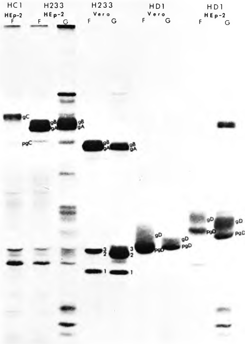
FIGURE 7. Autoradiograms of electrophoretically separated polypeptides labeled with 35 S-methionine and immunoprecipitated from HSV-1(F) and HSV-2(G) infected Vero and HEp-2 cells with hybridoma antibodies HC1, H233, and HD1.
