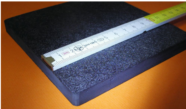
Figure 23.14. Tile of a carbon aerogel for high-temperature thermal insulation with carbon-fiber paper covering layers on both sides to enhance mechanical stability [38].
