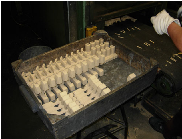
Figure 34.18. Core production in a foundry using m-silica aerogel as a nanoadditive (with permission of the company).
