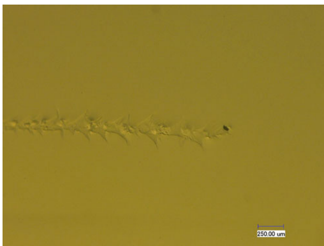
Figure 32.4. Entry track produced by the capture of 50 \mu\text{m} hypervelocity fine particle in silica aerogel. The aerogel shown was gradient density 15–50 \text{mg/cc} .
