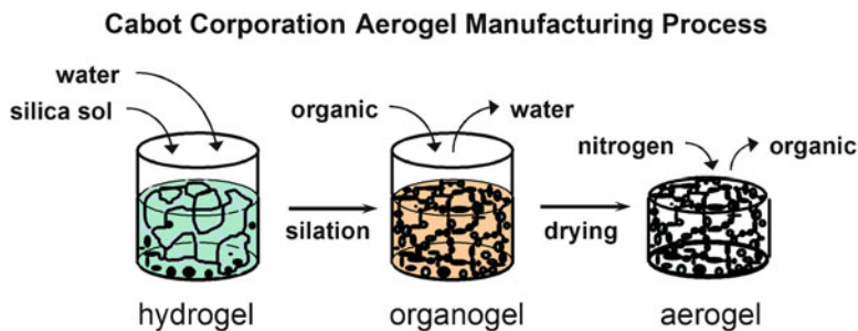
Figure 38.1. Schematic of Cabot's aerogel manufacturing process.
