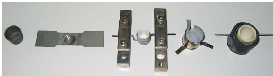
Figure 4 Various apparatus for metal containment for resistive heating (from left to right): small molybdenum crucible; tantalum boat; alumina crucible inside coiled tungsten winding, shown positioned between two electrical terminal blocks; tantalum heat shield surround for crucible; alumina crucible in shielded and insulated tungsten winding.
