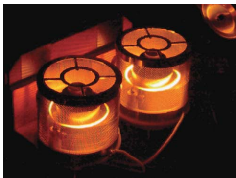
Figure 8 Twin electron-beam furnaces with skeleton lids.
