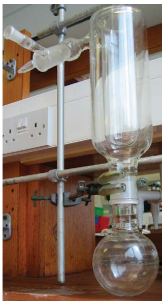
Figure 16 High-vacuum sublimation apparatus for recovery of volatile solid ligands; RBF diameter 100 mm.
