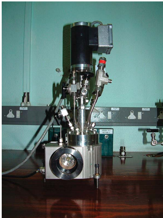
Figure 2 High pressure IR transmission cell.
