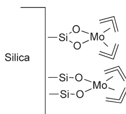
Figure 23 Different modes of attachment of the [\text{Mo}(\eta^3\text{-allyl})_2] fragment to silica.
