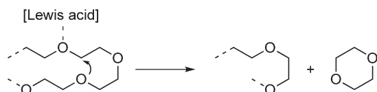
Scheme 2 Polymerization of epoxide in a cationic mechanism and a possible side reaction.
