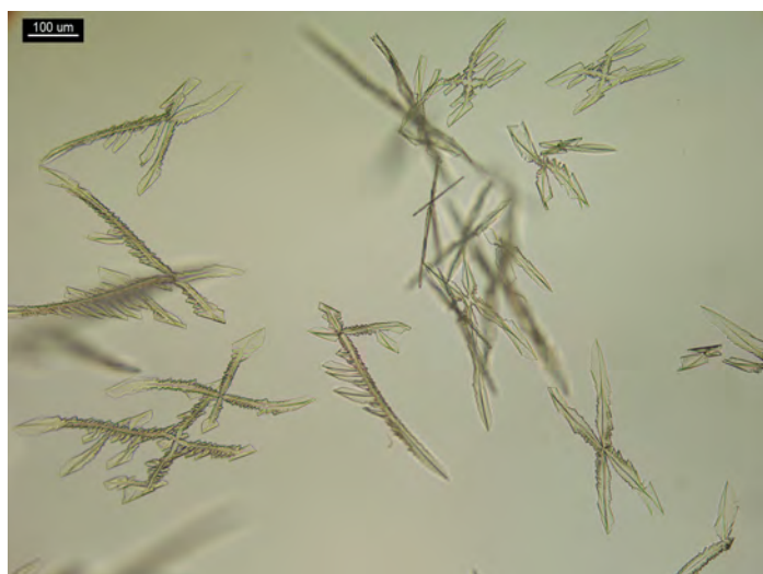
Figure 4. Direct test: 1 PPP of dl -methamphetamine and 5 μL of H 2 PtCl 6 reagent. Crystals form feathery X shapes.
