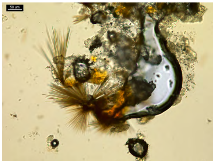
Figure 6. 10 PPP from a 2 mg hydromorphone pharmaceutical tablet and 15 µL of reagent mixture. Crystals form rosettes of needles.
