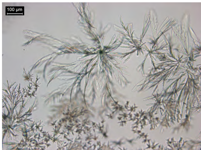
Figure 3. 1 PPP of heroin in 5 µL of 1% HCl and 5 µL of HgCl 2 reagent. Crystals form feathery dendrites.
