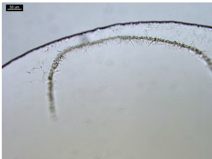
Figure 5. Volatility test: 2 PPP of d -amphetamine and one drop of 40% NaOH; crystals in a 5 μL hanging drop of H 2 PtCl 6 reagent. Crystals grow from a crust that forms at the edge of a hanging drop. Sometimes the crystals detach and move towards the center of the hanging drop.
