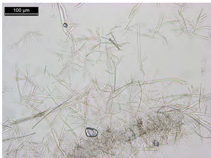
Figure 9. Volatility test: One drop of 40% NaOH added to 3 PPP of dl -amphetamine. Crystals formed in a 5 μL hanging drop of H 2 PtCl 6 reagent for 5 minutes. The coverslip with the hanging drop was removed from the reaction chamber and placed face-down onto the glass slide.
