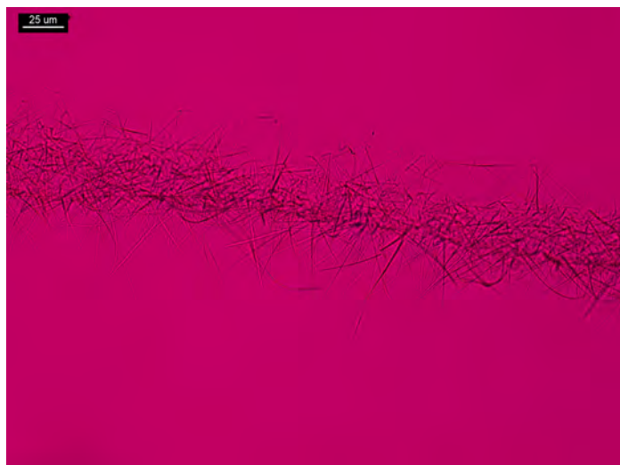
Figure 7. Same as Figure 6. Crystals appear nearly isotropic; crossed polars and Red I compensator.
