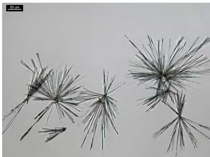
Figure 2. 5 PPP of morphine and 5 μL of HgCl 2 reagent form rosettes of needles; no coverslip.
