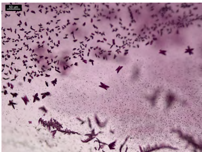
Figure 3. 1 PPP of PCP in 5 μL of 20% HOAc and 5 μL of \text{KMnO}_4 reagent. Crystals form bow ties, butterflies, rectangles and X shapes.
