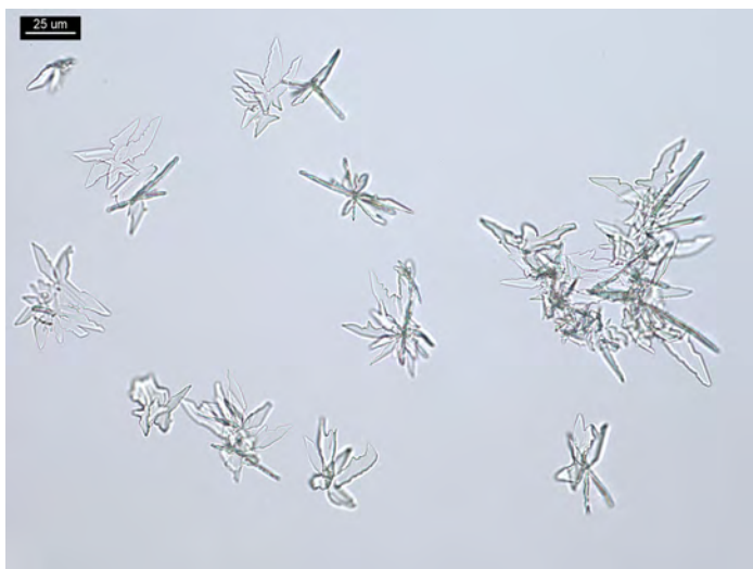
Figure 3. Direct test: 2 PPP dl -amphetamine dissolved in 5 μL of concentrated H 3 PO 4 and 5 μL of H 2 PtCl 6 reagent.
