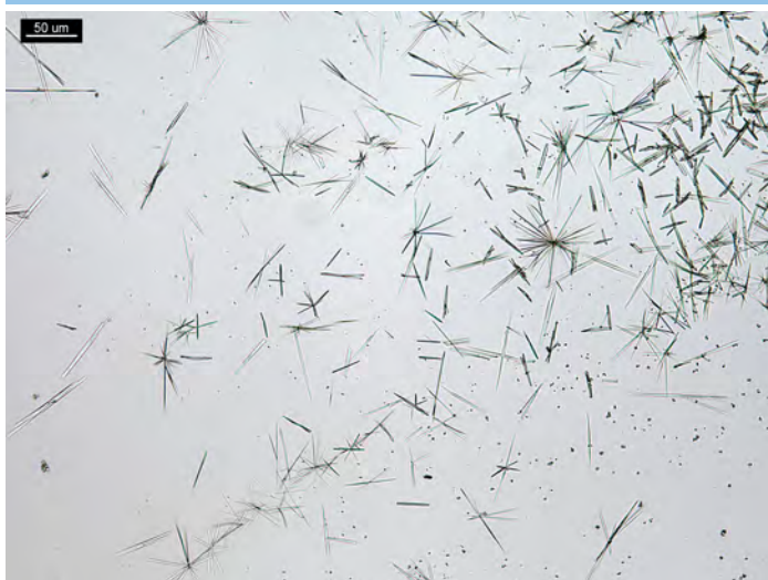
Figure 1. 1 PPP of clonazepam with 5–10 \mu\text{L} of \text{H}_2\text{PtCl}_6 reagent. Crystals form narrow blades and rods, sometimes arranged as rosettes.
