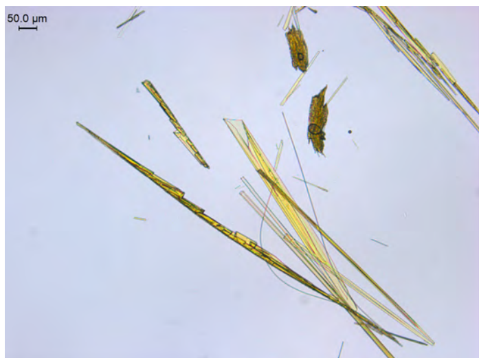
Figure 6. Volatility test: 2 PPP of d -amphetamine and one drop of 40% NaOH; crystals in a 5 μL hanging drop of HAuCl 4 reagent. Crystals form long yellow rods. Note the segmented and serrated morphology in some crystals.
