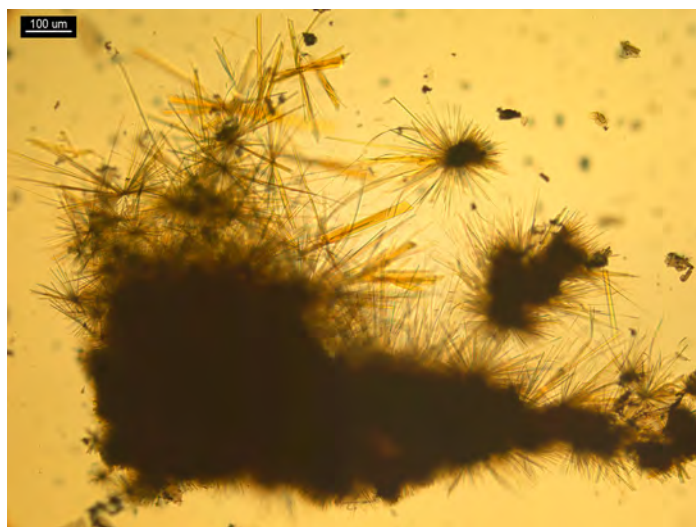
Figure 3. 1 PPP oxycodone in 5 \mu L of water and 5 \mu L of \text{H}_2\text{PtBr}_6 reagent. Crystals form yellow rosettes of elongated rods and needles.
