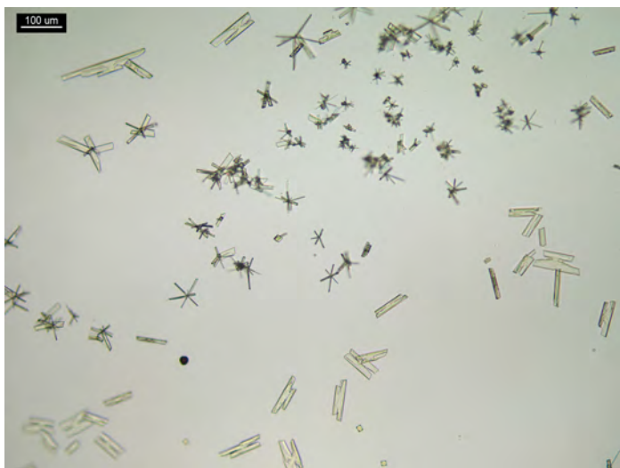
Figure 5. Direct test: 1 PPP of dl -methamphetamine and 5 μL of H 2 PtCl 6 reagent. Crystals form rods and stars.
