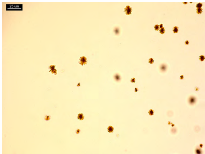
Figure 7. 5 μL from a morphine sulfate oral solution (20 mg/mL) and 10 μL of \text{HAuBr}_4 reagent form rosettes of blades.
