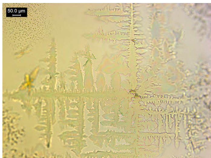
Figure 4. Volatility test: 2 PPP dl -amphetamine and one drop of 40% NaOH in a 5 μL hanging drop of H Au Cl 4 reagent, after 5 minutes the coverslip with the hanging drop was removed, inverted faceup and exposed to air. Crystals grow as branched, serrated plates.
