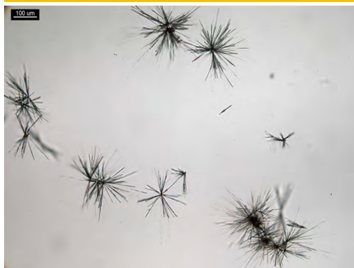
Figure 1. 5 PPP of morphine and 5 µL of HgCl 2 reagent form rosettes of needles.
