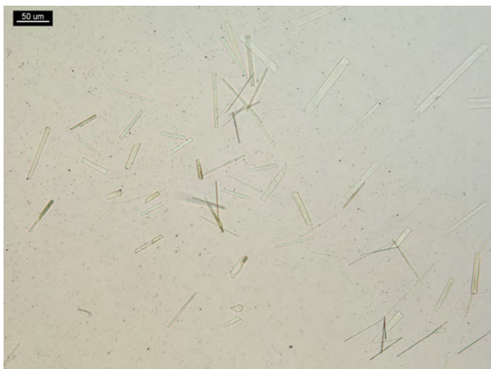
Figure 7. Direct test: 1 PPP of d -methamphetamine and 5–10 μL of H Au Cl 4 reagent. Crystals form rods.
