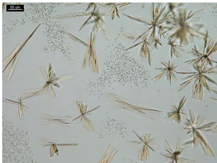
Figure 10. Paramethoxymethamphetamine:MDMA mixture (1:1) and 5–10 \mu\text{L} of \text{HAuCl}_4 and (1+2) \text{H}_3\text{PO}_4 reagent. Crystals are distorted, do not appear X-shaped, but are shaped like tablets and clusters.
