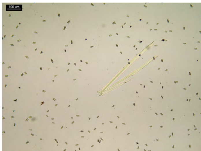
Figure 8. Direct test: 1 PPP of d -methamphetamine and 5–10 μL of H Au Cl 4 reagent. Large swallow tail- or clothespin-shaped crystals are surrounded by short rods.
