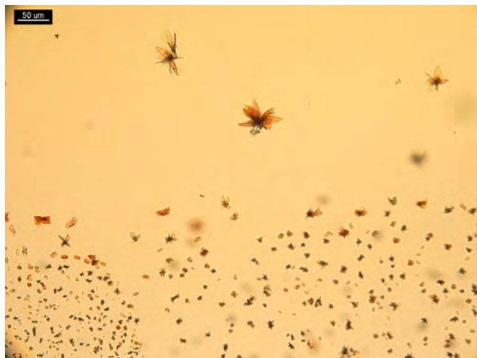
Figure 6. 2 PPP from a 30 mg morphine (extended release) pharmaceutical tablet and 10 μL of \text{HAuBr}_4 reagent form plates and rosettes of plates.
