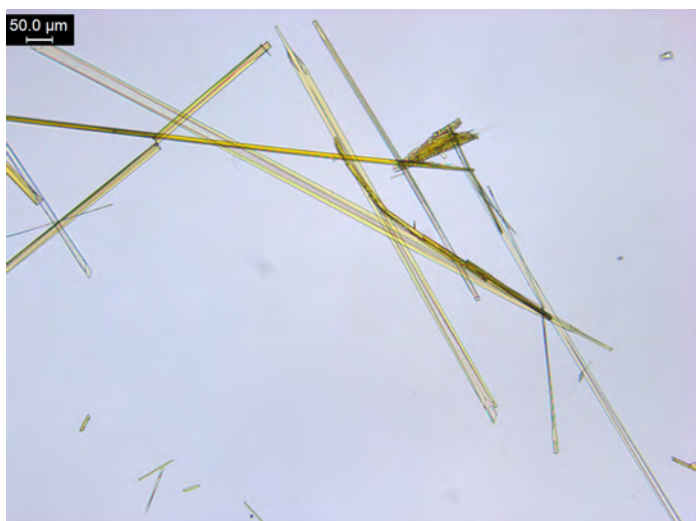
Figure 7. Volatility test: 2 PPP of d -amphetamine and one drop of 40% NaOH; crystals in a 5 μL hanging drop of HAuCl 4 reagent. Crystals form long yellow rods.
