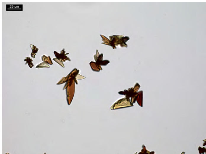
Figure 2. 1 PPP of codeine and 10 μL of reagent. Crystals form rosettes of triangles.
