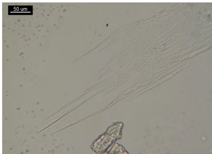
Figure 14. 1 PPP of insoluble material and 5 μL of \text{HAuCl}_4 reagent after chloroform extraction to remove guaifenesin from a Primatene® pharmaceutical tablet (12.5 mg ephedrine and 200 mg guaifenesin). Crystals form elongated plates that are stepped and jointed at 90°.
