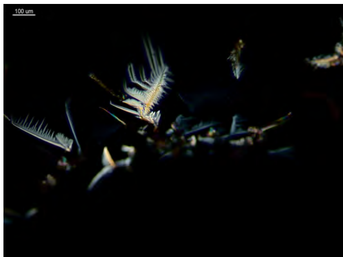
Figure 2. 1 PPP of cocaine in 5 μL 10% HCl and 5 μL of \text{H}_2\text{PtCl}_6 reagent. Crystals form feathery combs; crossed polars.
