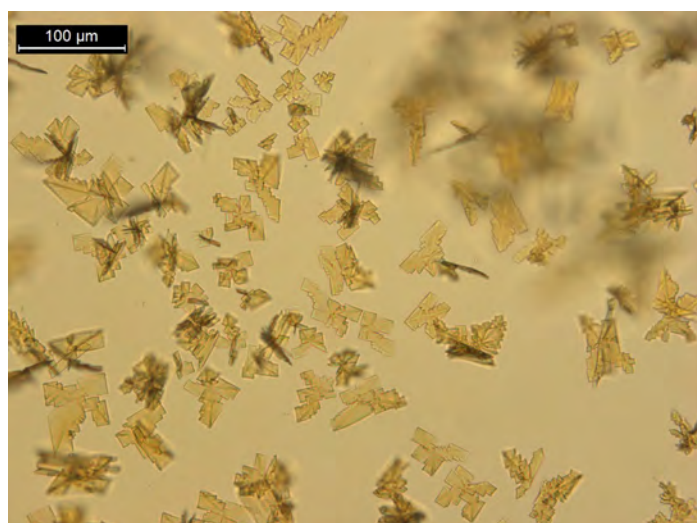
Figure 8. 1 PPP of BZP and 1 PPP TFMPP dissolved in 5 μL of H 2 O and 5 μL of H 2 PtBr 6 reagent. Crystals form rectangular and square plates, with some serrated X-shaped plates.
