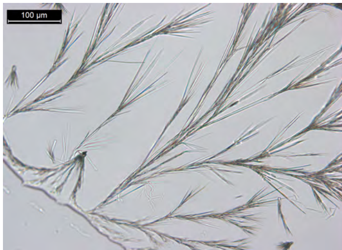
Figure 7. Quinine:heroin, 1:1 and 5 μL of HgI 2 and (27+73) HCl reagent. Crystals form straight-branched and forked dendrites, needles and branched paddles.
