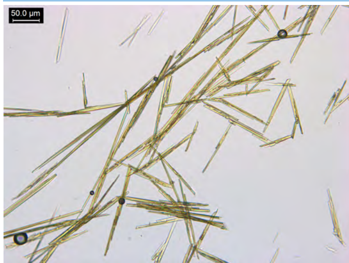
Figure 1. Volatility test: 2 PPP of d-amphetamine and one drop of 40% NaOH; crystals in a 5 µL hanging drop of HAuCl 4 reagent. Crystals form long yellow rods.
