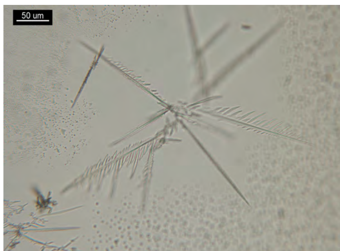
Figure 8. 1 PPP of Wal-itin® D pharmaceutical tablet (240 mg pseudoephedrine sulfate and 10 mg loratadine) and 5 μL of \text{HAuCl}_4 reagent. Crystals form branches and combs.
