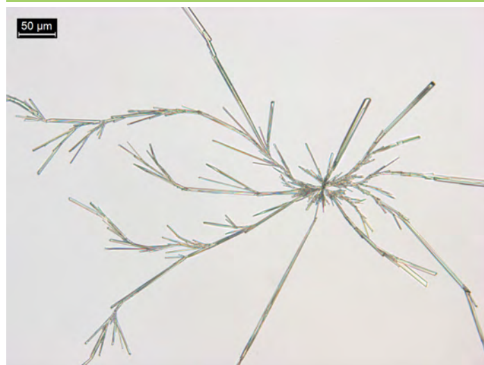
Figure 1. 1 PPP of diazepam dissolved in 5 µL of 1% HCl and 5 µL of NH 4 SCN reagent. Crystals form rosettes of thin and branched blades.
