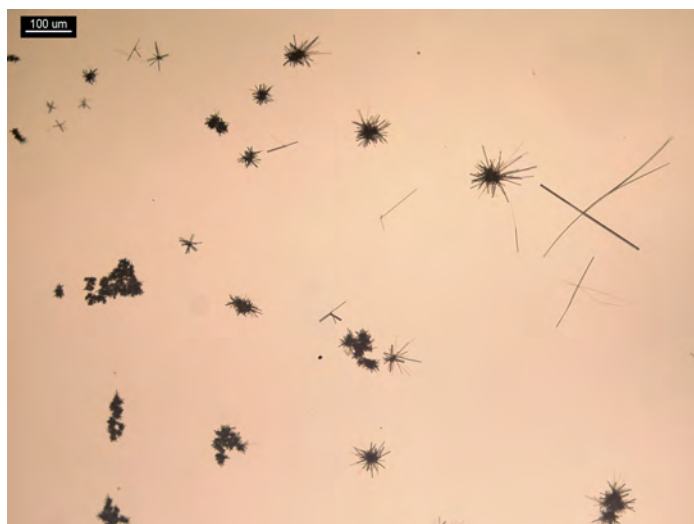
Figure 7. 10 μL from a methylphenidate oral solution (1 mg/mL) after chloroform extraction and 10 μL of lead iodide solution reagent. Results are inconclusive because rosettes of rods, rather than blades, formed.
