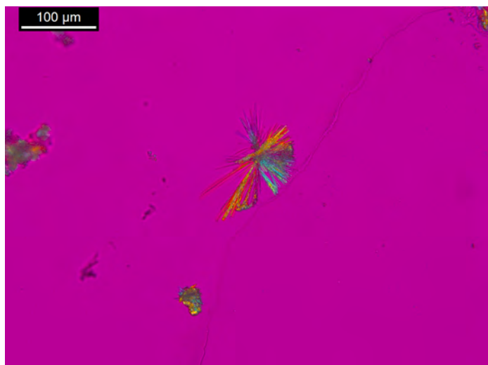
Figure 7. Same as Figure 6. Note negative sign of elongation; crossed polars and Red I compensator.
