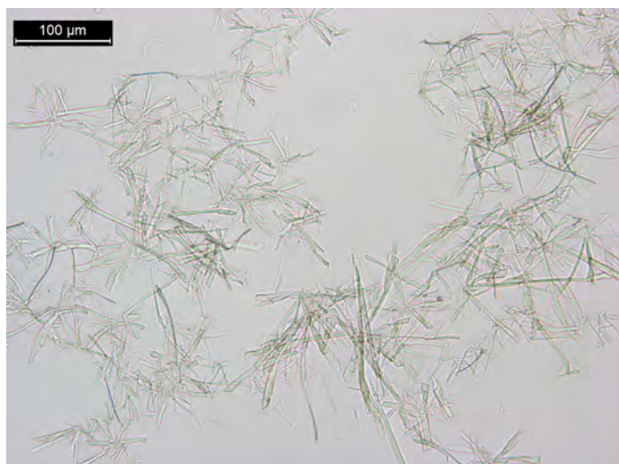
Figure 8. Volatility test: One drop of 40% NaOH added to 3 PPP of dl -amphetamine. Crystals formed in a 5 μL hanging drop of H 2 PtCl 6 reagent for 5 minutes. The coverslip with the hanging drop was removed from the reaction chamber and placed face-down onto the glass slide.
