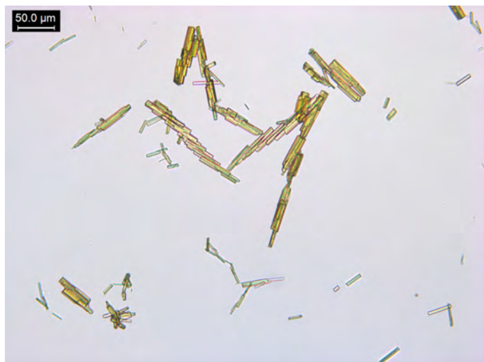
Figure 10. Volatility test: 2 PPP of d -amphetamine and one drop of 40% NaOH; crystals in a 5 μL hanging drop of H AuCl 4 reagent. Crystals form stacked and segmented long yellow rods.
