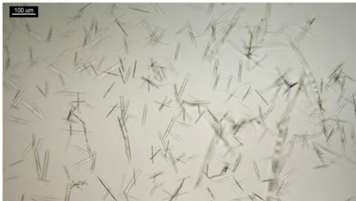
Figure 1. Direct test: 1 PPP of dl -methamphetamine and 5–10 µL of HAuCl 4 reagent. Rectangular rods with blunt or indented ends form instantly.
