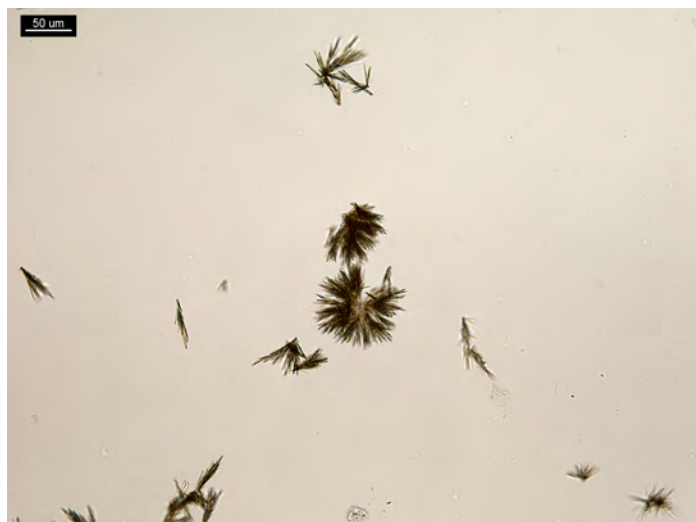
Figure 2. 1 PPP of hydrocodone in 5 μL of water and 5 μL of reagent mixture: \text{H}_2\text{PtBr}_6 , \text{HBr} , and (2+3) \text{H}_2\text{SO}_4 . Crystals form rosettes and broken rosettes.
