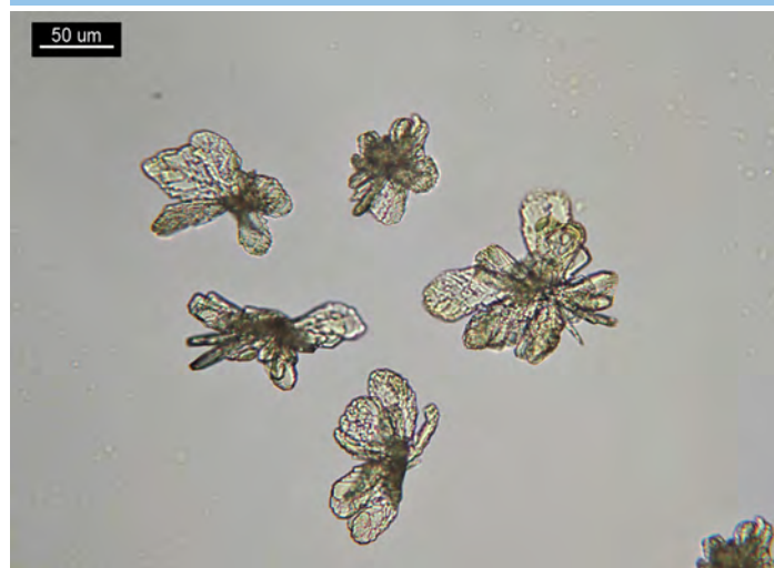
Figure 1. 1 PPP of methylphenidate and 10 \mu L of picric acid reagent. Crystals form rosettes of plates.
