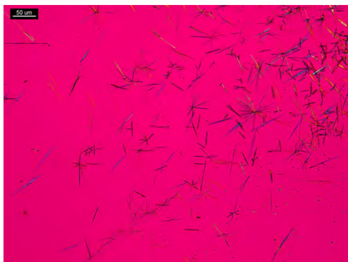
Figure 5. 1 PPP of clonazepam with 5–10 µL of H 2 PtCl 6 reagent; crossed polars and Red I compensator.
