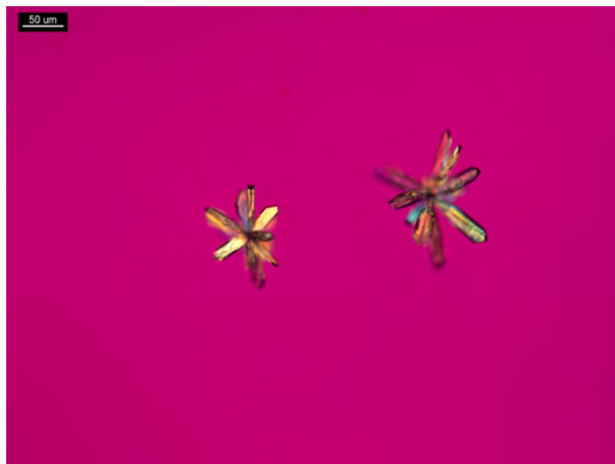
Figure 7. 1 PPP of sample dissolved in 5 μL of 20% HOAc and 5 μL of NH 4 SCN reagent. Crystals form rosettes of blades; crossed polars and Red I compensator.
