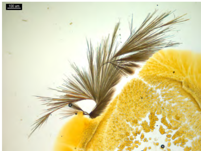
Figure 4. 1 PPP of hydromorphone and 10 μL of reagent mixture. Pleochroism observed on thicker needles: orange (parallel) to light yellow (perpendicular); microscope polarizer is oriented East-West.
