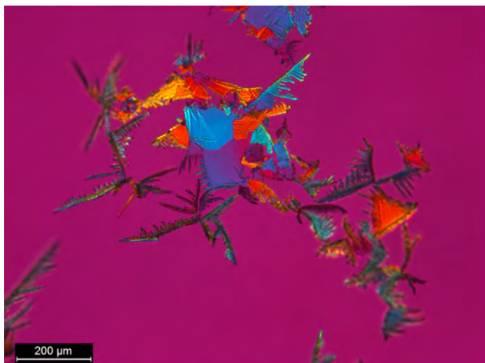
Figure 11. Procaine and cocaine (1:1) in 5 μL 10% HOAc and 5 μL of H 2 PtCl 6 reagent. Crystals form feathery combs; crossed polars and Red I compensator.
