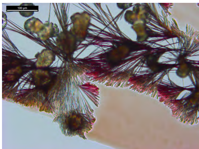
Figure 2. 2 PPP of psilocin after extraction and 2 μL of trinitrobenzoic acid reagent. Crystals form sheaves and fans of needles.
