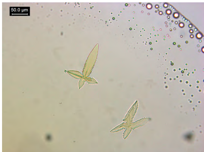
Figure 3. Volatility test: 2 PPP dl -amphetamine and one drop of 40% NaOH in a 5 μL hanging drop of H Au Cl 4 reagent.
