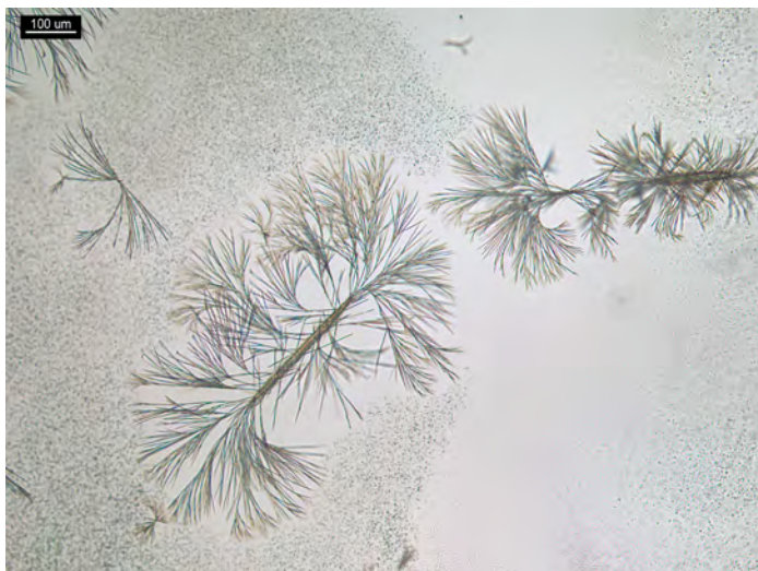
Figure 11. Strychnine:heroin, 1:1 in 5 μL of 1% HCl and 5 μL of HgCl 2 reagent. Crystal form distorted dendrites.
