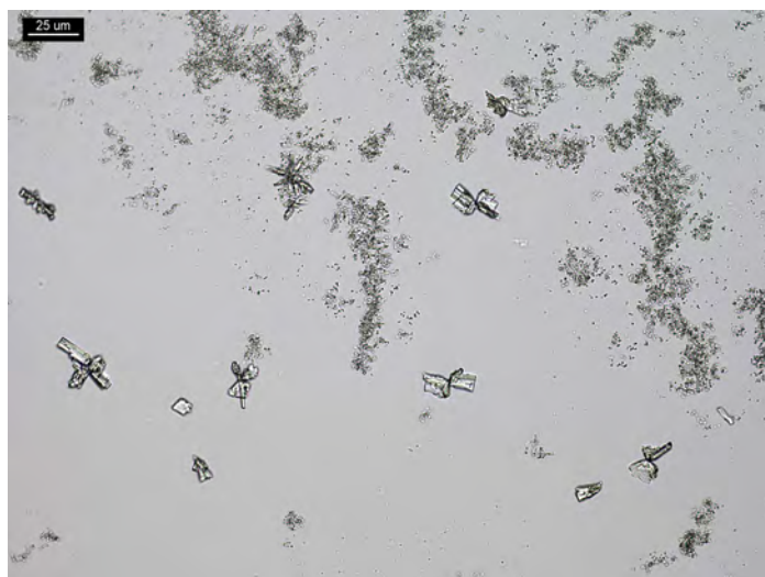
Figure 4. Phenergan oral solution (6.25 mg promethazine and 10 mg codeine) after an acid-base extraction in 5 \mu\text{L} of 1% HCl and 5 \mu\text{L} of reagent, with coverslip. Crystals form high-contrast, nearly equant tablets, prisms and rosettes.
