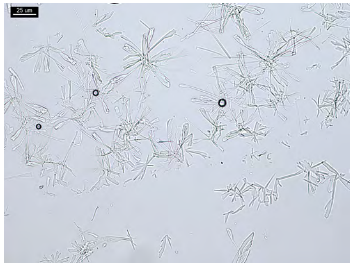
Figure 4. Volatility test: One drop of 40% NaOH added to 3 PPP of dl -amphetamine. Crystals formed in a 5 μL hanging drop of H 2 PtCl 6 reagent for 5 minutes. Then, the coverslip with the hanging drop was removed from the reaction chamber and placed facedown onto the glass slide.
