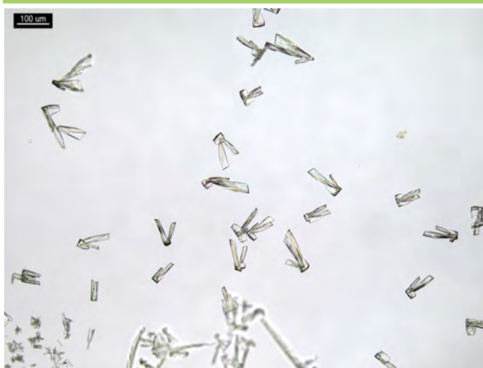
Figure 1. 1 PPP of cocaine in 5 \mu\text{L} 10% HCl and 5 \mu\text{L} of \text{H}_2\text{PtCl}_6 reagent. Crystals form K or V shapes.
