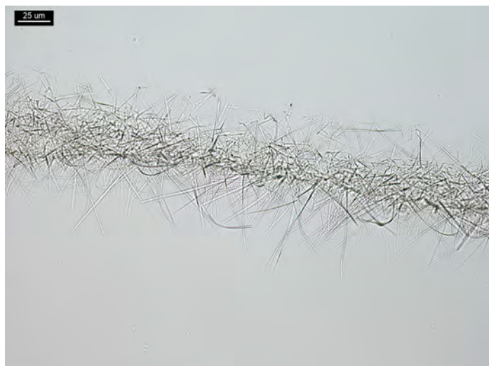
Figure 6. Volatility test: 2 PPP of d -amphetamine and one drop of 40% NaOH; crystals in a 5 µL hanging drop of H 2 PtCl 6 reagent. For this photomicrograph, the coverslip with the hanging drop was removed from the reaction chamber and placed drop-side down onto the glass slide.
