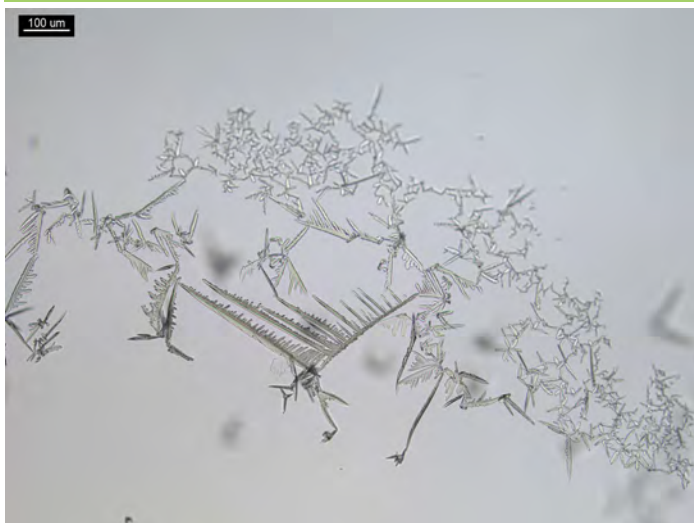
Figure 1. 1 PPP of cocaine in 5 \mu\text{L} 10% HOAc and 5 \mu\text{L} of \text{H}_2\text{PtCl}_6 reagent. Forms spiny, V-shaped crystals.
