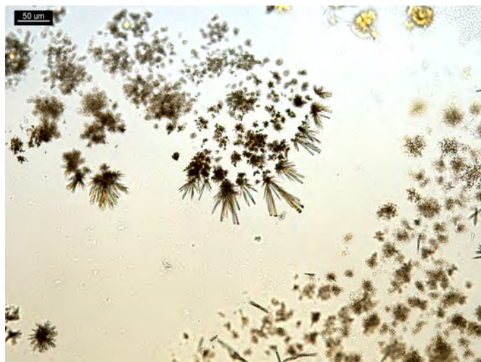
Figure 11. 10 mg hydrocodone and 325 mg acetaminophen tablet in 5 μL of water and 5 μL of reagent mixture, after extraction procedure. Clusters of yellow-brown precipitates form quickly and turn into rosettes of fine needles.
