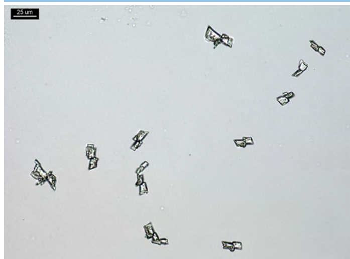
Figure 1. 1 PPP of codeine in 5 µL of 1% HCl and 5 µL of reagent, with coverslip. Crystals are equant tablets and prisms.
