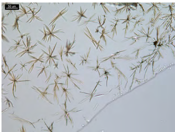
Figure 9. dl -Methamphetamine:MDMA mixture (1:1) and 5–10 μL of \text{HAuCl}_4 reagent. Crystals form star shapes and a few distorted X shapes.
