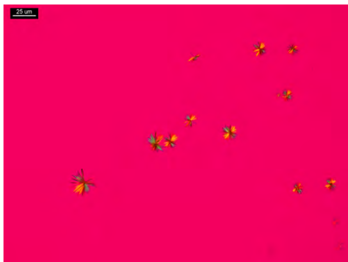
Figure 8. 5 μL from a morphine sulfate oral solution (20 mg/mL) and 10 μL of \text{HAuBr}_4 reagent form rosettes of blades with a negative sign of elongation; crossed polars and Red I compensator.
