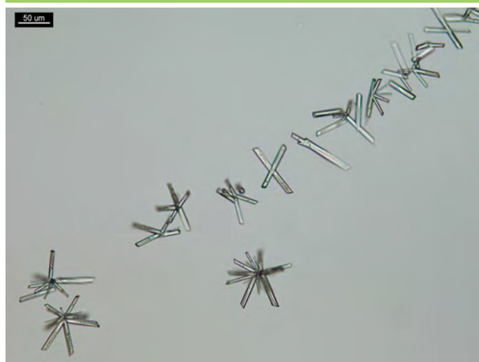
Figure 1. 1 PPP of hydromorphone and 5 \mu\text{L} of sodium nitroprusside reagent. Crystals form rods and elongated prisms, often in rosettes and stars.
