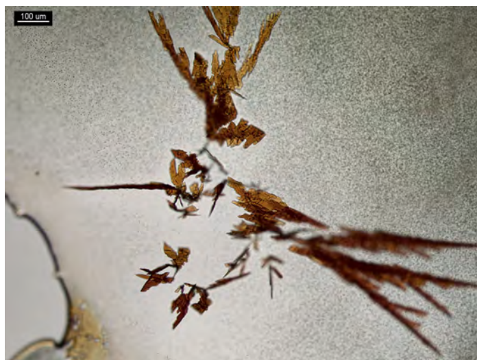
Figure 4. 3 PPP of morphine in 5 μL of water and 5 μL of Wagner's I-KI reagent. Crystals form clusters of irregular, feathery plates.
