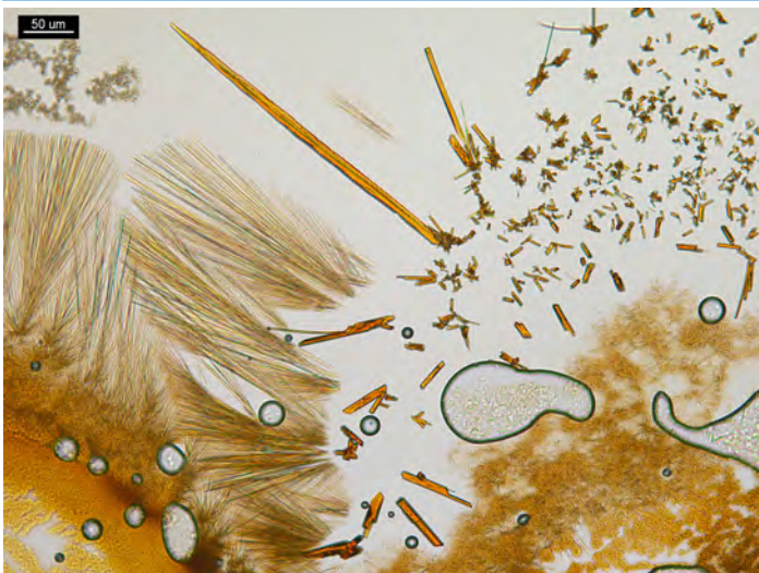
Figure 1. 1 PPP of oxycodone in 5 µL of water and 5 µL of H 2 PtBr 6 reagent. Crystals form rods and rosettes.
