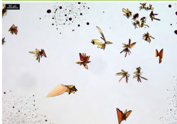
Figure 1. 1 PPP of codeine and 10 \mu L of reagent. Crystals form rosettes of triangles and hatchet blades.
