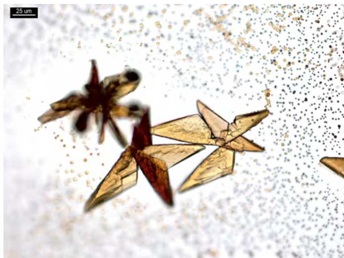
Figure 2. 1 PPP of codeine and 5 \mu\text{L} of reagent. Crystals form rusty red to yellow pleochroic rosettes of triangles; microscope polarizer is oriented East-West.
