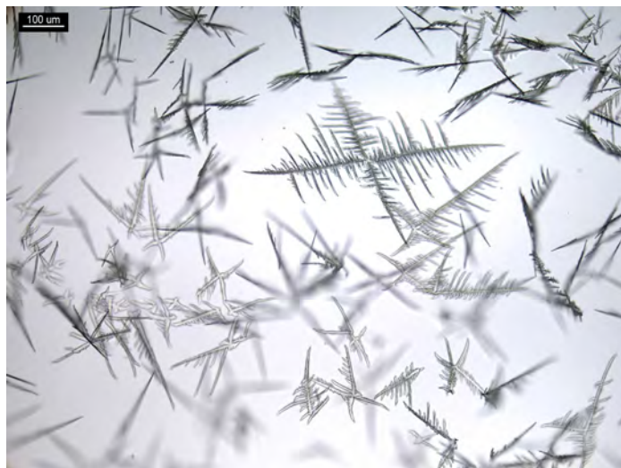
Figure 13. Direct test: 1 PPP from a street drug sample of methamphetamine with 5 μL of H 2 PtCl 6 and (1+3) H 3 PO 4 reagent. Crystals form dendrites and X shapes.
