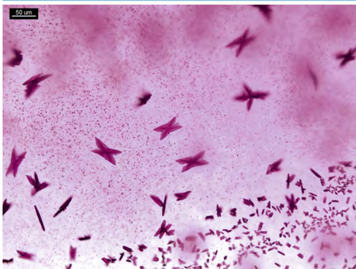
Figure 1. 1 PPP of PCP in 5 µL of 20% HOAc and 5 µL of KMnO 4 reagent. Crystals form bow ties, butterflies, rectangles, rods and X-shaped crystals.
