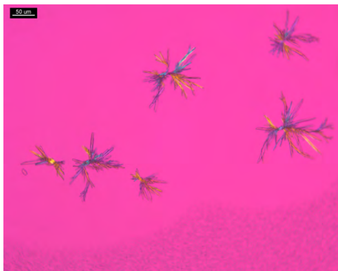
Figure 3. 1 PPP of methadone and 3 μL 2 N HOAc and 5 μL of HgCl 2 reagent (after ≈ 6 minutes). Crystals form fans and sheaves and dendrites; crossed polars and Red I compensator.
