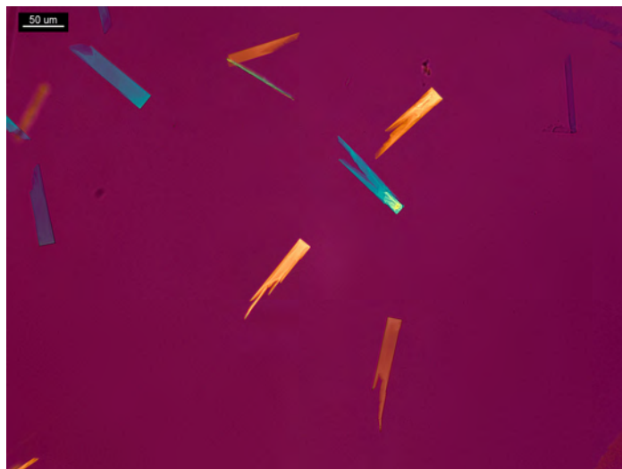
Figure 12. Direct test: 1 PPP from a street drug sample of ice (a pure form of methamphetamine) and 5–10 μL of H AuCl 4 reagent. Clothespins form instantly; crossed polars and Red I compensator.
