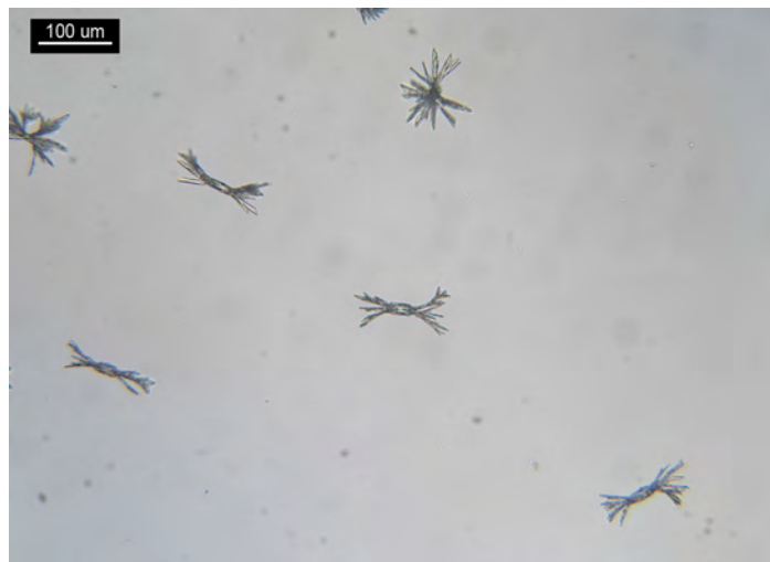
Figure 4. 1 PPP of methadone and 3 μL 2 N HOAc and 5 μL of HgCl 2 reagent; no coverslip. Crystals form rosettes and sheaves resembling wrapped candy.
