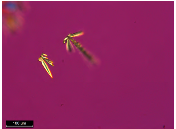
Figure 7. Levamisol and cocaine (1:1) in 5 μL 10% HOAc and 5 μL of \text{H}_2\text{PtCl}_6 reagent. Forms K-shaped crystals; crossed polars and Red I compensator.
