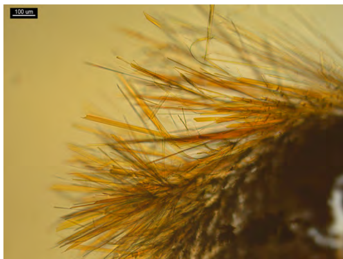
Figure 2. 1 PPP oxycodone in 5 \mu L of water and 5 \mu L of \text{H}_2\text{PtBr}_6 reagent. Crystals form yellow elongated rods.
