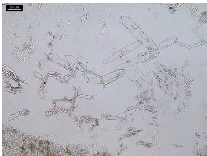
Figure 11. Sudafed® 12-hour pharmaceutical tablet (120 mg pseudoephedrine HCl and 220 mg naproxen sodium) and dilituric acid reagent after acid-base extraction. Crystals form elongated, six-sided tablets and plates.
