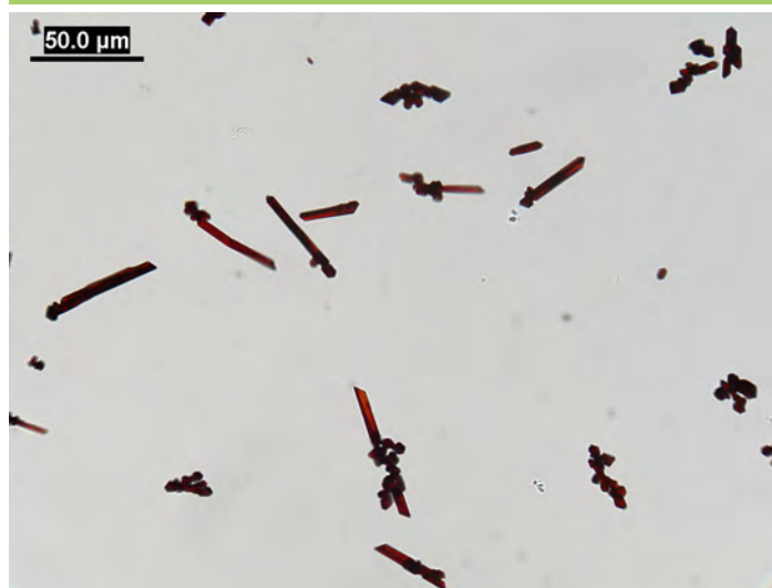
Figure 1. 1 PPP oxycodone in 5 µL of water and 5 µL of potassium tri-iodide reagent. Crystals form dark red rods and plates.
