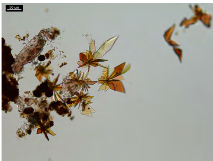
Figure 9. 8 PPP from a 30 mg codeine, 300 mg acetaminophen pharmaceutical tablet and 5 \mu\text{L} of reagent. Crystals form rosettes of angular plates and triangles. An acid-base extraction produced similar crystals.
