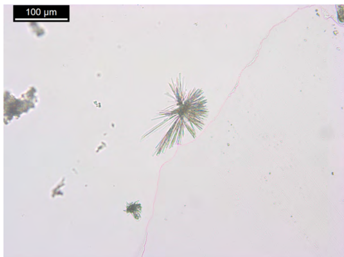
Figure 6. 3 PPP from a 100 mg pharmaceutical tablet and 5 μL of \text{HgCl}_2 reagent. Crystals form rosettes of needles.
