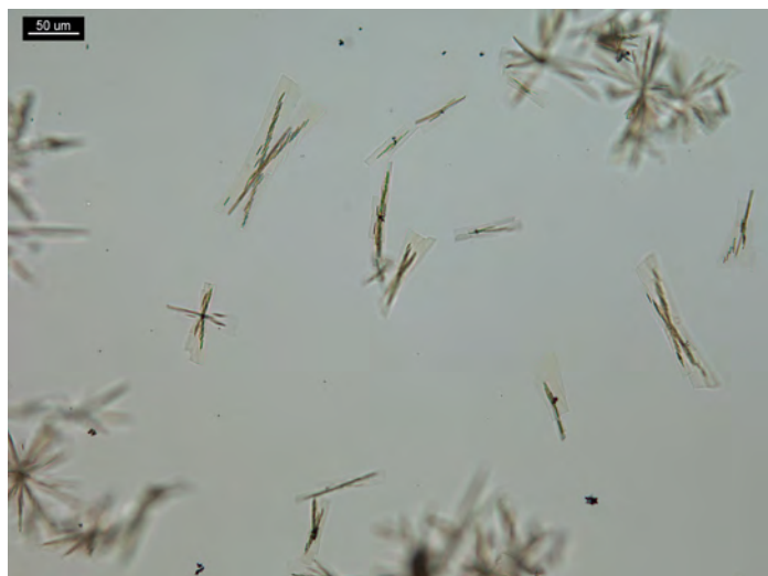
Figure 7. Dextromethorphan:MDMA mixture (5:1) and 5–10 μL of \text{HAuCl}_4 reagent. Crystals form X shapes with little or no distortion.
