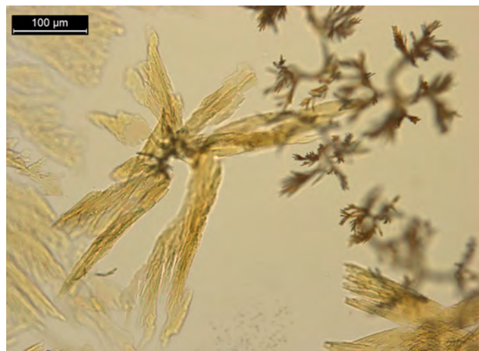
Figure 6. TFMPP only (no BZP) dissolved in 5 μL of H 2 O and 5 μL of H 2 PtBr 6 reagent. Crystals form rectangular laths and dendrites.
