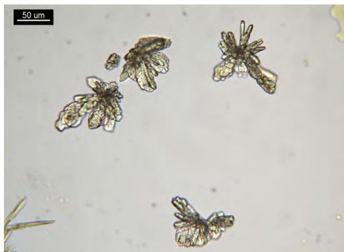
Figure 2. 1 PPP of methylphenidate and 10 μL of picric acid reagent. Crystals form sheaves, stars and dendrites.
