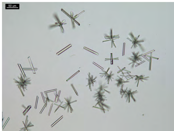
Figure 2. 1 PPP of hydromorphone and 5 µL of sodium nitroprusside reagent. Crystals form rods and elongated prisms, often in rosettes and stars.
