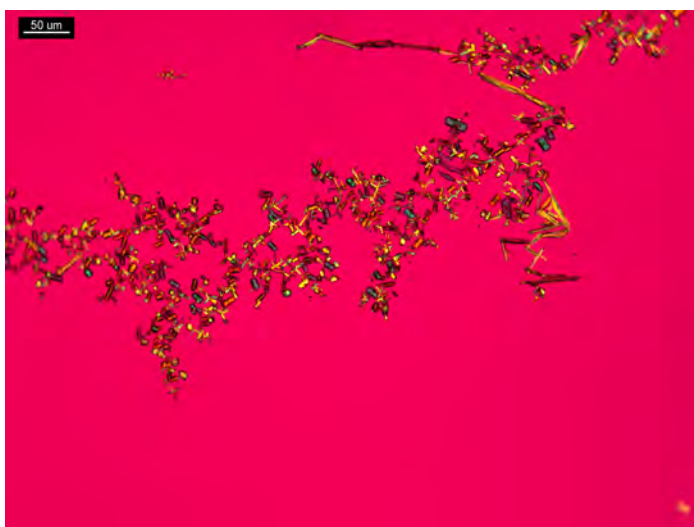
Figure 9. Volatility test: 1 PPP of dl -methamphetamine and 5 μL of H 2 PtCl 6 reagent. Rice grains and rods form in clusters. For this photomicrograph, the coverslip with the hanging drop was removed from the reaction chamber and placed facedown onto the glass slide; crossed polars and Red I compensator.
