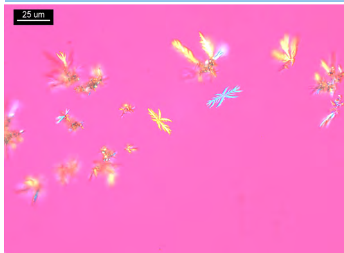
Figure 1. 1 PPP of cocaine in 5 µL of 10% HOAc and 5 µL of HAuCl 4 reagent. Crystals form X-shapes bisected by a barbed rod; crossed polars and Red I compensator.
