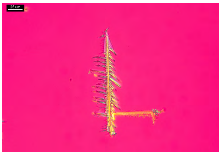
Figure 2. 3 PPP of cocaine in 5 μL of 10% HCl and 5 μL of \text{HAuCl}_4 reagent; crossed polars and Red I compensator. Note bright yellow interference colors when crystals are parallel to polars. Also, barbs on main rod are at oblique angles.
