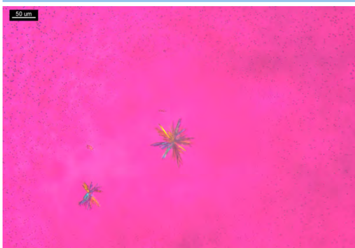
Figure 1. 1 PPP of methadone and 3 µL 2 N HOAc and 5 µL of HgCl 2 reagent. Crystals form rosettes and clusters in a hanging drop (after ≈ 4 minutes); crossed polars and Red I compensator.
