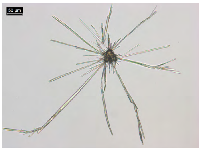
Figure 2. 1 PPP of diazepam dissolved in 5 μL of 1% HCl and 5 μL of \text{NH}_4\text{SCN} reagent. Crystals form rosettes of blades.
