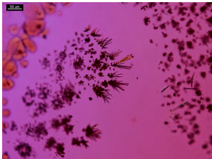
Figure 12. Same as Figure 11. Rosettes of fine needles have a negative sign of elongation; crossed polars and Red I compensator.
