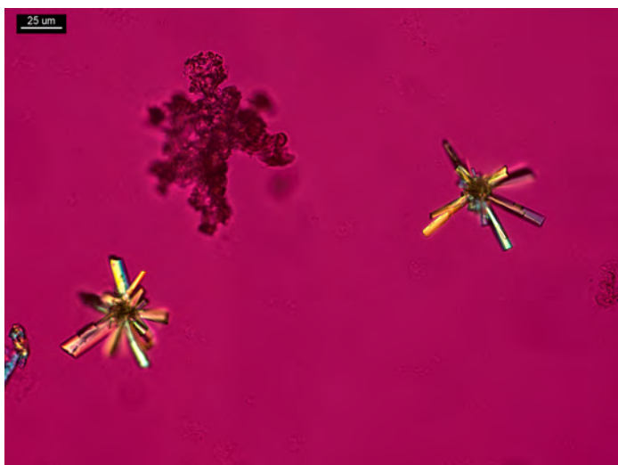
Figure 3. 5 PPP from a 300 mg acetaminophen and 30 mg codeine tablet in 5 \mu\text{L} of 1% HCl and 5 \mu\text{L} of reagent, with coverslip. Crystals form high-contrast, elongated prisms and rosettes are visible; crossed polars and Red I compensator.
