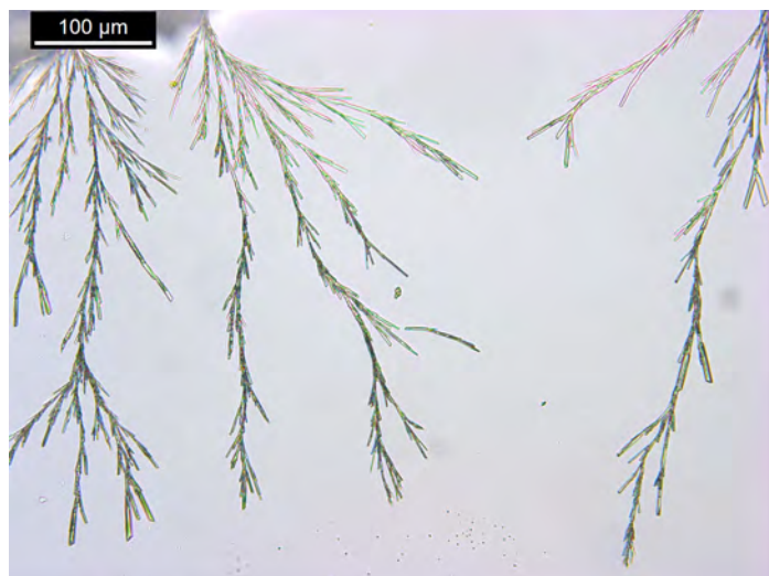
Figure 6. Rectal gel containing 2.5 mg/0.5 mL of diazepam and 5 μL of 1% HCl and 5 μL of \text{NH}_4\text{SCN} reagent, after chloroform extraction. Crystals form branched blades.
