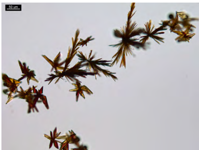
Figure 7. 1 PPP of codeine and 5 \mu\text{L} of reagent. Crystals form rosettes of triangles and rods.
