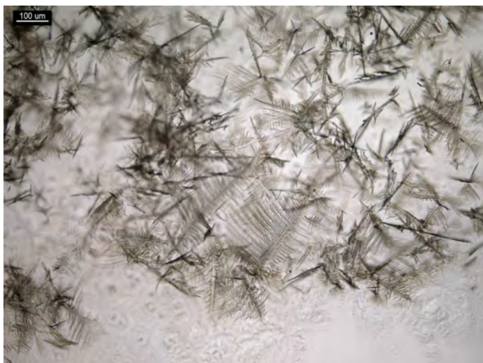
Figure 3. 1 PPP of of d -methamphetamine with 5 μL of H 2 PtCl 6 reagent. Crystals form dendrites and X-shaped.
