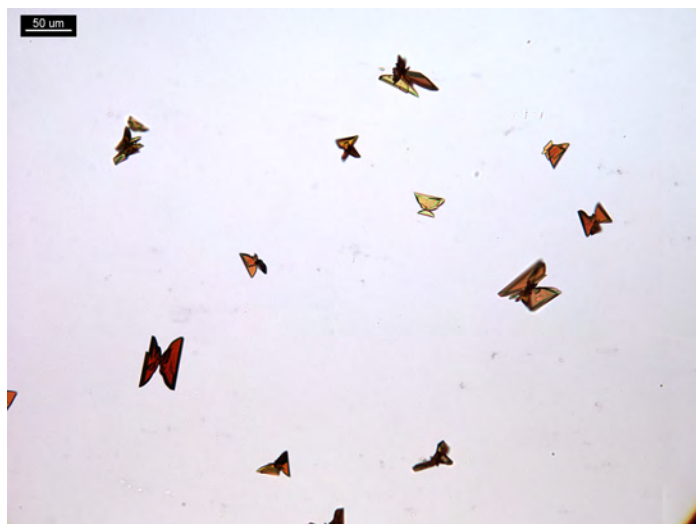
Figure 6. 1 PPP of codeine and 10 μL of reagent. Crystals form hourglass- and semicircle-shaped crystals.
