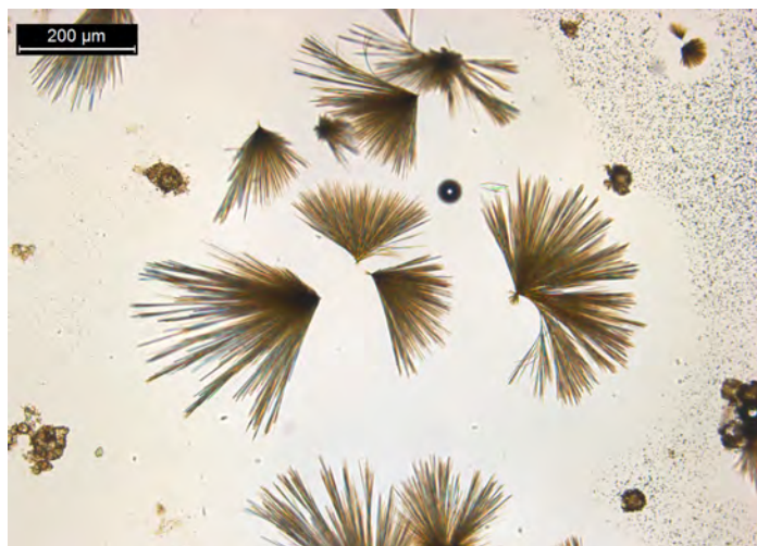
Figure 8. 1 PPP of hydromorphone and 10 µL of reagent mixture. Crystals form fans, rosettes and needles.
