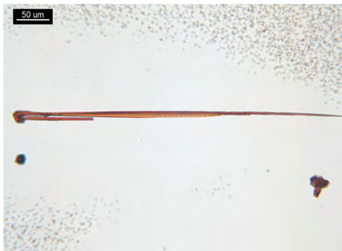
Figure 6. Same crystal as Figure 4. Microscope polarizer is oriented East-West. Note pleochroic dark red-orange color.
