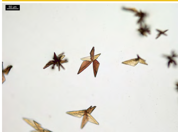
Figure 1. 1 PPP of codeine and 5 µL of reagent. Amorphous grains precede crystal formation. Crystals form triangles and rosettes of triangles.
