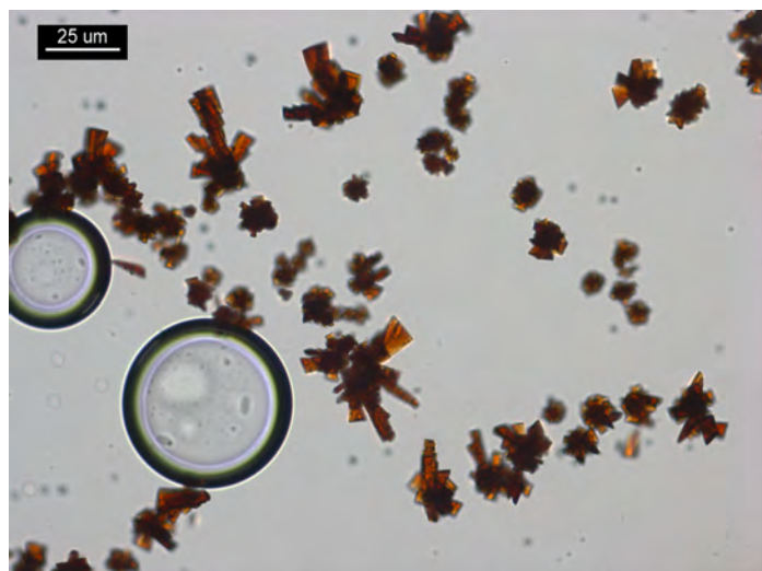
Figure 2. 1 PPP of morphine and 10 \mu\text{L} of \text{HAuBr}_4 reagent. Crystals form clusters and rosettes of plates. Pleochroism on plates: red to orange; East-West polarizer.
