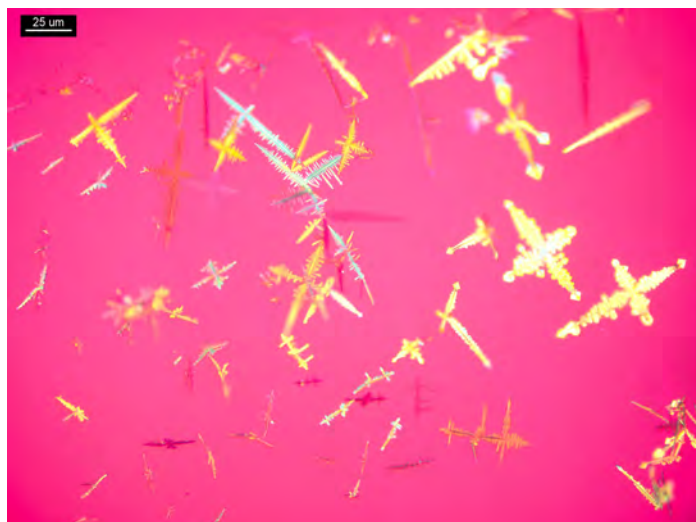
Figure 2. 3 PPP of cocaine in 5 μL of 10% HOAc and 5 μL of H AuCl 4 reagent. Crystals form combs and crosses; crossed polars and Red I compensator.
