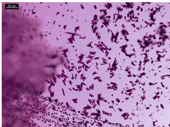
Figure 2. 1 PPP of PCP in 5 μL of 20% HOAc and 5 μL of \text{KMnO}_4 reagent. Crystals form bow ties and rectangles.
