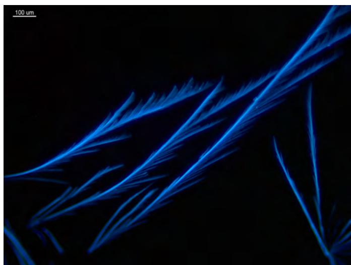
Figure 11. 2 PPP of heroin and 5 \mu\text{L} of \text{HgI}_2 and (27+73) HCl reagent. Anomalous first-order gray interference colors appear blue; crossed polars.
