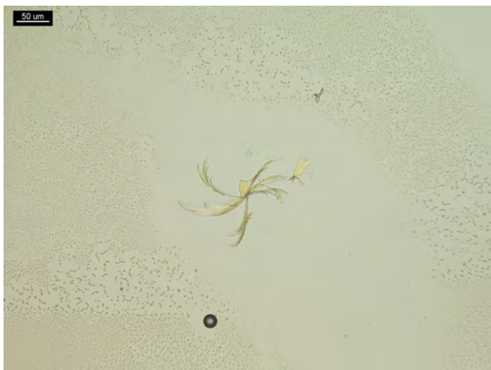
Figure 9. 10 μL from a methylphenidate oral solution (1 mg/mL) after chloroform extraction and 10 μL of picric acid reagent. Crystals form pinwheel shapes.
