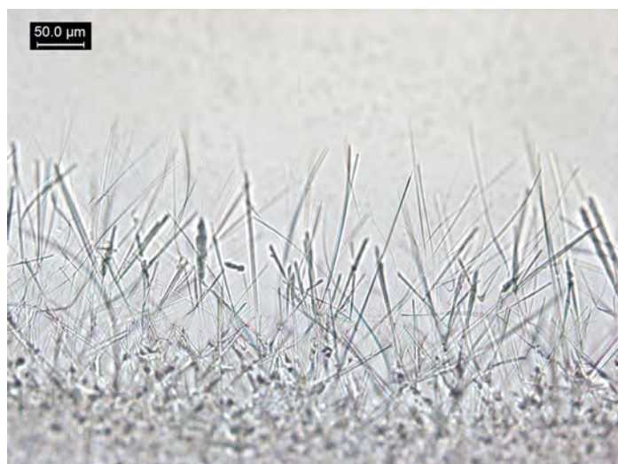
Figure 4. Volatility test: 2 PPP of d -amphetamine and one drop of 40% NaOH; crystals in a 5 μL hanging drop of H 2 PtCl 6 reagent. Crystals grow from a crust that forms at the edge of the hanging drop.
