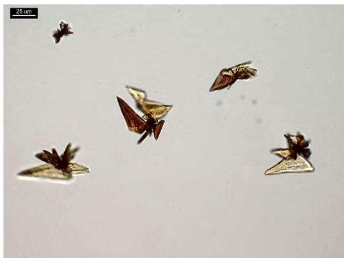
Figure 4. 1 PPP of codeine and 10 μL of reagent. Crystals form rusty red/orange to yellow pleochroic rosettes of triangles; microscope polarizer is oriented East-West.
