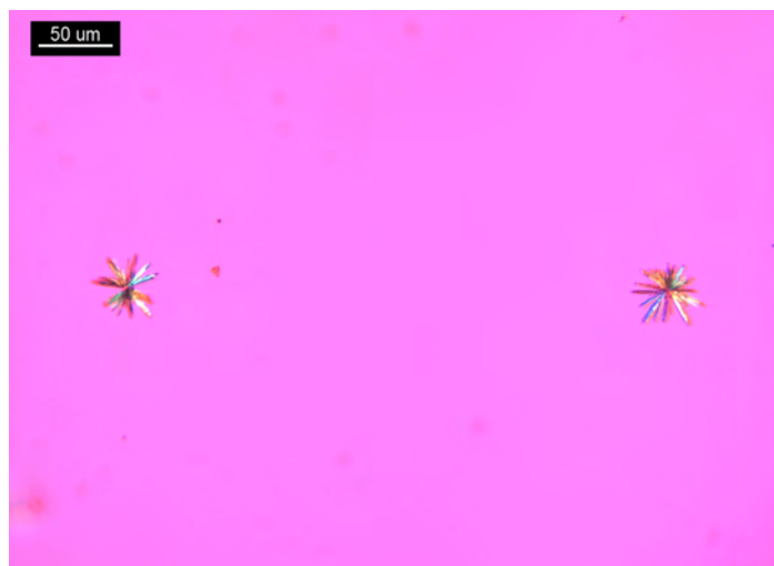
Figure 6. 10 μL from a methadone hydrochloride oral solution (5 mg/5 mL) and 5 μL of HgCl 2 reagent (after ≈ 3 minutes). No extraction was necessary. Crystals form rosettes; crossed polars and Red I compensator.
