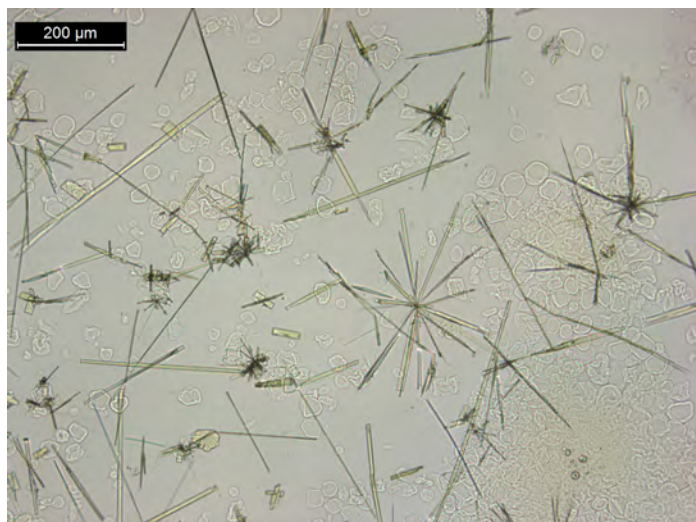
Figure 15. Direct test: One pill from a 10 mg Dexedrine® capsule was crushed and gently stirred with 10 μL of HAuCl 4 reagent. Crystals form long yellow rods.
