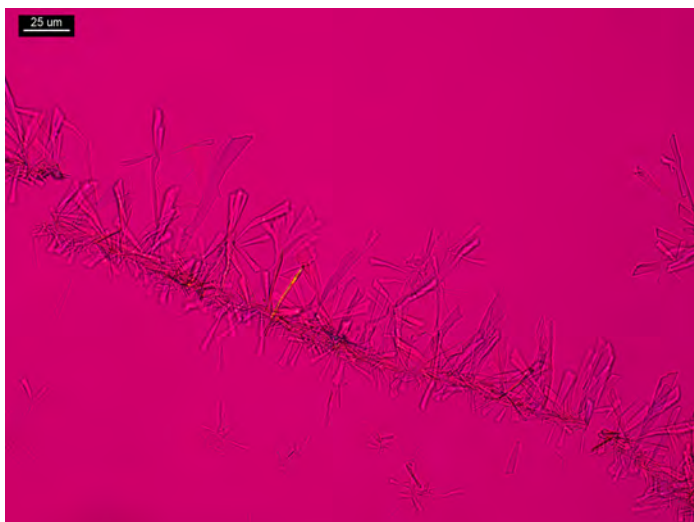
Figure 11. Volatility test: One drop of 40% NaOH added to 3 PPP of dl -amphetamine. Crystals formed in a 5 μL hanging drop of H 2 PtCl 6 reagent; crossed polars and Red I compensator.
