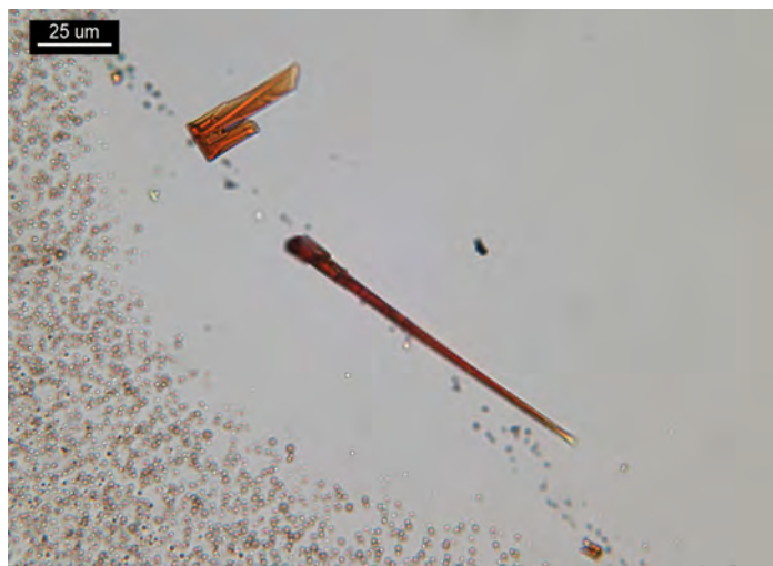
Figure 12. 1 PPP of insoluble material from a Bronkaid® (25 mg ephedrine sulfate and 400 mg guaifenesin) pharmaceutical tablet, after chloroform extraction to remove guaifenesin, and 10 \mu L of the \text{HAuBr}_4 reagent. Nail-shaped crystals formed within 15 minutes.
