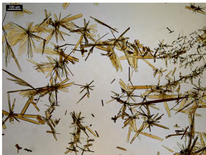
Figure 9. 1 PPP of acetaminophen (no hydrocodone) in 5 μL of water and 5 μL of reagent mixture: \text{H}_2\text{PtBr}_6 , \text{HBr} , and (2+3) \text{H}_2\text{SO}_4 . Crystals form yellow blades and sheaves.
