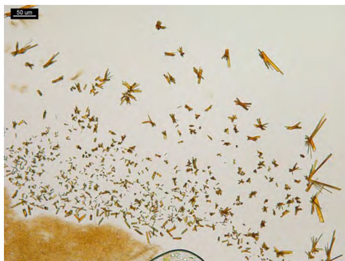
Figure 4. 1 PPP oxycodone in 5 \mu L of water and 5 \mu L of \text{H}_2\text{PtBr}_6 reagent. Crystals form rods and blades.
