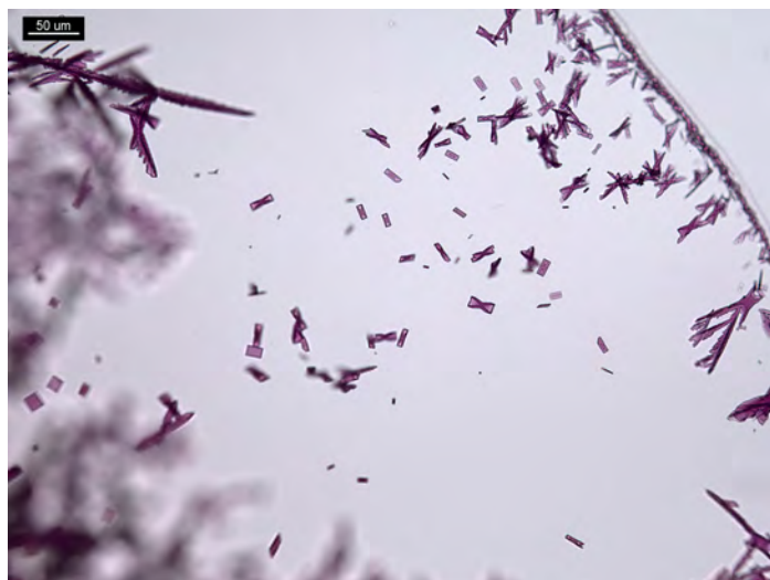
Figure 4. 1 PPP of PCP in 5 μL of 20% HOAc and 5 μL of \text{KMnO}_4 reagent. Crystals form bow ties and elongated rods.
