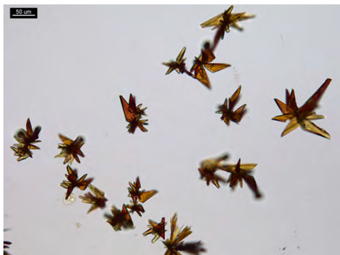
Figure 6. 1 PPP of codeine and 5 \mu\text{L} of reagent. Crystals form rosettes of triangles and rods.
