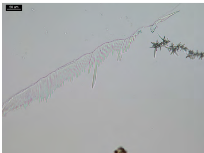
Figure 5. 1 PPP of hydromorphone and 5 µL of sodium nitroprusside reagent. Feather-shaped and serrated crystals formed initially near the edge of the test drop. Note: If pushed back into the center of the drop with a glass rod, toothpick or pipette tip, these crystals dissolve and recrystallize as typical rods and elongated prisms.
