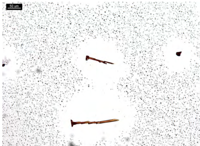
Figure 2. 1 PPP of L -ephedrine and 10 µL of the HAuBr 4 reagent. Crystals are nail-shaped.
