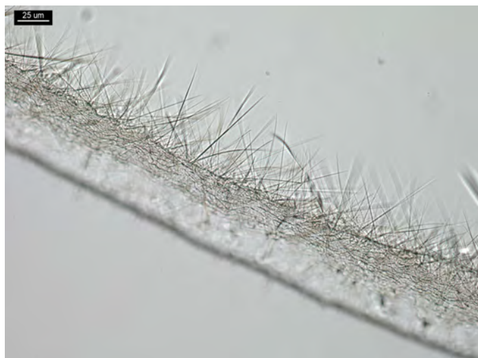
Figure 2. Volatility test: 2 PPP of d -amphetamine and one drop of 40% NaOH; crystals in a 5 μL hanging drop of H 2 PtCl 6 reagent. Crystals grow from a crust that forms at the edge of the hanging drop.
