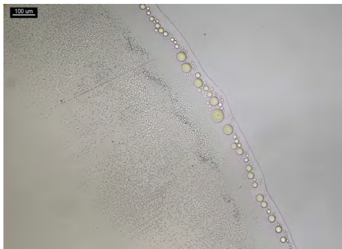
Figure 2. 1 PPP of L -ephedrine and 5 μL of H[AuCl 4 ] reagent. Oily drops form immediately after adding the reagent.
