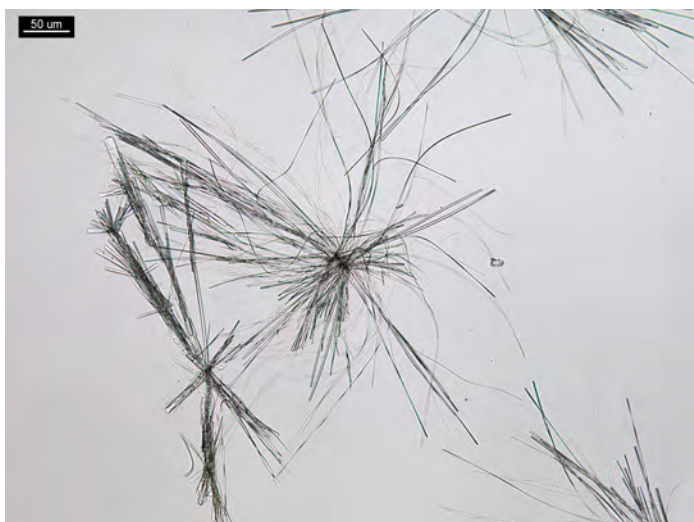
Figure 3. 5 PPP of morphine and 5 μL of HgCl 2 reagent form rosettes of needles; with coverslip.
