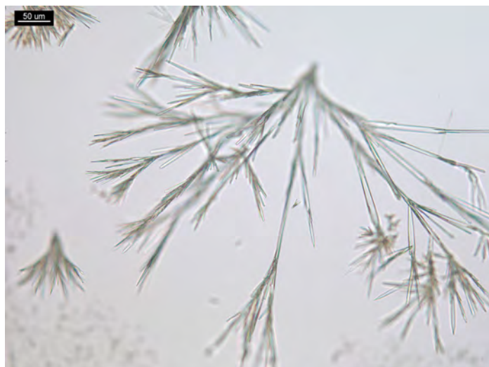
Figure 9. Strychnine:heroin, 1:1 and 5 \mu\text{L} of \text{HgI}_2 and (27+73) HCl reagent. Crystals form straight-branched and forked dendrites, needles and branched paddles.
