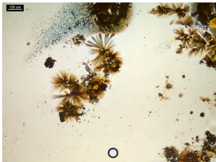
Figure 2. 1 PPP of hydromorphone and 10 μL of reagent mixture. Crystals form rosettes, sheaves, fans and needles.
