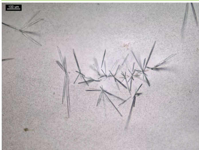
Figure 1. 2 PPP of sample dissolved in 5 µL of 20% HOAc and 5 µL of NH 4 SCN reagent. Crystals form blades and rosettes of blades.
