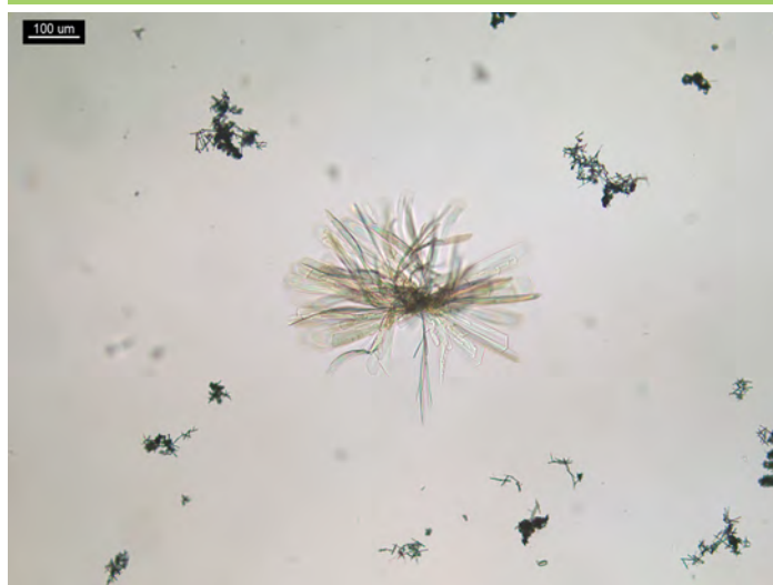
Figure 1. 3 PPP of methylphenidate and 10 µL of lead iodide solution reagent. Crystals form large rosettes of blades and clusters.
