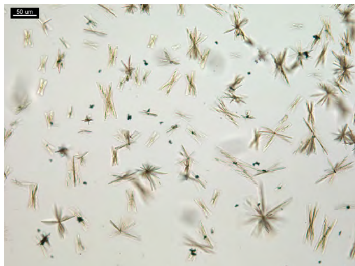
Figure 11. Paramethoxyamphetamine:MDMA (5:1) and 5–10 \mu\text{L} of \text{HAuCl}_4 and (1+2) \text{H}_3\text{PO}_4 reagent. X-shaped crystals, tablets and clusters. The X-shaped crystals are shorter and wider than MDMA-gold chloride crystals.
