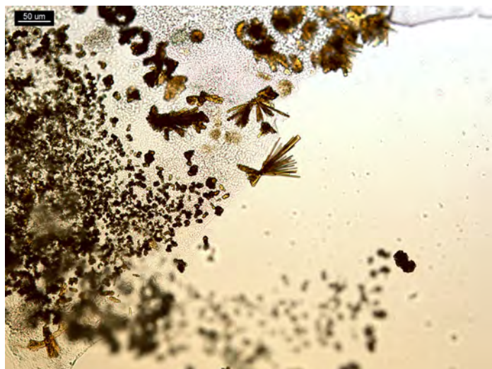
Figure 14. 5 mg hydrocodone and 500 mg acetaminophen tablet in 5 \mu L of water and 5 \mu L of reagent mixture, after extraction procedure. Clusters of yellow-brown precipitates form quickly and turn into rosettes of fine needles.
