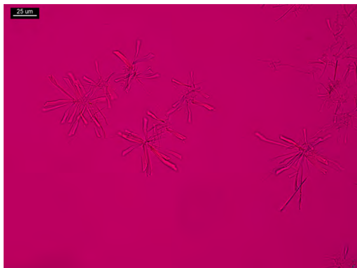
Figure 10. Volatility test: One drop of 40% NaOH added to 3 PPP of dl -amphetamine. Crystals formed in a 5 μL hanging drop of H 2 PtCl 6 reagent. Crystals have very low birefringence; crossed polars and Red I compensator.
