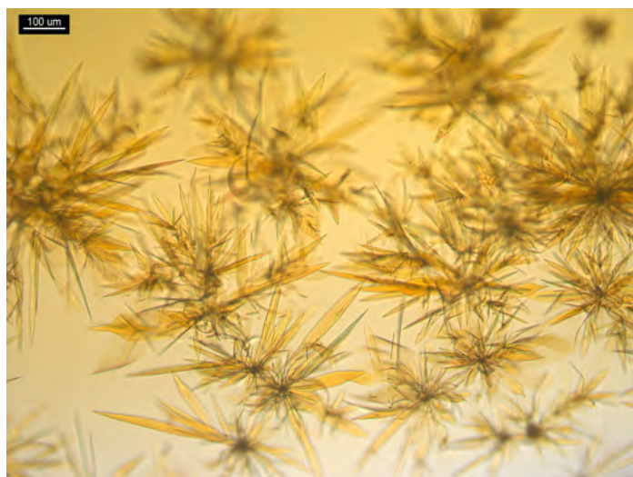
Figure 8. 2.5 μL from a 20 mg/mL oxycodone oral solution in 2.5 μL of water and 5 μL of \text{H}_2\text{PtBr}_6 reagent. Crystals form rosettes of blades.
