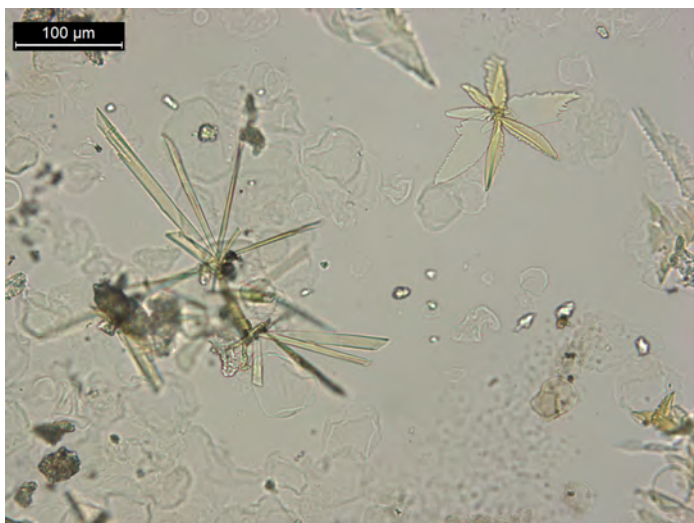
Figure 9. Direct test: 5 PPP from a 10 mg tablet crushed and gently stirred with 10 μL of \text{HAuCl}_4 reagent. This test detected d -amphetamine (long yellow rods, left) and dl -amphetamine (serrated plates, upper right).
