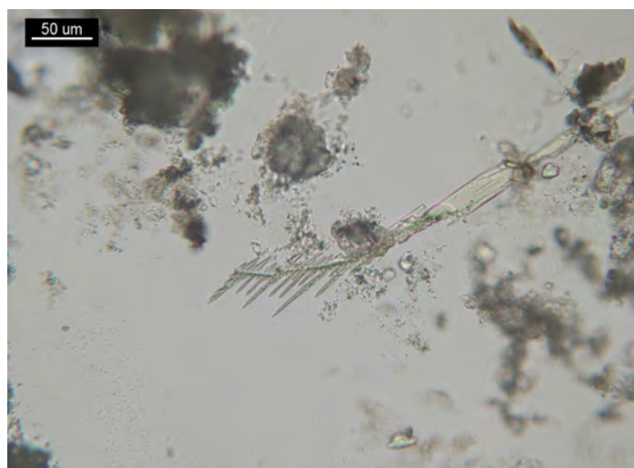
Figure 9. A small portion from a children's pseudoephedrine chewable tablet (15 mg pseudoephedrine) after a chloroform extraction and 5 μL of \text{HAuCl}_4 reagent. Crystals form branches and combs.
