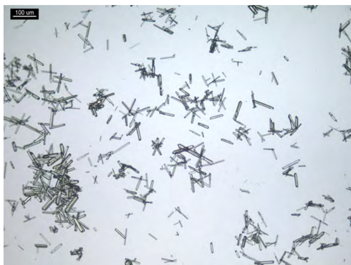
Figure 9. 3 PPP of tramadol and 10 μL of lead iodide solution reagent. Crystals form rods and stars of rods, which are distinguishable from methylphenidate.
