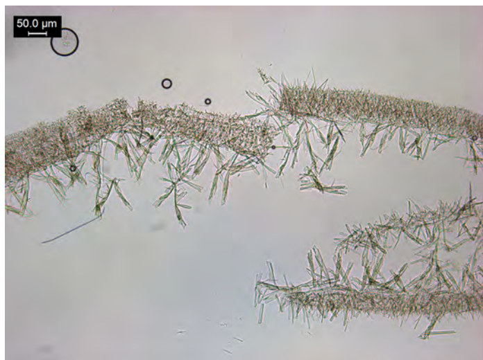
Figure 7. Volatility test: One drop of 40% NaOH added to 3 PPP of dl -amphetamine. Crystals formed in a 5 μL hanging drop of H 2 PtCl 6 reagent. Crystals grow from a crust that forms at the edge of the hanging drop. The coverslip with the hanging drop was removed from the reaction chamber and placed facedown onto the glass slide.
