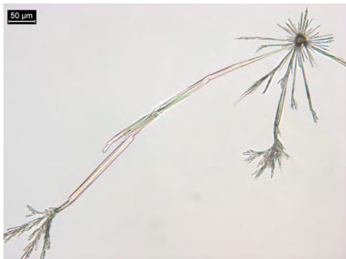
Figure 4. 1 PPP of diazepam dissolved in 5 μL of 1% HCl and 5 μL of \text{NH}_4\text{SCN} reagent. Crystals form rosettes of blades.
