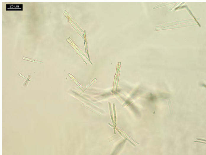
Figure 1. Direct test: 1 PPP of d -methamphetamine with 5-10 µL of HAuCl 4 reagent. Clothespins, forked rods and swallow tails form instantly.
