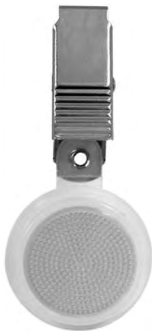
FIGURE 6.3.1.3 Passive Sampling Badge. The passive sampling badge contains a sorbent or a filter coated with a specific reactant that traps the contaminant(s) in the air. Passive monitors work by diffusion of the contaminant from the surrounding environment into the sorbent and the determination of the average air concentration is determined by validation testing. (Courtesy of SKC, Inc., Eighty Four, PA.)
