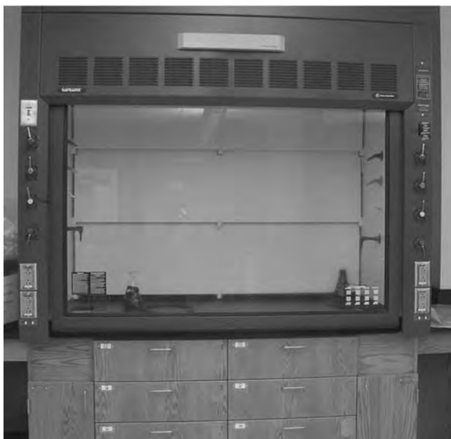
FIGURE 7.1.4.1 Laboratory Hood with a Vertical Sash. Sashes should always be closed except when arms and hands need to be accessing something inside the chemical hood. This both saves energy (for many modern hoods) and provides a shield against explosions and fires.
