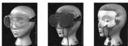
FIGURE 7.1.2.1 Degrees of Eye Protection from Simulated Splashes Using Varied Types of Eye Protection. The mannequin faces on the right show how effective each type of eye protection is against a chemical splash. Only the chemical splash goggles provide adequate protection and are the only acceptable form of eye protection in chemistry laboratories. (Courtesy of Linda Stroud, Ph.D., Science & Safety Consulting Services. Copyright © 2008 Science & Safety Consulting Services, Inc., Raleigh, NC.)
