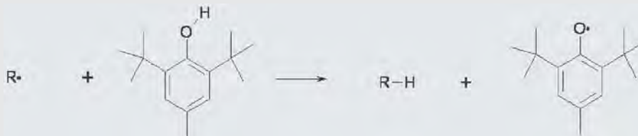
FIGURE 5.3.2.3 BHT Radical Reaction. BHT scavenges alkyl radicals, and the BHT radical is very stable and unreactive.
