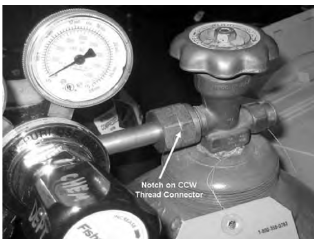
FIGURE 5.3.1.3 Notch in Connecting Nut Indicating CCW Thread. For most normal gases the CGA connector attaches clockwise (CW), but for flammable gases the CGA connector attaches counterclockwise (CCW).
