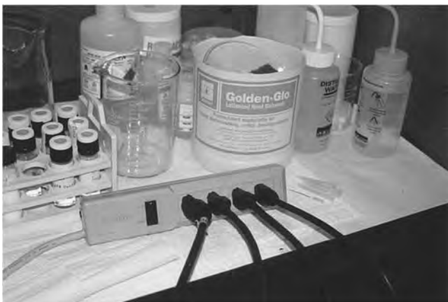
FIGURE 5.3.5.2 Outlet in Chemical Hood. A strip outlet in a chemical hood represents a fire hazard since the outlets and switch are not spark-proof and flammable chemicals are often used in hoods. The dangling cords might also present a trip hazard. A liquid spill could also present a shock hazard. (From Journal of Chemical Health and Safety 7(5): 6 (2000). Used with permission. Copyright © 2000 Division of Chemical Safety and Health of the American Chemical Society.)
