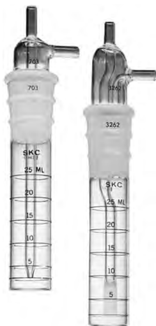
FIGURE 6.3.1.2 An Impinger for Air Sampling. The bottom portion of the impinger is filled with a measured quantity of a liquid. The air sample is drawn into the liquid from the opening at the top by using reduced pressure at the side port. The impinger on the right has a sintered glass attachment at the bottom, which creates many small bubbles in the air and optimizes the air–liquid interface. (Courtesy of SKC, Inc., Eighty Four, PA.)
