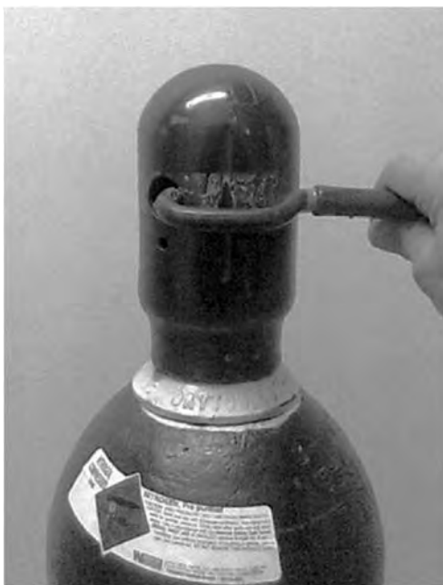
FIGURE 5.3.1.4 Tool to Remove Cylinder Cap. Do not try to force a stuck cylinder cap with a long screwdriver or other tool that goes through the cap. This may inadvertently open the tank by moving the main tank valve.
