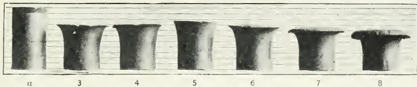
A. RESULTS OF SMALL LEAD BLOCK TESTS OF P. T. S. S. ELECTRIC DETONATORS NOS. 3, 4, 5, 6, 7, AND 8. a , BLOCK BEFORE TEST.
