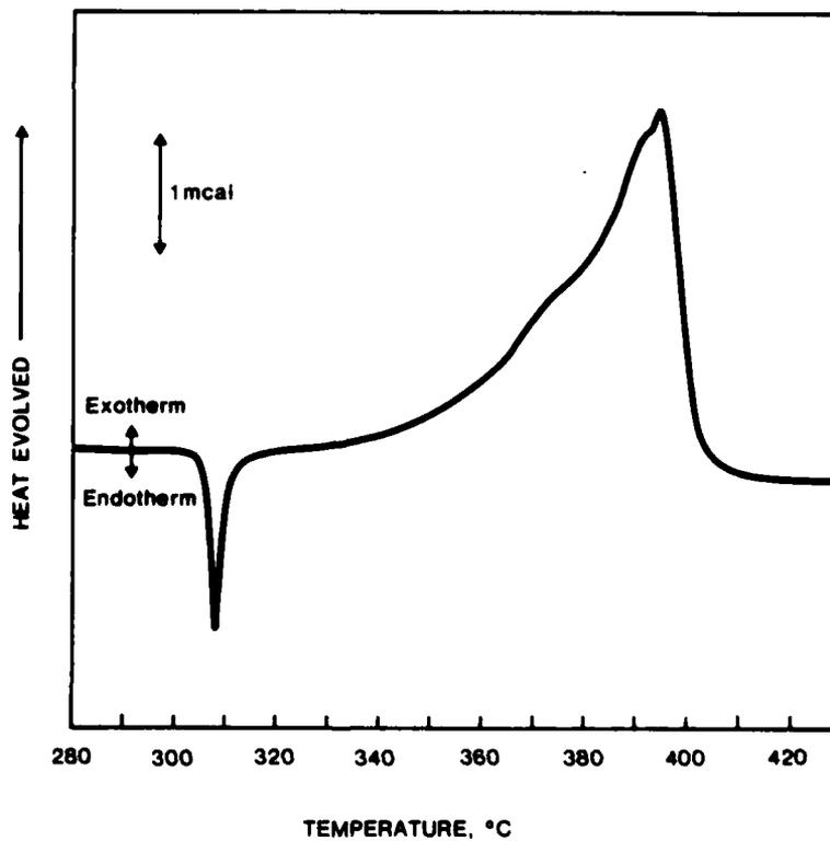
Fig. 2 DSC Thermogram for Silver Azide, heating rate 40°C/min, 0.35 mg.
