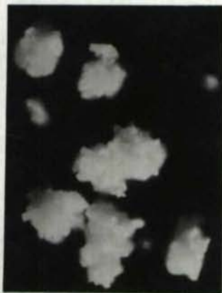
Fig 45 X50 Lead azide - P.E.T.N. Composite granule
