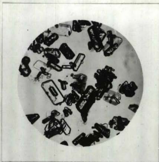
Fig1. X50 Barium styphnate from barium acetate and styphnic acid
