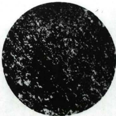
Fig. 25 X50 Lead azide precipitated in the presence of sulphate type of surface active agent.
