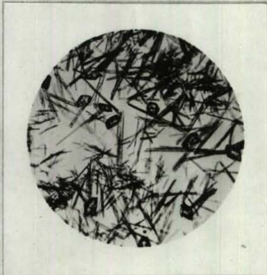
Fig6. X50 Barium styphnate trihydrate (accicular) being converted to fig.5 product (monohydrate).
