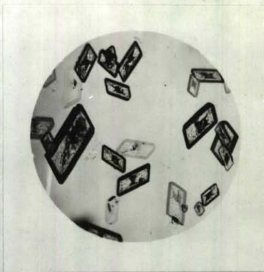
Fig.2. X50 Barium styphnate from barium chloride added to magnesium styphnate.
