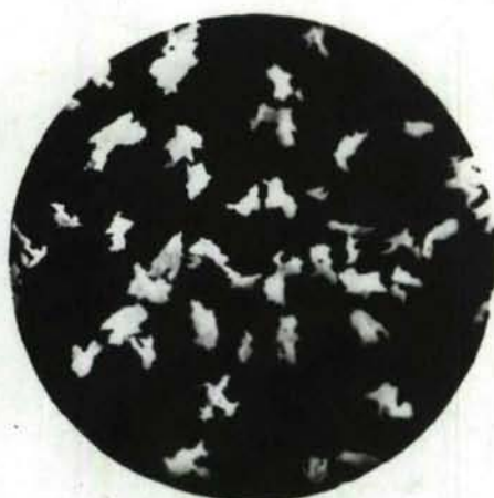
Fig 32 X50 Lead azide co-precipitated with sodium carboxy methyl cellulose (RD1333)
