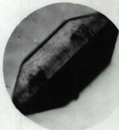
Fig. 26 X500 Lead azide, service, showing nucleating growths of lead carbonate
