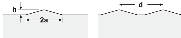
Fig. 8.43. A ridge formed on the surface of a strained elastic material under plane strain conditions is shown on the left. The diagram on the right shows a pair of identical ridges with their centers separated by a distance d .
