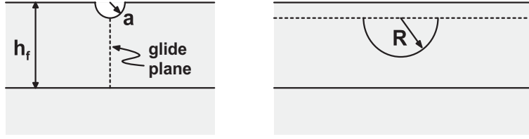
Fig. 6.41. Schematic diagram of dislocation nucleation from the base of a cylindrical groove in the surface of a strained film. The radius of the groove of semicircular cross-section is a and the radius of the semicircular dislocation line is R .
