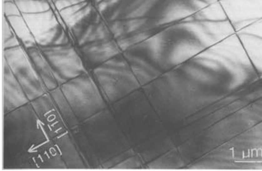
Fig. 1.16. A plan-view, bright-field transmission the electron microscopy (TEM) image of misfit dislocations within the interface between a 200-nm thick \text{Si}_{0.9}\text{Ge}_{0.1} film and a much thicker (001) Si substrate. The dislocations form a crossed-grid pattern which is oriented along two \langle 110 \rangle directions on the (001) interface plane. Reproduced with permission from Fukuda et al. (1988).
