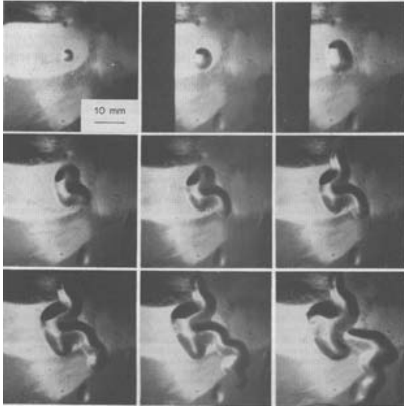
Fig. 5.18. Optical micrographs showing axisymmetric growth followed by telephone cord instability in response to an increase in mismatch stress in a mica film bonded to an aluminum substrate. Reproduced with permission from Hutchinson et al. (1992).
