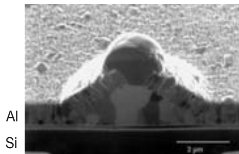
Fig. 7.25. Cross-sectional focused ion beam image of a hillock penetrating through the surface of a 1\text{ }\mu\text{m} thick Al film on a relatively thick (100) Si substrate. Reproduced with permission from Kim et al. (2000).
