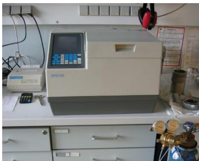
Figure 1.20 Parr 1356 bomb calorimeter equipped with a Parr 1108CL oxygen bomb.
