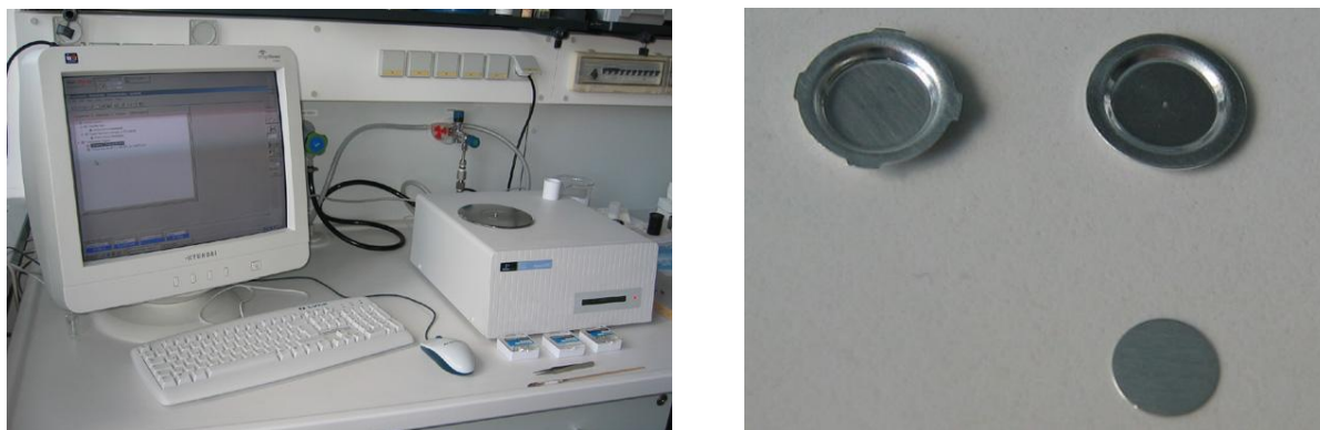
Figure 1.19 left: Perkin Elmer Pyris 6 DSC; right: DSC Aluminum sample container
