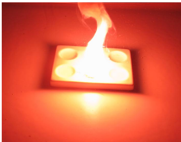
Figure 11.16 Combustion of a mixture containing magnesia and strontium tetrazolate pentahydrate (1:1).
