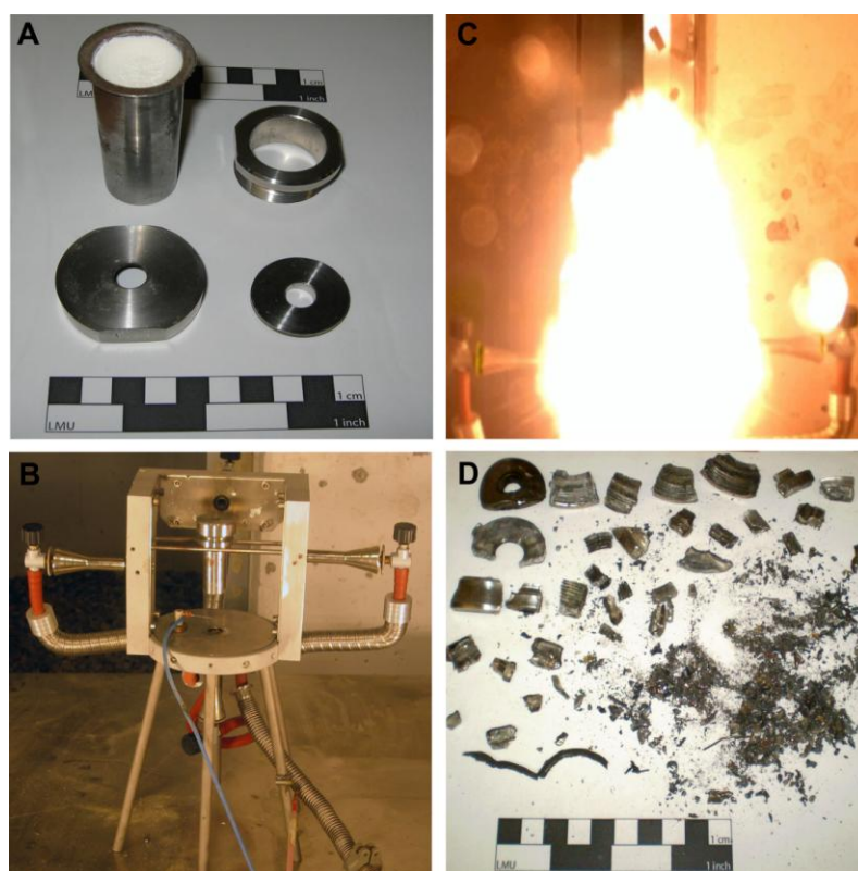
Figure 3.31 A) Steel Sleeve loaded with 25 mL explosive; B) Koenen test setup showing the four Bunsen burners; C) Moment of explosion (0.25 ms) of HATDN; D) Collected fragments.
