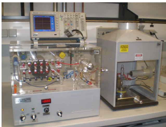
Figure 1.25 OZM small scale electrical discharge device
