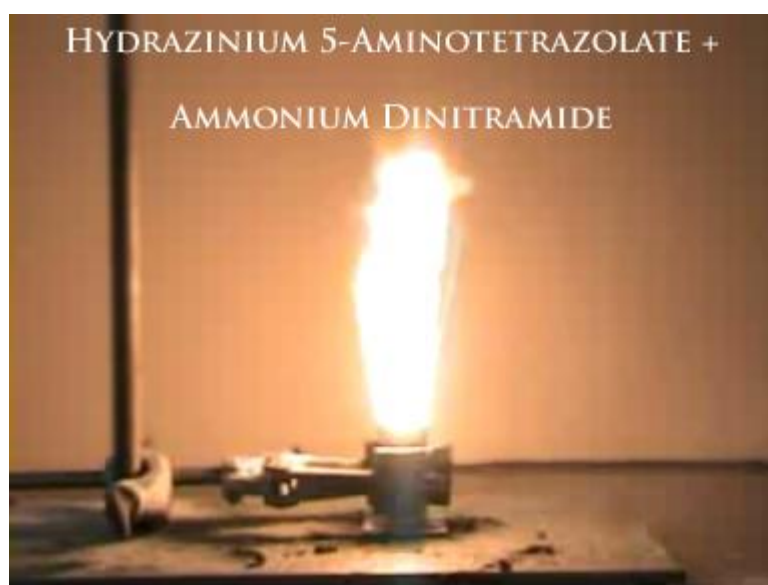
Figure 2.13 Combustion of 60:40 mixture of 30 with ADN.
