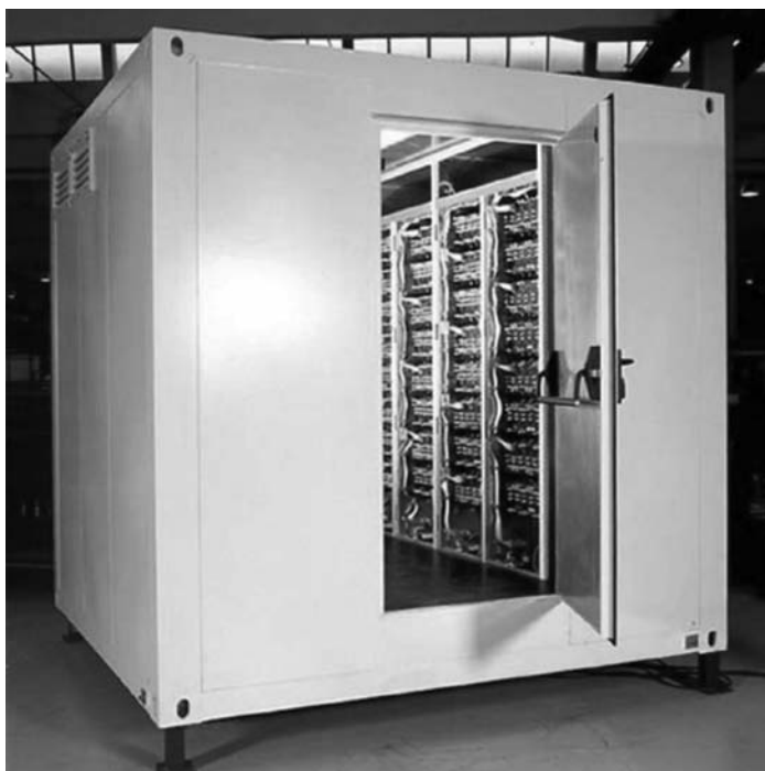
FIGURE 11.21 Siemens "SITRAS SES" energy storage system for railway applications. The module consists of 1344 DLC pieces of 2600F.
