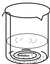
Figure 5.1 Suspension of aluminum wire in \text{CuCl}_2 solution.
