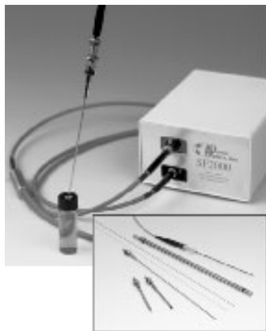
Figure 19-19 Fiber-optic sensor measures O_2 by its ability to quench the luminescence of Ru(II) at the tip of the fiber. A blue-light-emitting diode provides excitation energy. [Courtesy Ocean Optics, Dunedin, FL]
