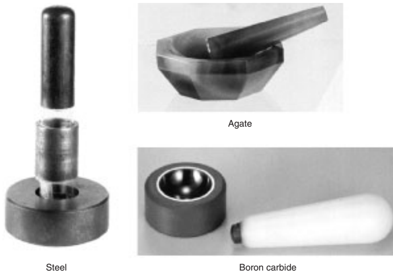
Figure 28-5 Steel, agate, and boron carbide mortars and pestles. The mortar is the base and the pestle is the grinding tool. In regard to boron carbide, the mortar is a hemispheric shell enclosed in a plastic or aluminum body. The pestle has a boron carbide button at the tip of a plastic handle. [Courtesy Thomas Scientific, Swedesboro, NJ, and Spex Industries, Edison, NJ.]
