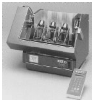
Figure 28-9 Automated apparatus that fuses three samples at once over propane burners. It also provides mechanical agitation of the Pt/Au crucibles. Crucibles are shown in the tipped position used to pour contents out after fusion is complete. [Courtesy Spex Industries, Edison, NJ.]
