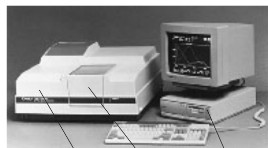
(a) Source, monochromator, detector Sample compartment Display and controls
