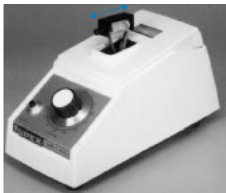
Figure 28-6 Wig-L-Bug sample shaker and polystyrene vial and ball for pulverizing soft materials. The arrow shows the direction of shaking. [Courtesy Spex Industries, Edison, NJ.]
