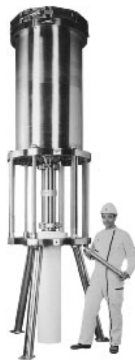
Figure 23-8 Industrial-scale preparative chromatography column can purify a kilogram of material. The column volume is 300 L. [Courtesy Prochrom, Inc., Indianapolis, IN.]
