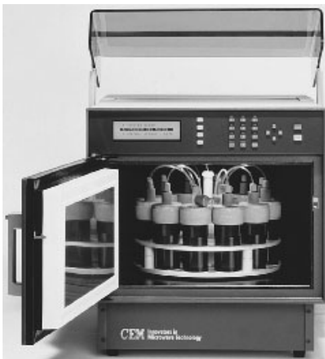
Figure 28-13 Extraction vessels in a microwave oven that processes up to 12 samples in under 30 min. Each 100-mL vessel has a vent tube that releases vapor if the pressure exceeds 14 bar. Vapors from the chamber are ultimately vented to a fume hood. The temperature inside each vessel can be monitored and used to control the microwave power. [Courtesy CEM Corp., Matthews, NC.]
