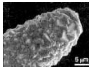
Boron-doped diamond coating on Pt electrode.
