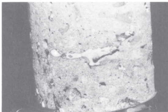
Figure 10.34 Exuded gel on the surface of a core.
