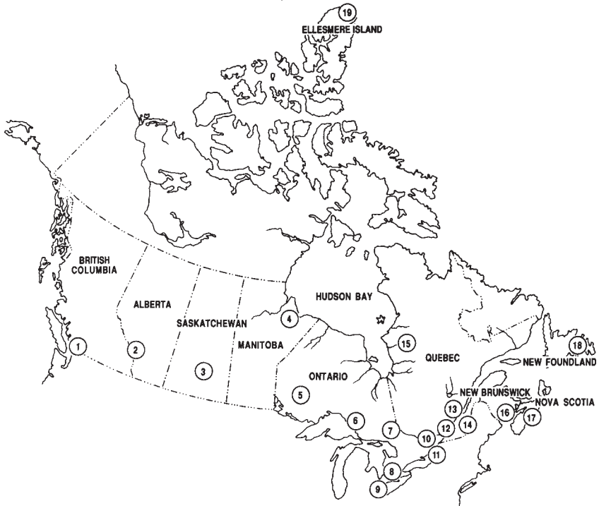
Figure 8.2 Map of Canada showing locations of sources of documented reactive aggregates. 1, Chilliwack, BC , acid volcanic rock in gravel deposits; 2, Near Calgary, Alberta , metaquartzite rock and chert; 3, South Saskatchewan River, Saskatchewan , opaline shale; 4, Nelson River, Manitoba , dolomitic limestone (alkali-carbonate reaction); 5, Sioux Lookout, north-western Ontario , chert in gravels; 6, Wawa, Ontario , silicified volcanic glass and tuff from gravel; 7, Sudbury area of Ontario , argillite, greywacke, quartz arenite and quartz sandstone from gravel deposits; 8, south-western Ontario , potentially reactive cherts; 9, Windsor, Ontario , chert in fine gravel; 10, Ottawa area, Ontario , silicious limestone; 11, Kingston and Cornwall, Ontario , alkali-carbonate reaction; 12, Montreal area, Quebec , sandstone and silicious limestone; 13, Quebec City, Quebec , silicious limestone; 14, Beauceville region, Quebec , andesitic tuff; 15, James Bay region of Quebec , biotite gneiss; 16, southern New Brunswick , gravel deposits containing quartz arenites, argillites, greywackes and volcanic rocks; 17, Nova Scotia , quartzites, greywackes, phyllites quartz arenites, argillites and rhyolite from several areas; 18, eastern Newfoundland , silicified volcanic rock in gravel deposits; 19, Alert, Ellesmere Island , greywacke and chert (silicified volcanics).
