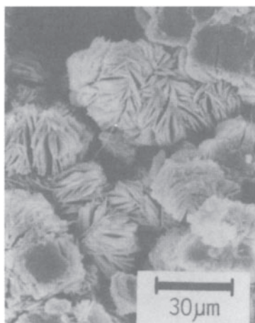
Figure 10.5 Scanning electron micrograph of rosette-like products. From Ref. 10.
