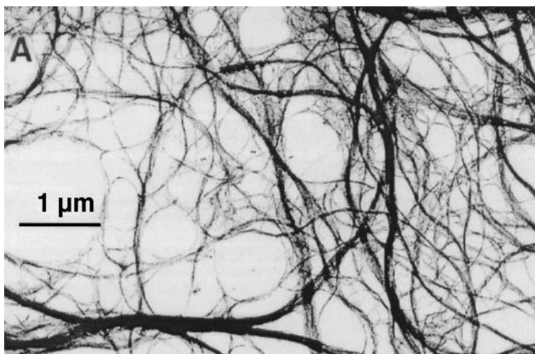
Figure 3.3 Transmission electron micrograph of a dilute suspension of sugar beet cellulose. (From Reference 20 with permission from Springer.)
