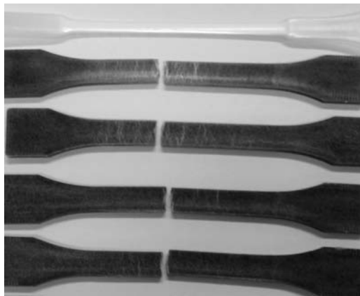
Figure 7.5 Jute/PP tensile samples with 0, 6, 12, 18, and 23 vol% jute from Cabral et al. (unpublished results). (Fiber content increases from the top to the bottom.)
