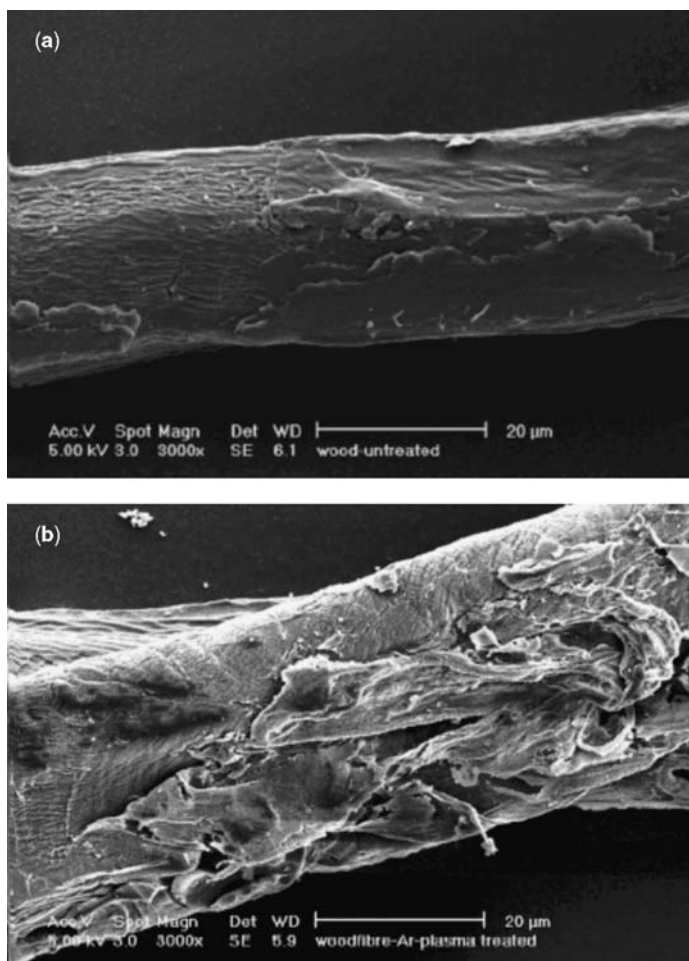
Figure 3.4 (a) SEM of the untreated wood fiber surface. (From Reference 35 with permission from Elsevier Ltd.) (b) SEM of the argon plasma treated wood fiber surface. (From Reference 35 with permission from Elsevier Ltd.)
