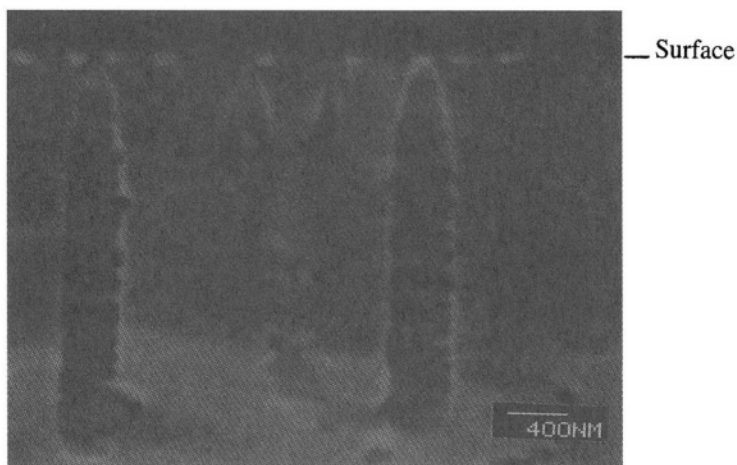
FIGURE 8.37. Variation of diameter of pores from the surface to the bulk, where it is constant, in 1% HF, 6 V, n(100) , 10^{17}/\text{cm}^3 . After Zhang. 8 (Reproduced by permission of The Electrochemical Society, Inc.)
