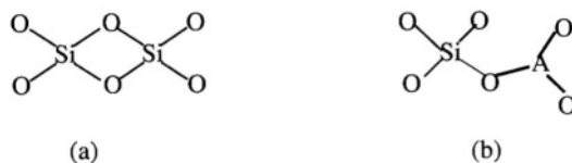
FIGURE 4.41. Disruption of silicon oxide structure due to the presence of an impurity element. (a) Structure without impurity; (b) structure with impurity.
