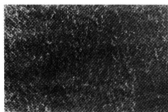
(a) p-Si, 25 \Omega cm, 40% HF, 30 mA/cm 2
