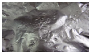
Abrasion and holes created by ultrasound on aluminum foil
