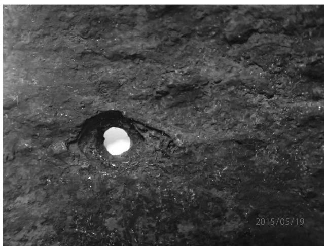
FIGURE 12.1 Photo of interior pipe failure joint at 580 meters.
