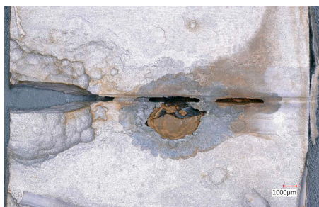
FIGURE 19.3 Example of damage on longitudinal weld of the pipe.
