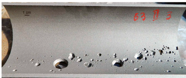
FIGURE 15.4 Perforation, deep pitting without thinning on bottom section (5 to 7 o'clock) observed on sweep-blasted section of FL-1 sample 2.
