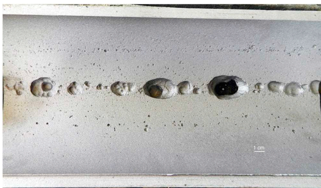
FIGURE 15.9 Pitting and channels between two perforations along the bottom of FL-4 sample 1.
