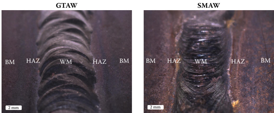
FIGURE 13.1 Joints welded by gas tungsten arc (GTAW) and shielded metal arc (SMAW) before biocorrosion experiments. BM, base metal; HAZ, heat-affected zone; WM, weld metal.
