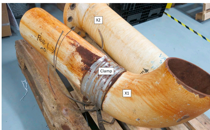
FIGURE 7.3 Pipe samples denoted X1 and X2, respectively. Note that the leak point on X1 is wrap repaired by a glued rubber plate fixed to the pipe using metallic strips. X1: Spool section with reported pinhole leakage. X2: Spool section from 2.5 m downstream the leakage location, including flange.
