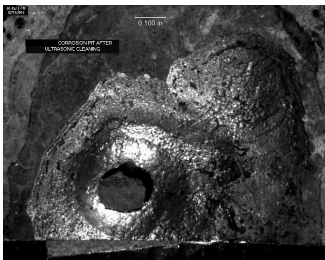
FIGURE 16.5 Micro photo of interior pipe hole after ultrasonic cleaning
