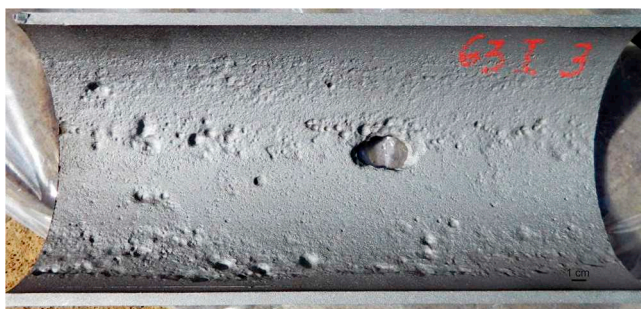
FIGURE 15.3 Perforation at 6 o'clock, deep pitting with thinning on bottom section (5 to 7 o'clock) observed on sweep blasted section of FL-1 sample 1.
