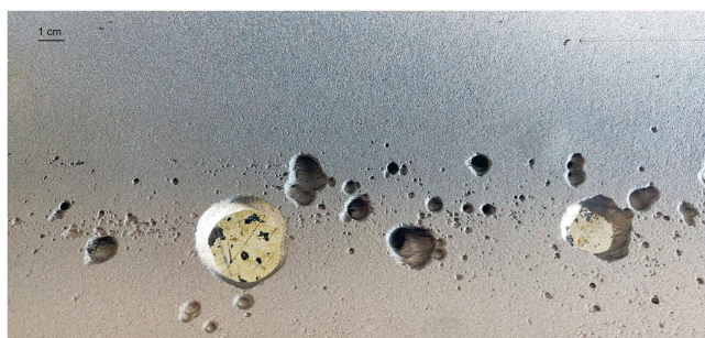
FIGURE 15.6 Close-up photograph showing perforation on FL-1 sample 2. Perforation pit boundary is sharp and not surrounded by pits.
