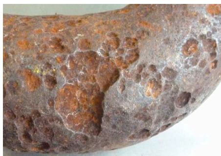
FIGURE 17.1 Part of corroded steel chain link (76 mm diam.) showing evidence of highly localized corrosion after removal of rust layers.
