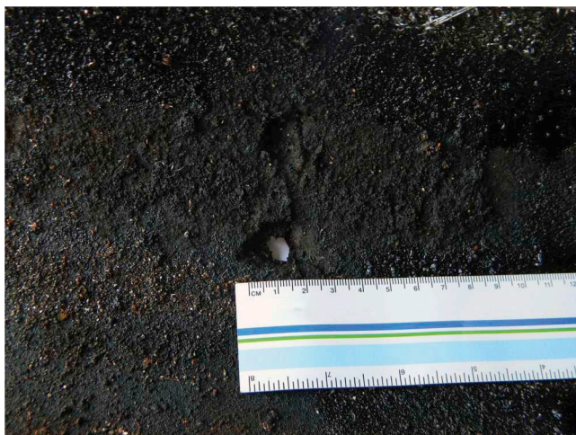
FIGURE 15.7 Blackish deposit near and away from the perforation (5 to 7 o'clock) observed on FL-4 sample 1 section taken from underground portion of the flowline.
