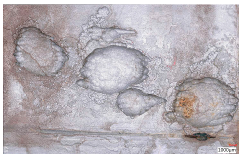
FIGURE 19.5 Example of pitting damage on pipe 2. Left: Multiple pits with max. pit depth of 2.2 mm (bottom right in this picture). Right: Detail of cross cut at perforation at the junction point.
