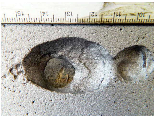
FIGURE 15.11 Typical association of a large pit with a small pit on FL-4 sample 2.
