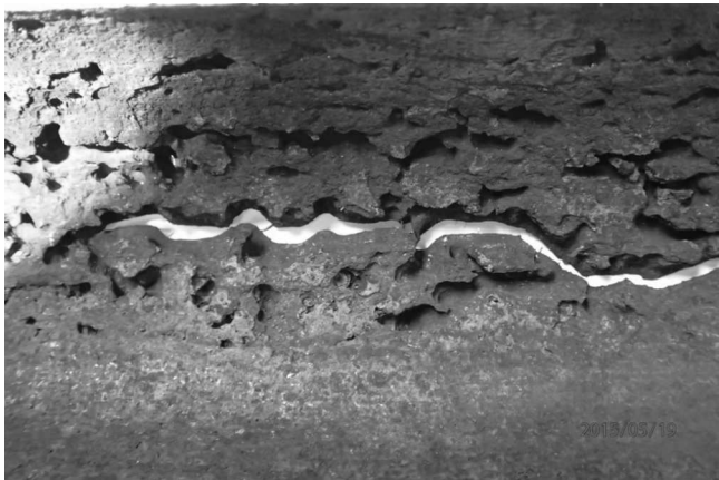
FIGURE 12.3 Photo of inner diameter pipe failure sample burst point.
