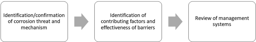
FIGURE 20.1 Three-step methodology for root cause analysis of a failure.
