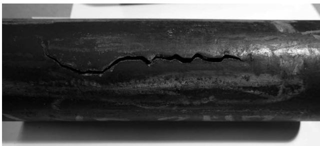
FIGURE 12.2 Photo of outer diameter pipe failure sample burst point.
