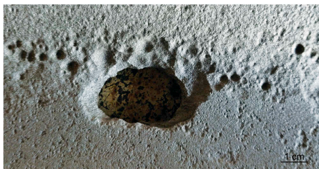
FIGURE 15.5 Close-up photograph showing several deep pits surrounding perforation on FL-1 sample 1. Pit boundary diffused and sloped.
