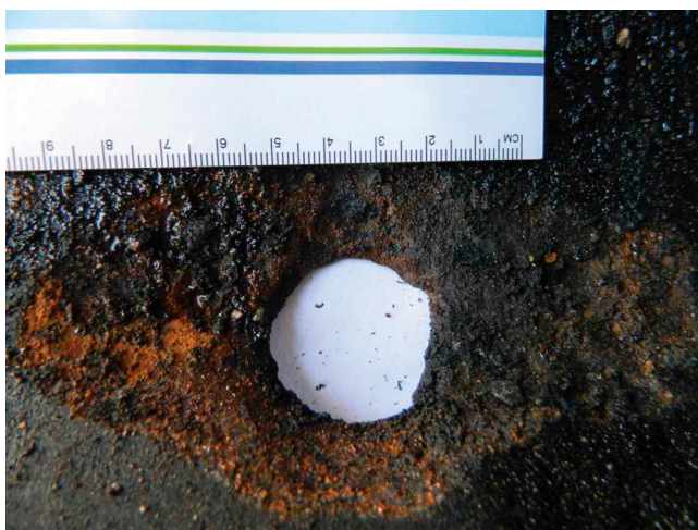
FIGURE 15.8 Blackish and orange-brown deposit near the perforation (5 to 7 o'clock) observed on FL-4 sample 2 section taken from aboveground portion of the flowline.
