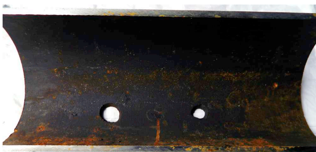
FIGURE 15.2 Thin, black deposit near perforation and away from perforation (5 to 7 o'clock) observed on FL-1 sample 2. No SRB were detected in this deposit.
