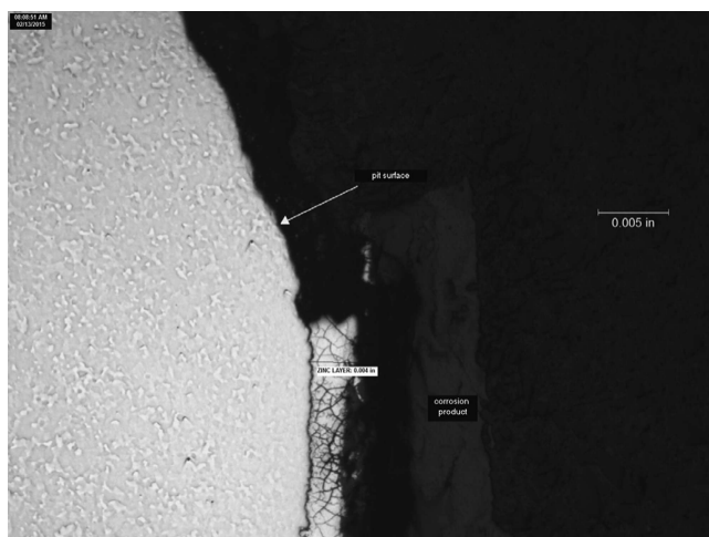
FIGURE 16.8 Cross section of pipe pit surface.
