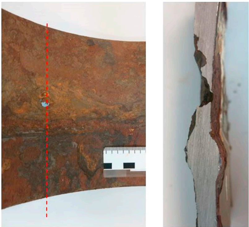
FIGURE 7.15 Metallographic sample (cross section) cut out for micro examinations (X1 through leak site).
