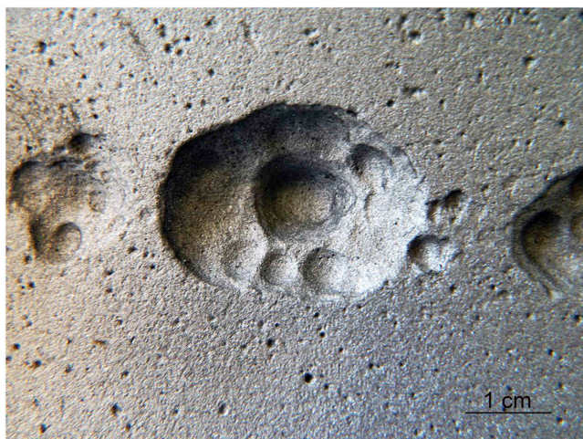
FIGURE 15.10 Pits within pits arrangement (5 to 7 o'clock) on FL-4 sample 2. Diffused boundary between large and small circular pits with sloped edges can be seen.
