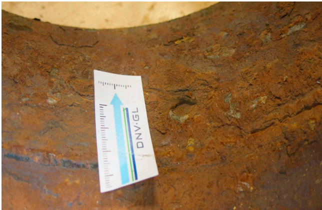
FIGURE 7.9 Close-up photo of a local corrosion cavity approximately 20 mm from the weld root as also shown in Figure 7.8.
