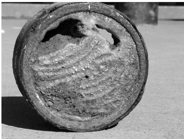
FIGURE 3.2 A pipe cross section showing the accumulation of salt layers that occurred over years of service in a natural gas pipeline that experienced occasional upsets of high salinity brine.
