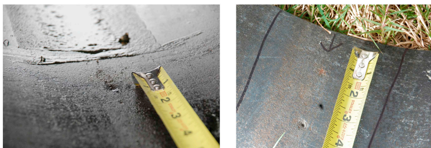
FIGURE 10.1 Field photographs showing representative pits along the bottom of the pipeline, as-found (left) and after cleaning (right).
