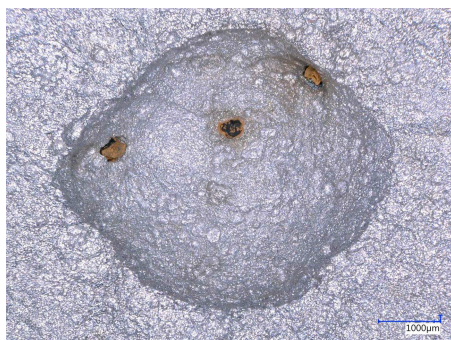
FIGURE 19.4 Severe corrosion pit in the wall of pipe 1. Pit depth is 1.5 mm.
