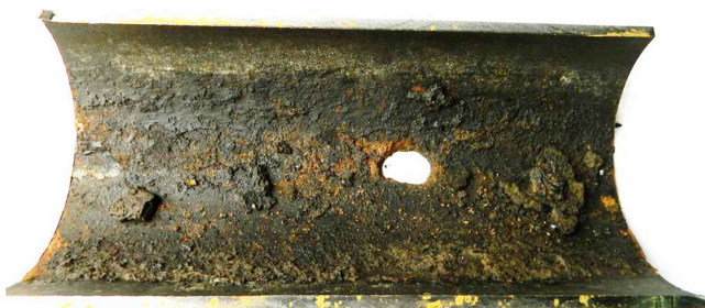
FIGURE 15.1 Brown-orange deposit near perforation and thick, black, loose deposits away from perforation (5 to 7 o'clock) observed on FL-1 sample 1. SRB were detected in this deposit.
