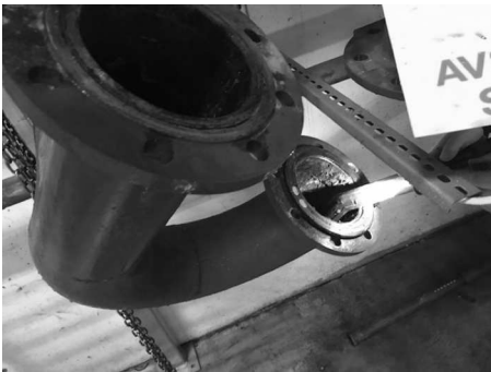
FIGURE 18.3 Inlet pipe in DN150 standard from the Women's and Children's Center. The pipe was a 1.5-meter U-bend and was replaced in 2017 due to corrosion. The pipe had been in operation for 10 years.
