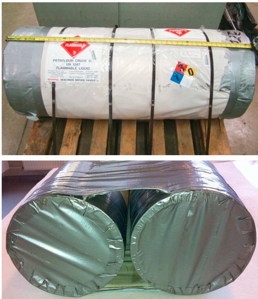
FIGURE 24.6 Examples of how the pipe sections are sealed (individually) with clean plastic and duct tape at the ends. Pipe sections should be placed on pallets and strapped firmly before shipment.
