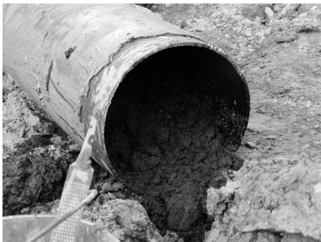
FIGURE 3.1 Thick sludge found when investigating internal corrosion in a pipeline.
