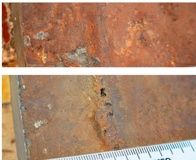
FIGURE 7.13 Representative internal surface along the weld. General corrosion and some corrosion pits along the weld.
