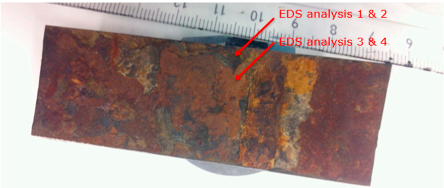
FIGURE 7.18 Section prepared for EDS analysis (in area indicated by arrows).
