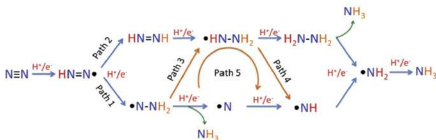
Fig. 13.10 Propose mechanism for the photocatalytic \text{N}_2 reduction [195]
